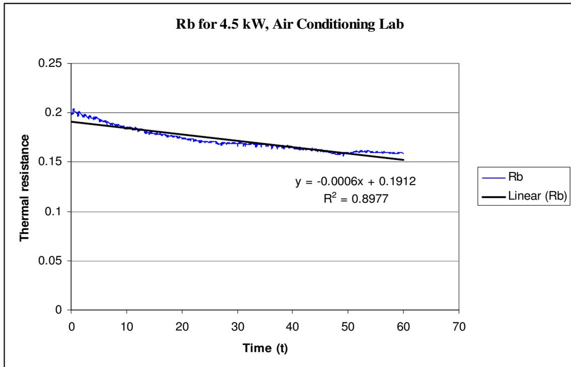
Figure 3 Thermal Resistances ( $R_b$ ) as a function of Time (t)
