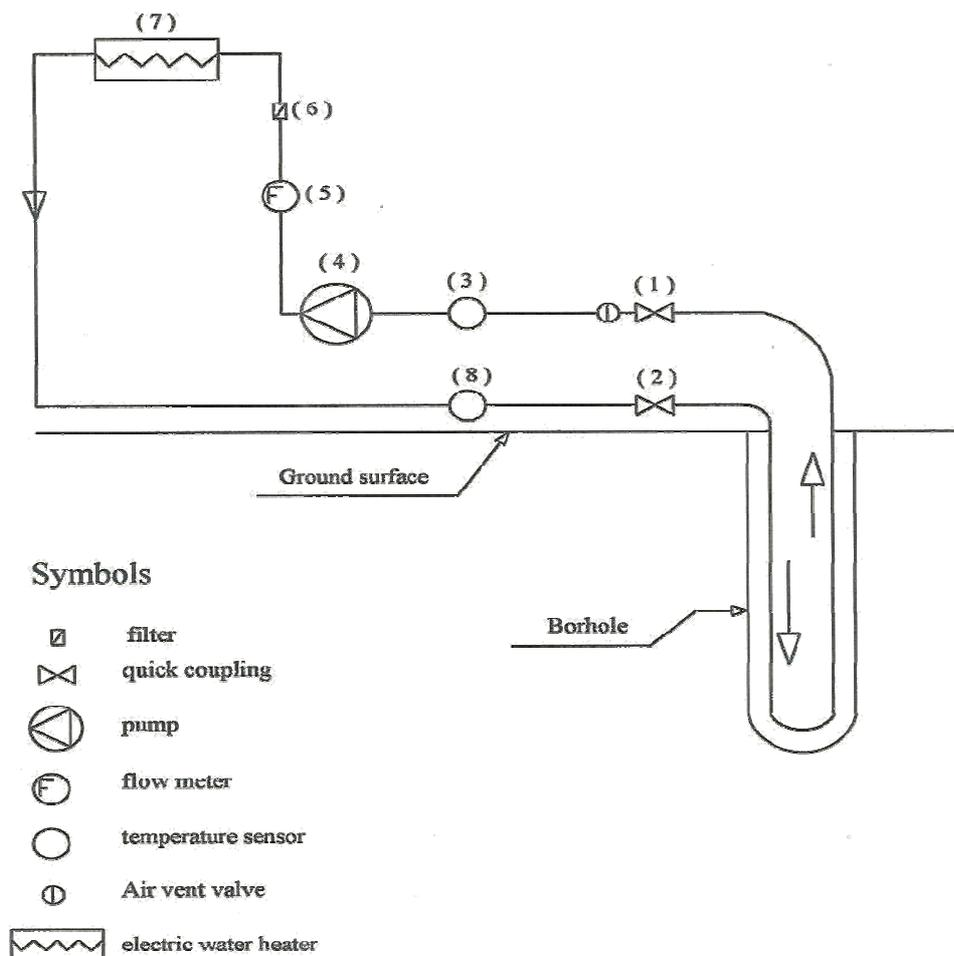
Figure 1 schematic a diagram of the experimental setup.
