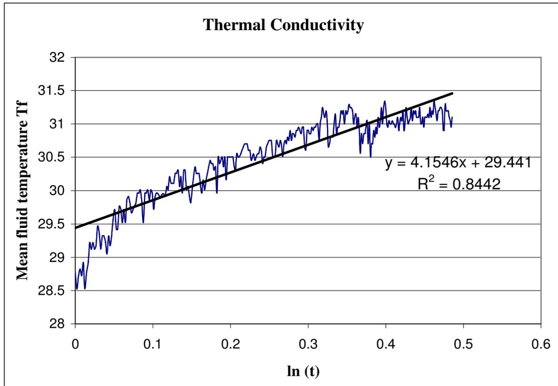
Figure 2 linearized function of the Mean Fluid Temperature ( $T_f$ ) versus Logarithmic time  $\ln(t)$
