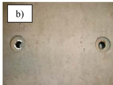
Steel tubes with one flange, illustrated in Fig. 4, with an inner diameter of 20mm and a length of 48mm set for screws were made for the DST+S series. Each screw was pre-tensioned with 130Nm using a torque wrench.
