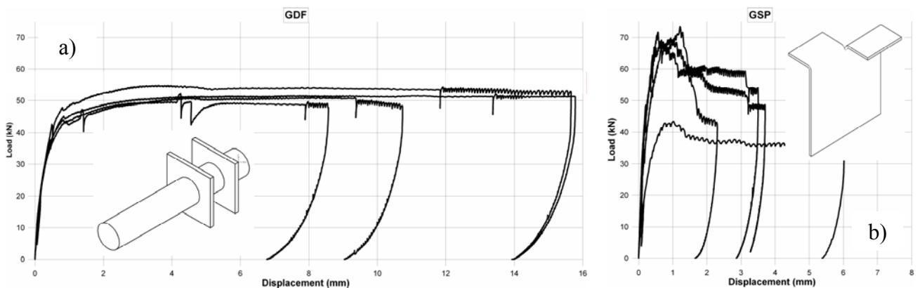
Fig. 11 Load-slip curves for shear connector types a) GDF and b) GSP
