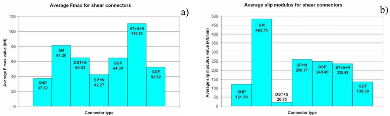
Fig. 8 Shear test results a) average failure load, b) average slip
