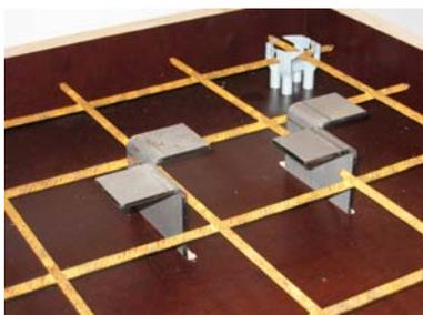
In Fig. 5 a pair of steel plates forms a shear connector system (GSP) which was nailed to the glulam beam by means of 8 nails  $\text{Ø}4.5 \times 75\text{mm}$ . A 10mm displacement between plates, was made to provide overlap of the fasteners. The flanges folded in the steel plate act as anchorage in concrete slab. The total length of the plate was 160mm and the width 75mm measured in the holes plane.
