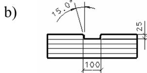
The notch in the glulam had a  $15^\circ$  slope and a width of 100mm measured at 25mm depth.
