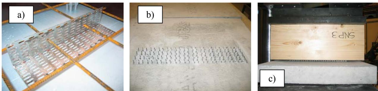
Fig. 2 Nailplate connector type a) in moulding form, b) prefabricated slab, c) pressing glulam member into concrete slab
