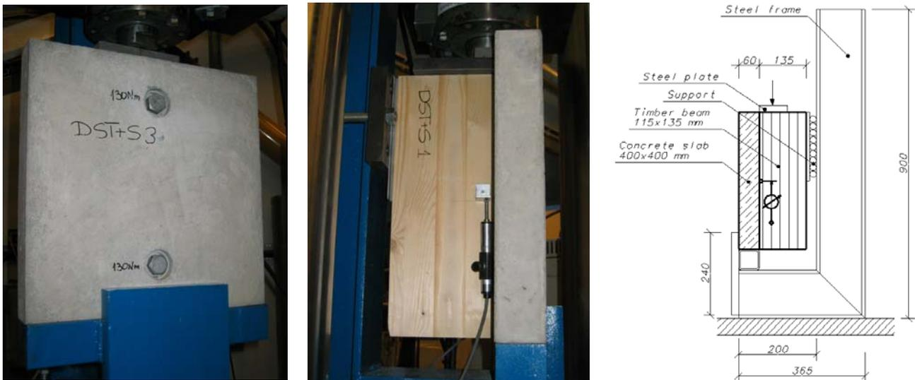
Fig. 1 Shear test set-up
