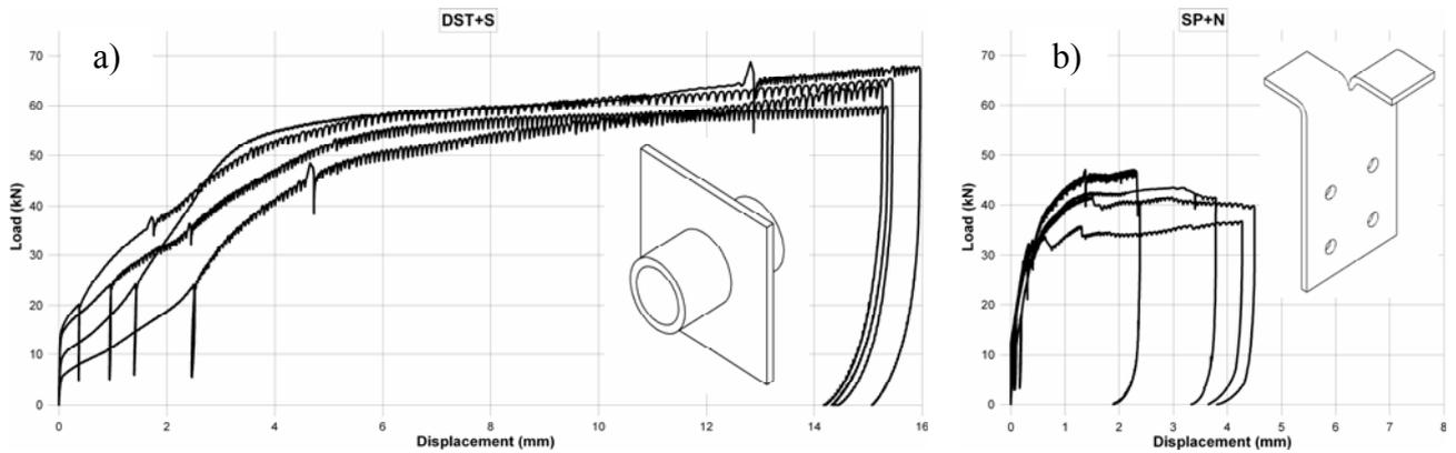
Fig. 9 Load-slip curves for shear connector types a) DST+S and b) SP+N.
