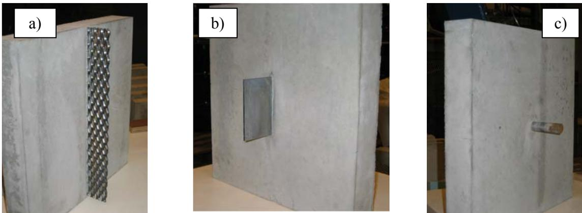
Fig. 3 Concrete slabs with inserted shear connectors a) SM steel mesh, b) GSP steel plate, c) GDF steel dowel
