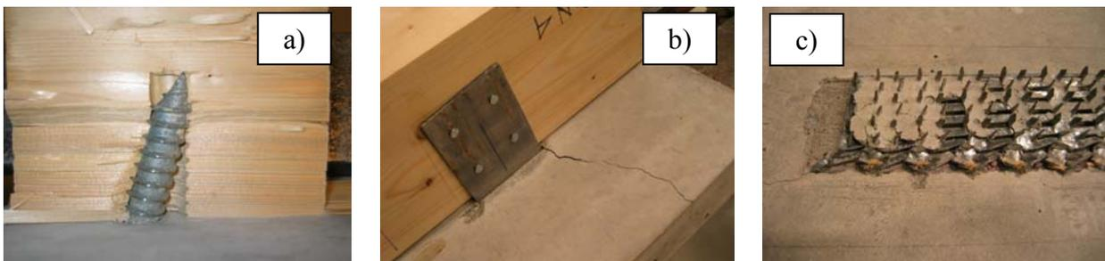
Fig. 10 Failure in connector types a) DST+S, b) SP+N, c) SNP,
