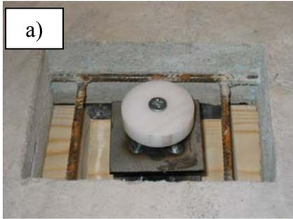
A steel tube shown in Fig. 6a), with a length of 67mm, with two welded flanges, together with a screw  $\text{Ø}20 \times 160\text{mm}$  placed above a notch in the timber beam is the ST+S+N series. A prefabricated concrete slab with a rectangular hole  $115 \times 120\text{mm}^2$  was placed on top of the glulam member. The hole was filled with concrete mix and tests were performed after 28 days from the filling operation. The screw was pre-tensioned with 130Nm using a torque wrench.
