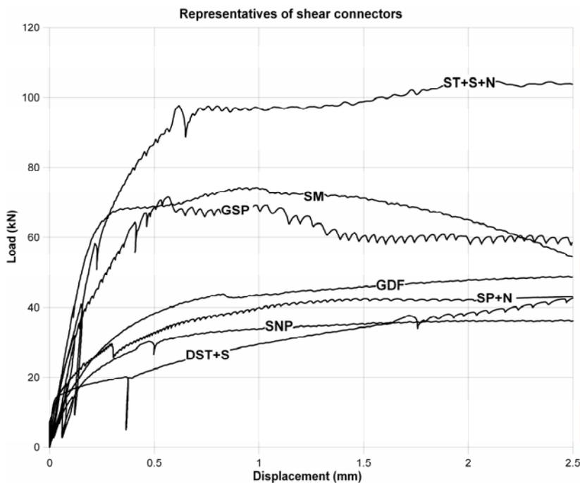
Fig. 7 Shear test results, load-slip curves representatives of all test specimens
