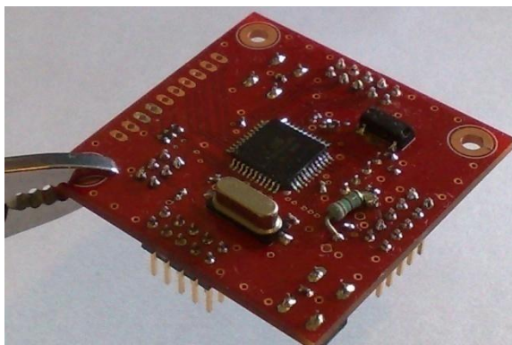
Fig. 16. Expansion Board with the ATmega 164P.
