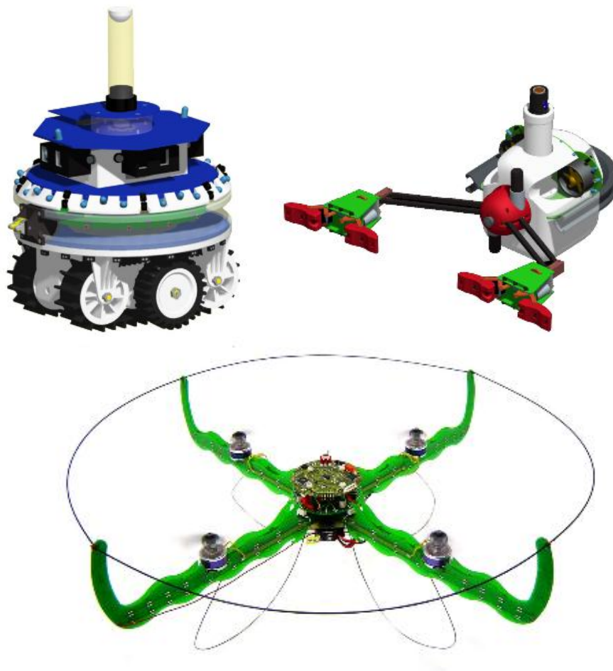
Fig. 12. A Foot-bot (Upper Left), a Hand-bot (Upper Right) and an Eye-bot (Lower Center), the three basic units that could comprise a Swarmanoid.
