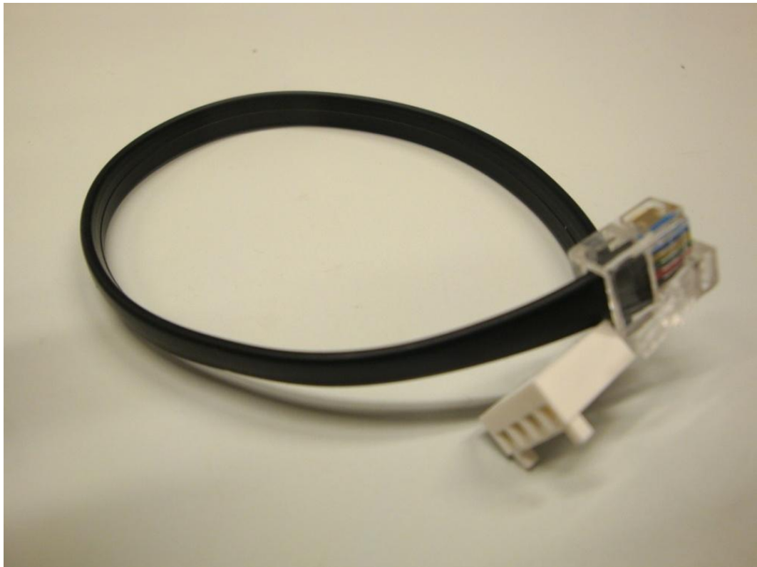
Fig. 18. NXT Module – Expansion board cable adapted to fit a regular header connector.
