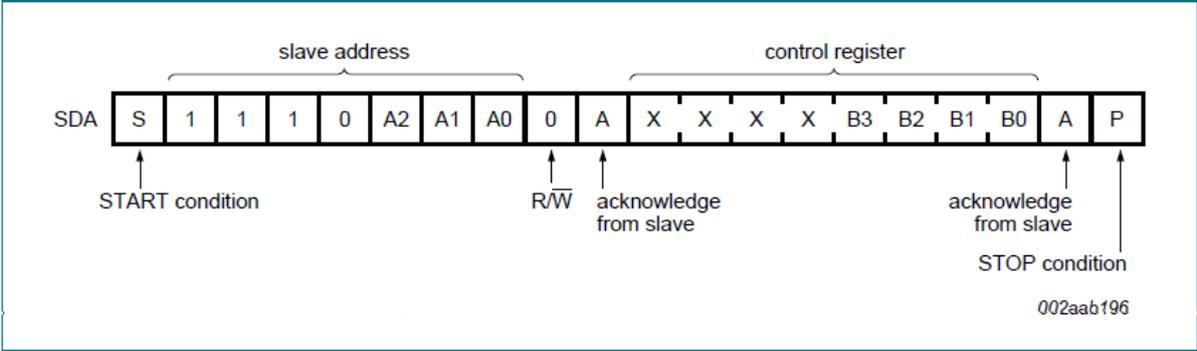
Figure 37: Write operation in PCA 9546A Control Register.
