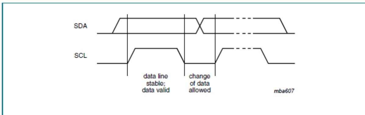
Figure26: Bit Transfer in I2C Bus.
