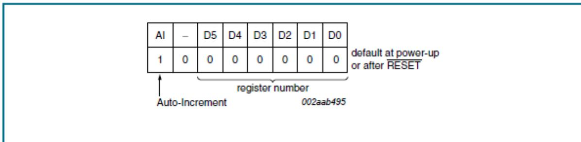
Figure 22: Data Byte stored in Command Register.
