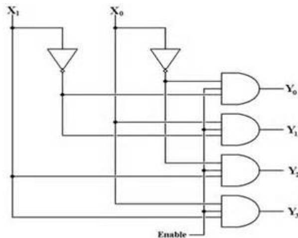
Figure 19: A 2-to-4 DEMUX circuit.
