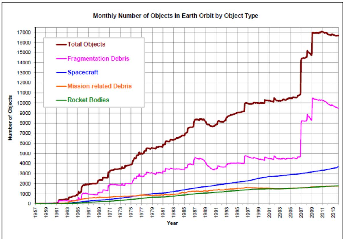
Figure 9: this chart shows the latest official summary of Debris in Earth orbit, cataloged by SSN. [13]
