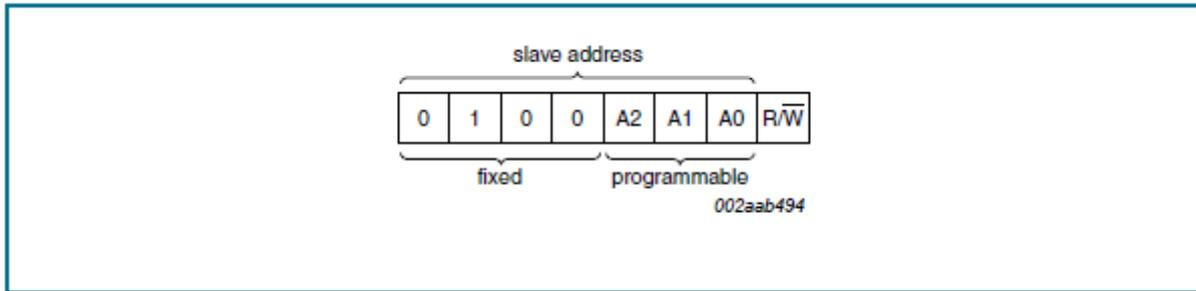
Figure 21: Data Byte for Device Address
