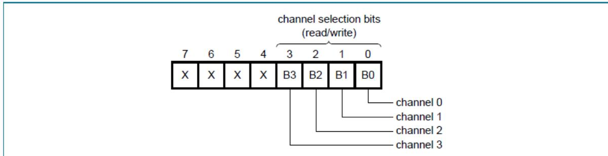
Figure 35: PCA 9546A channel selection.
