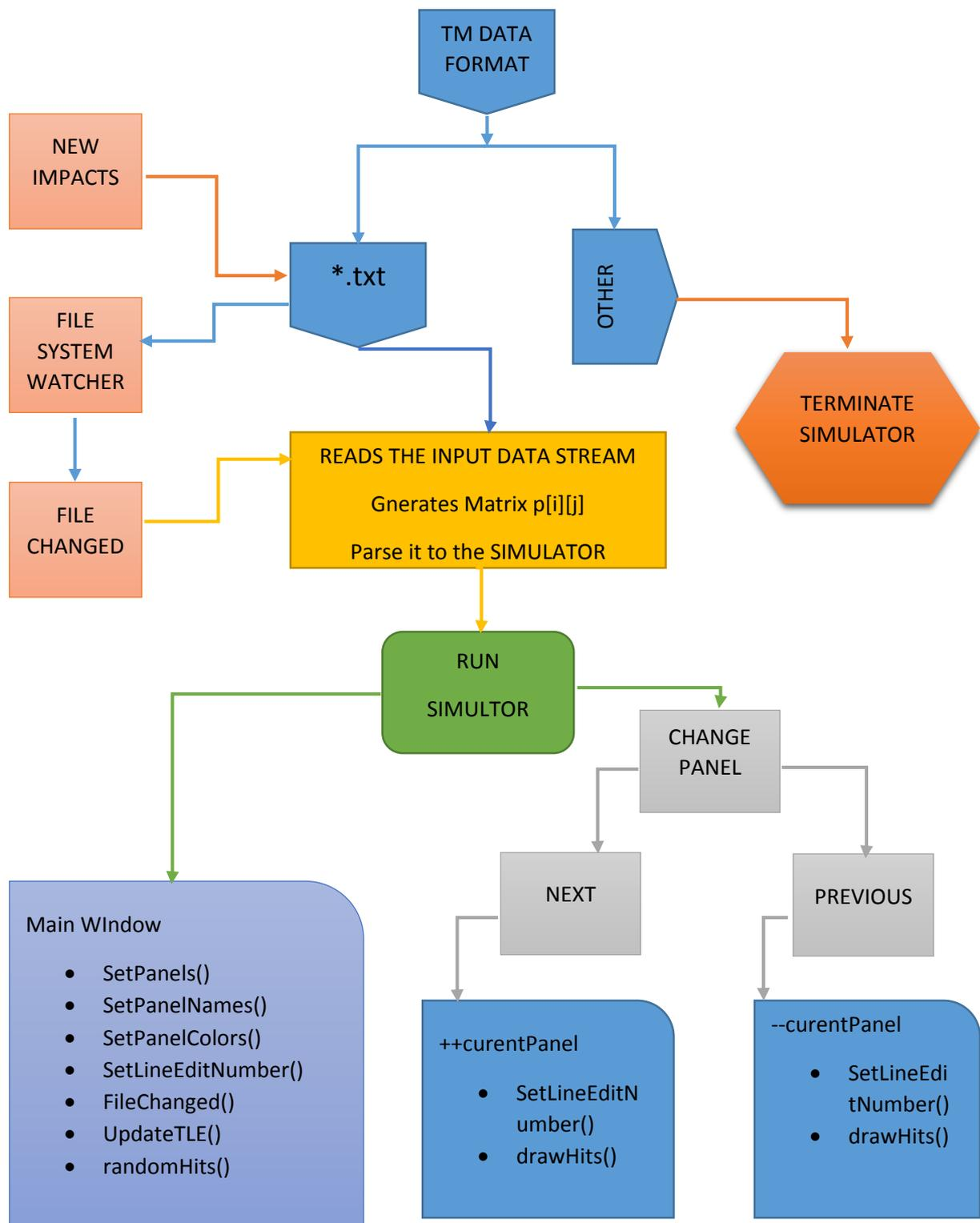
Figure 43: SOLID simulator Flow diagram.
