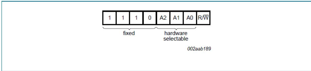
Figure 34: PCA 9546A Bus Address configuration.
