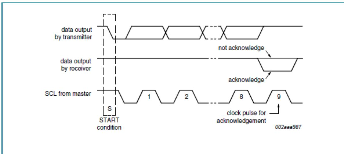
Figure 28: Acknowledgement on I2C Bus.
