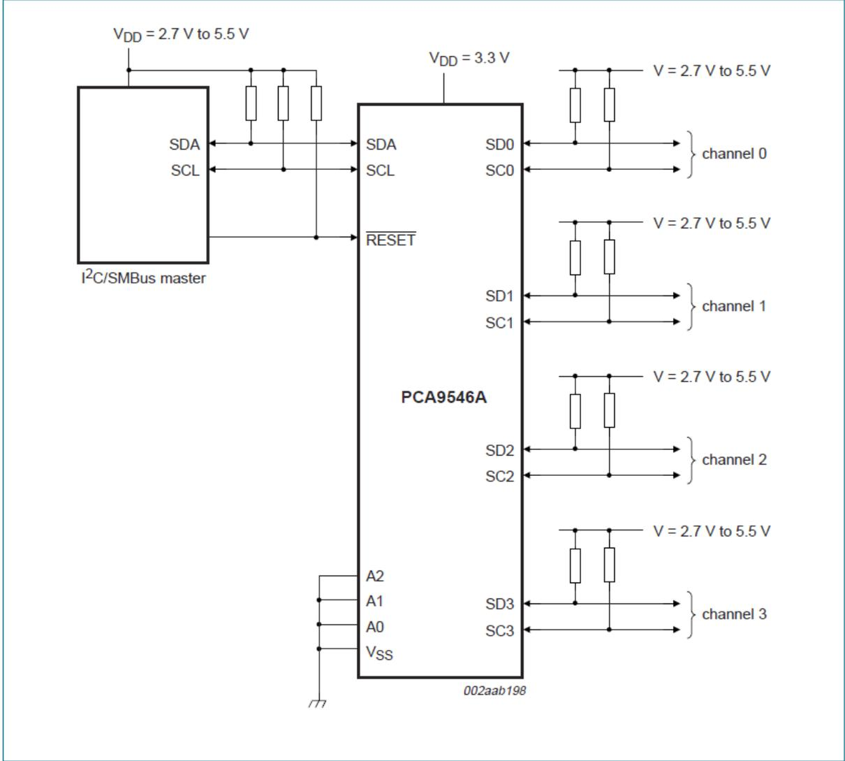
Figure 33: Application Diagram of PCA 9546A I2C Bus Switch.
