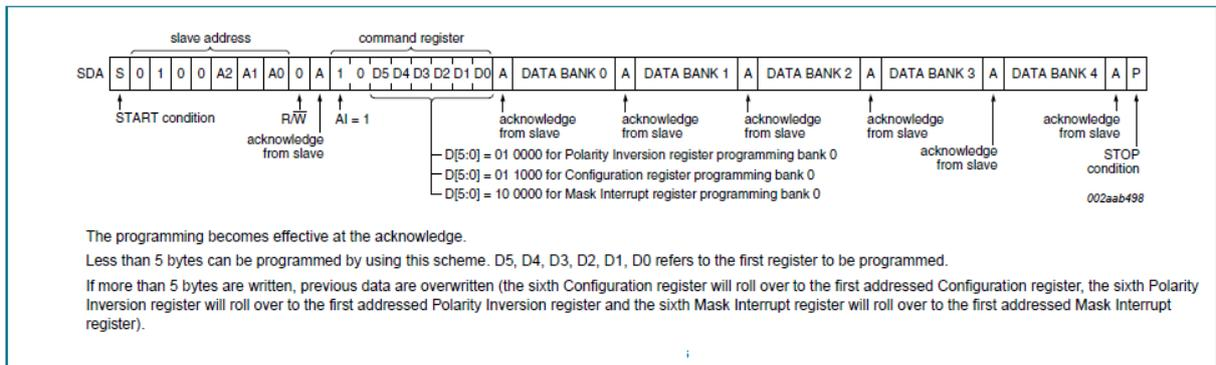
Figure 31: Write to the IOC or PI or MSK registers.
