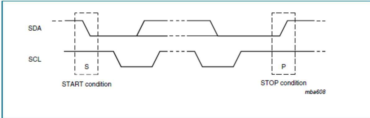
Figure 27: START and STOP condition.
