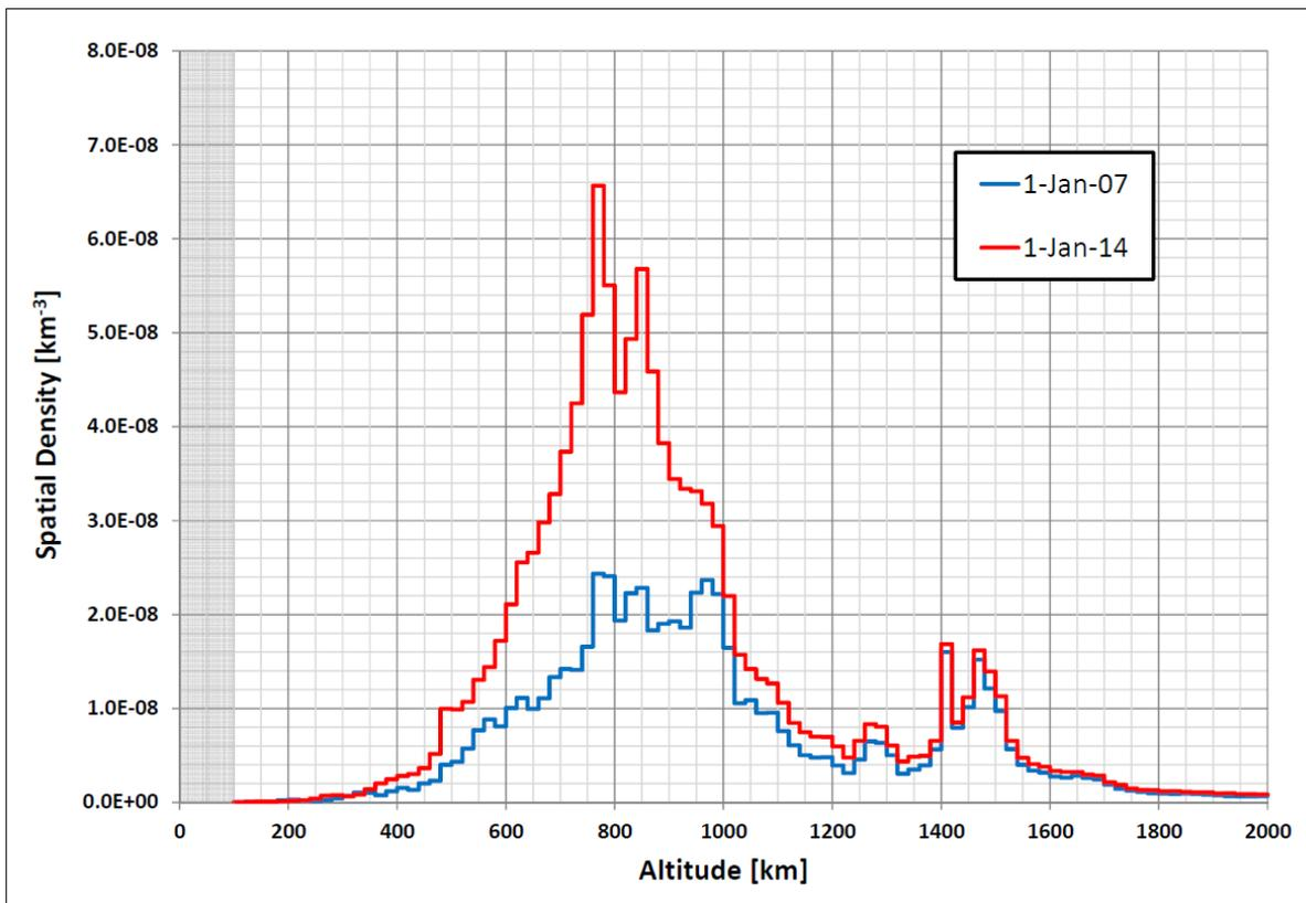
Figure 7: this chart compares the spatial density of Debris in LEO in year 2007 and 2014 [12]
