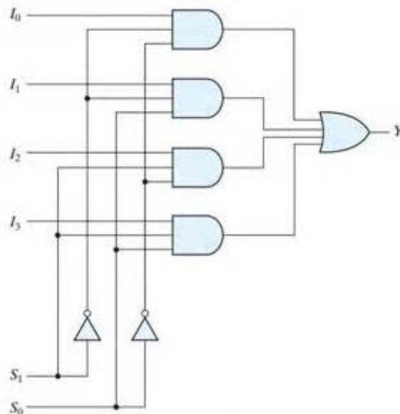
Figure 18: A 4-to-1 MUX construction with logic gates.
