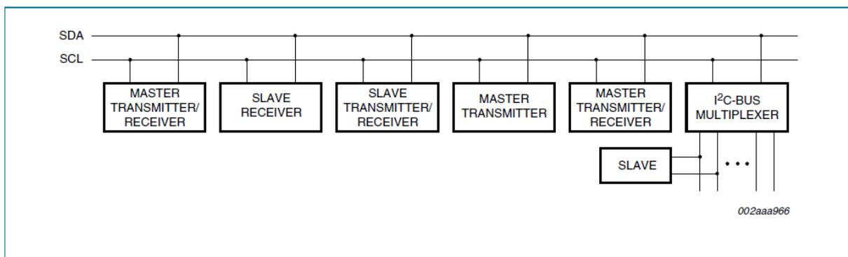
Figure 29: system configuration in I2C bus as Master and Slave.
