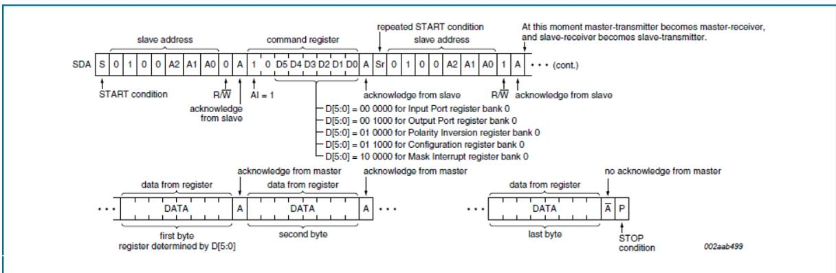
Figure 32: Read from IP, OP, IOC, PI and MSK registers.
