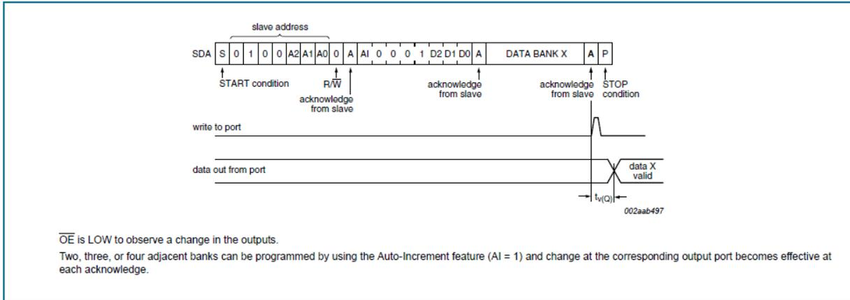
Figure 30: Write to a specific output port.
