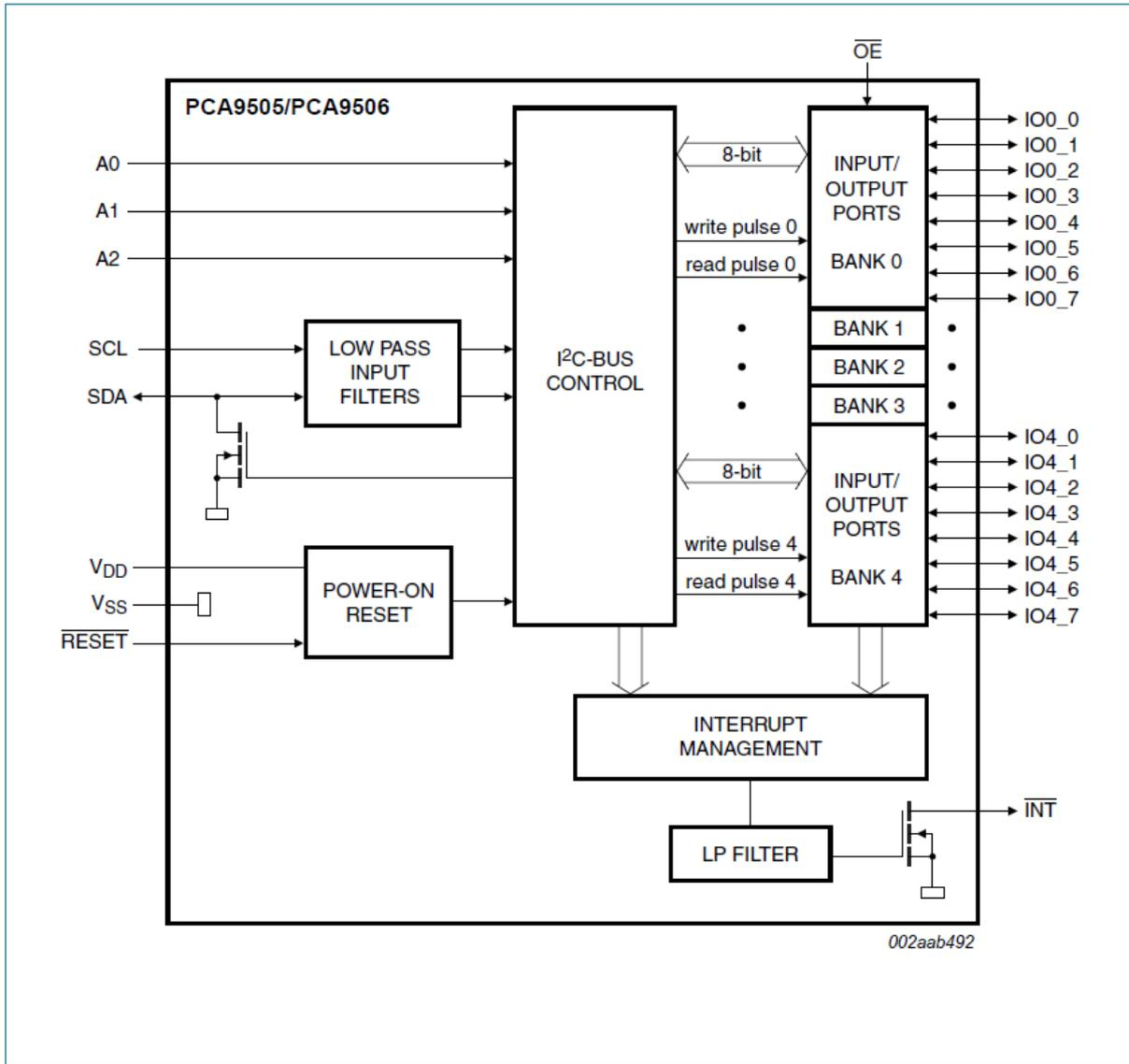
Figure 20: PCA 9505 /PCA 9506 Block Diagram.
