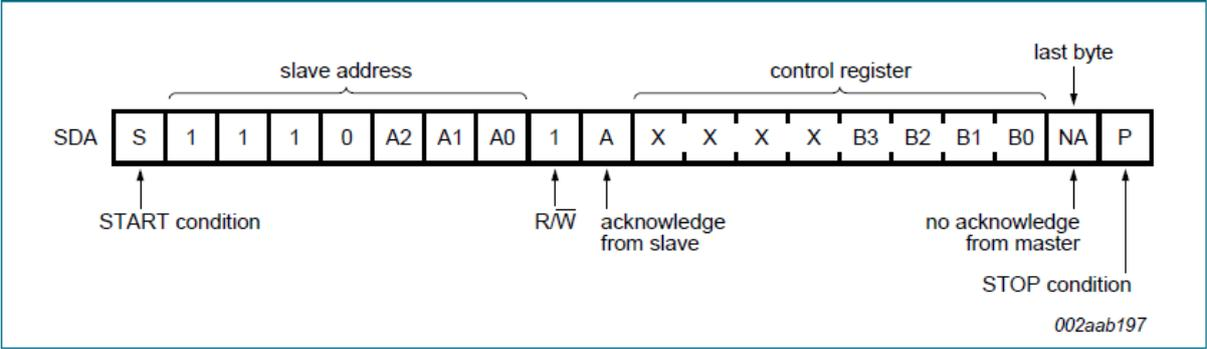
Figure 38: Read from PCA 9546A Control Register.
