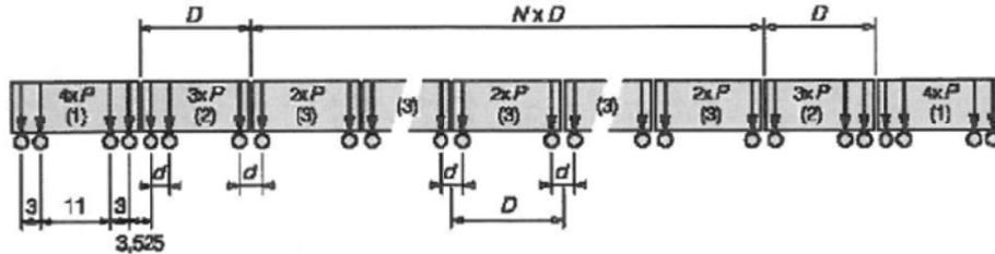
Figure (4.5) *Principal sketch of HSLM A1 from [10]. (1) Engine carriage, (2) coach connected to engine carriage, (3) intermediate carriage.*
