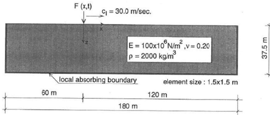
Figure (2.13) Schematic of load model, figure from [2].
