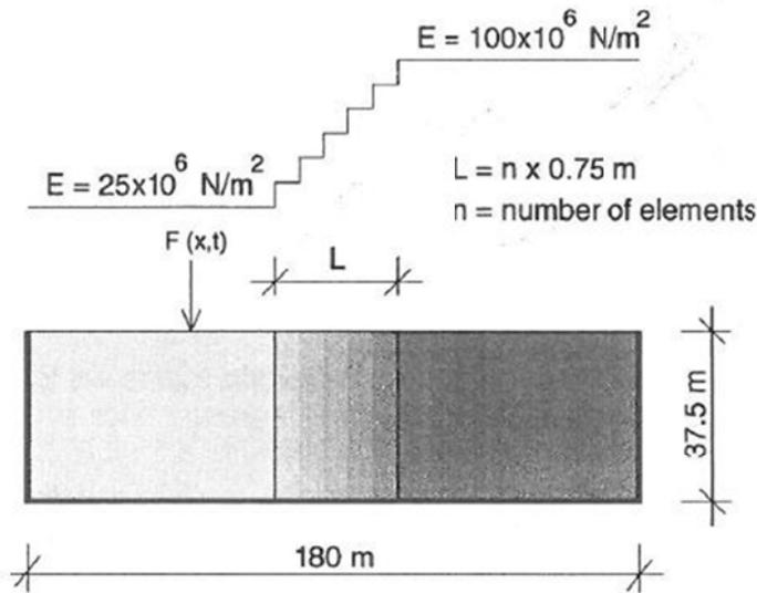
Figure (2.17) Schematic of the modeled elastic half-space with transition zone, figure from [2].
