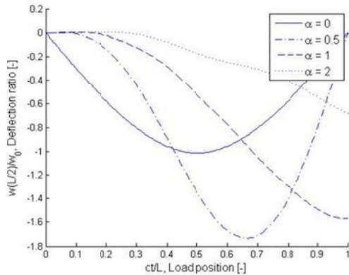
Figure (2.11) Deflection ratio at  $x = l/2$  as a function of load position.
