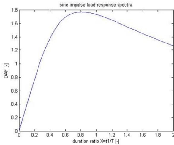
Figure (A.6) *Response spectra for a sine-formed impulse.*
