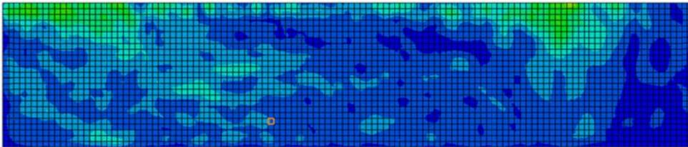
Figure (5.8) *Mises stress a few seconds after impact.*
