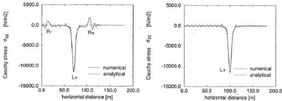
Figure (2.14) Vertical stress after 10 and 40m load propagation at a vertical distance from the surface of 5.68m, figure from [2].
