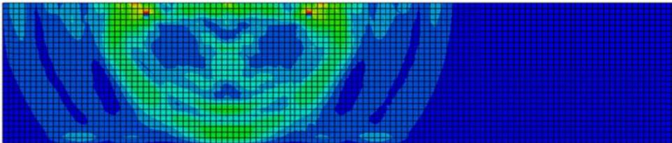
Figure (5.7) *Mises stress at the time slightly after impact with semi-infinite elements.*
