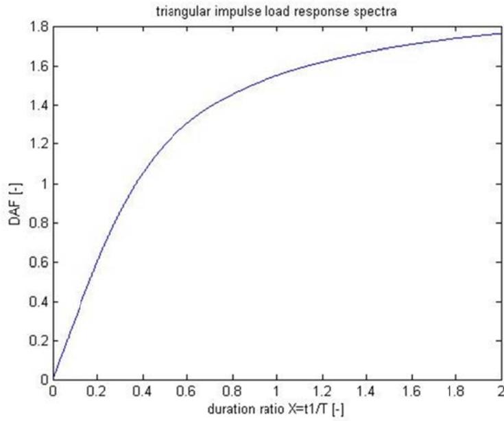
Figure (A.2) Response spectra for a suddenly applied triangular load.
