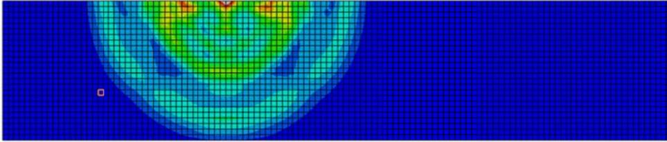
Figure (5.6) *Mises stress at the time just before impact with semi-infinite elements.*
