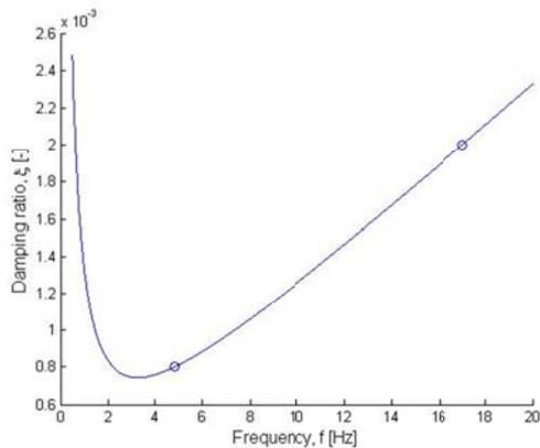
Figure (3.7) *Steel damping distribution.*
