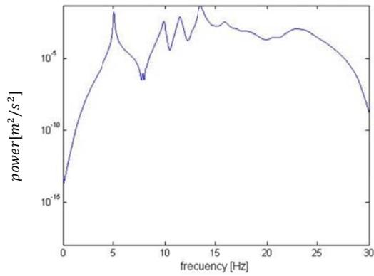
Figure (7.5) *Acceleration PSD at L/4, full model and no transition stiffness.*
