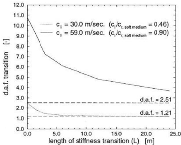
Figure (2.18) *DAF as a function of transition zone length, figure from [2].*
