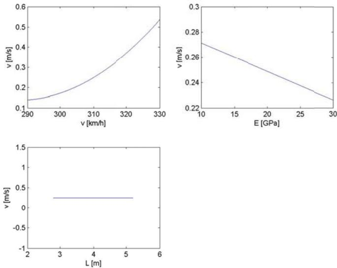
Figure (7.13) Regression function with respect to velocity of each variation parameter on valid interval (when one parameter is varying the other two withhold their mid value).
