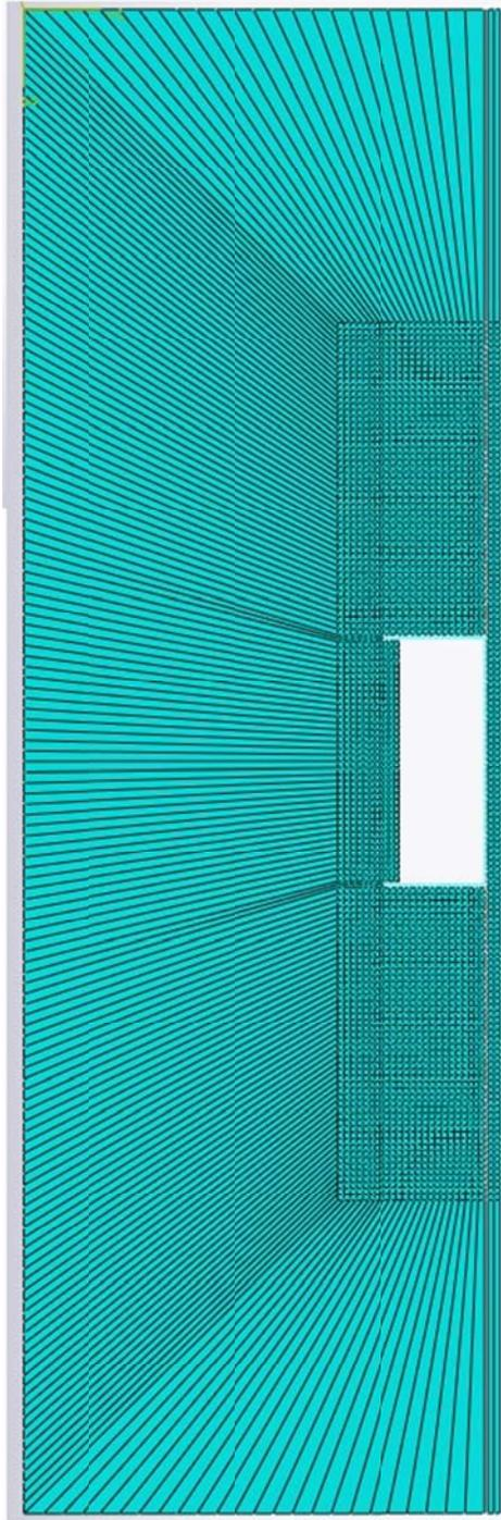
Figure (4.2) Meshed model, 0.4m element size. Note the boundary elements that are used to simulate a semi-infinite half space.
