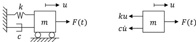
Figure (2.1) *Schematic (left) and free body diagram (right) of friction-free single degree of freedom system.*
