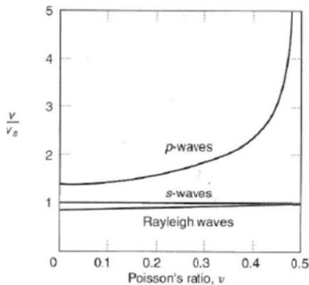
Figure (2.12) Relationship between wave speed ratio and Poisson's ratio,  $v_s$  is shear wave speed, figure from [12].
