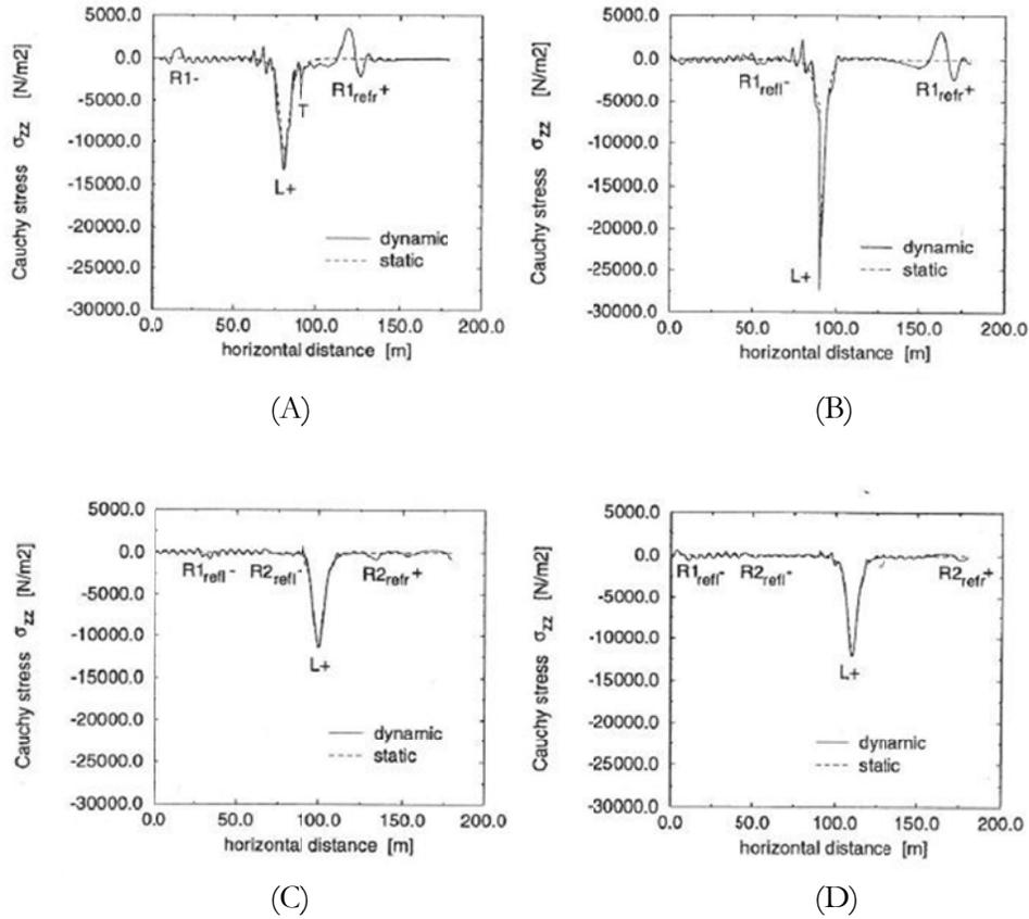
Figure (2.16) Vertical stresses at 5.84m distance from surface,  $c_l/c_{ray,soft}$  medium, figure from [2].
