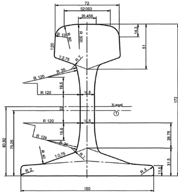
Figure (3.2) UIC60 Cross section, figure from [14]
