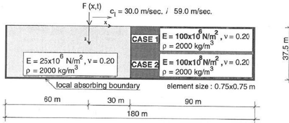
Figure (2.15) Schematic of load model considering a stiffness discontinuity, figure from [2].
