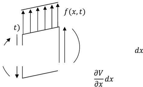
Figure (2.9) *FBD of Euler-Bernulli beam element excited with distributed load.*
