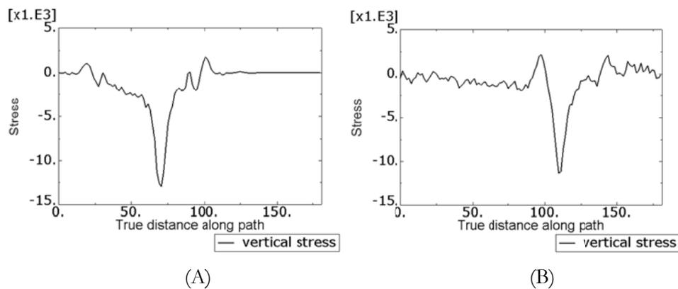
Figure (5.10) Vertical stresses after (A) 10m load propagation and (B) 40m load propagation at a distance from the surface of 6m.
