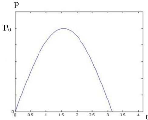
Figure (A.5) *Sine-formed impulse load.*
