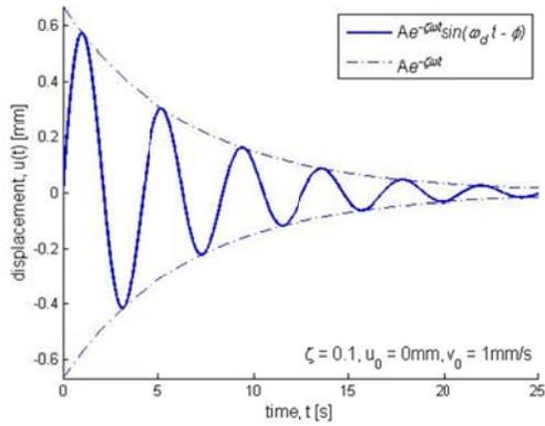
Figure (2.2) Free vibration of an underdamped SDOF-system.
