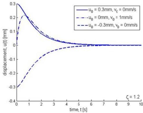
Figure (2.3) Free vibration of an overdamped SDOF-system.
