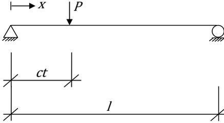
Figure (2.10) Schematic of a simply supported beam subjected to a moving load.
