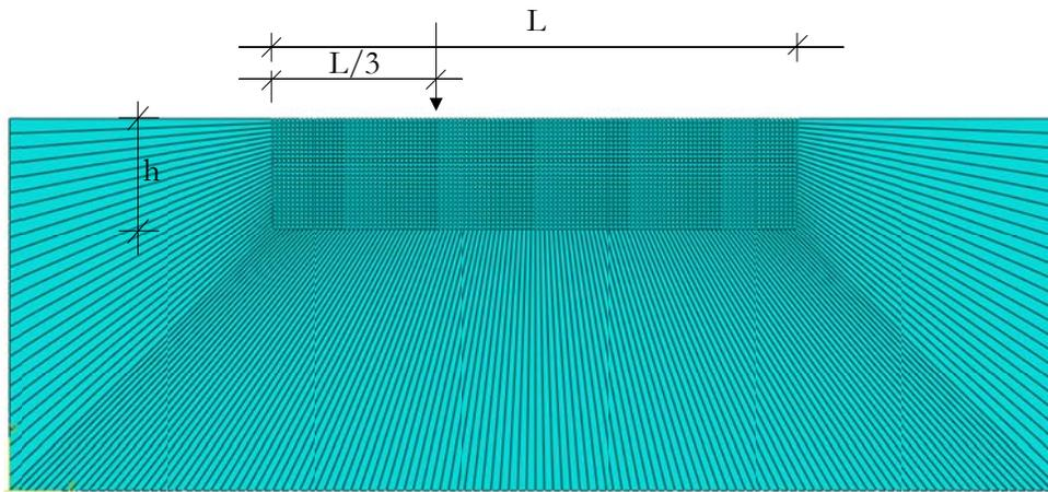
Figure (5.4) Schematic of loading and mesh,  $L=180m$   $h=37.5m$ , element size= $1.5m$ .
