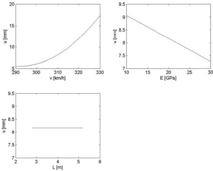
Figure (7.12) Regression function with respect to displacements of each variation parameter on valid interval (when one parameter is varying the other two withhold their mid value).
