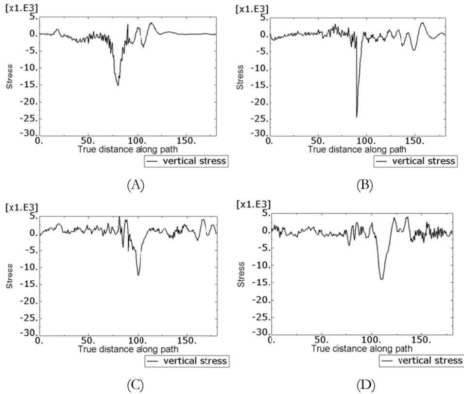
Figure (5.12) Vertical stress after (A) 20m, (B) 30m, (C) 40m and (D) 50m load propagation.
