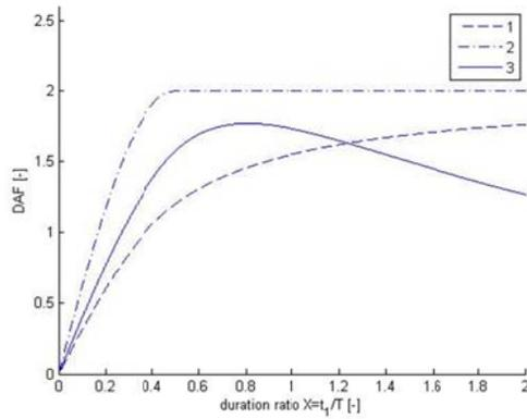
Figure (2.8) *Impulse response spectra. Dynamic amplification factor of SDOF system subjected to various formed impulse loads, 1. rectangular, 2. suddenly applied triangular, 3. sine formed.*
