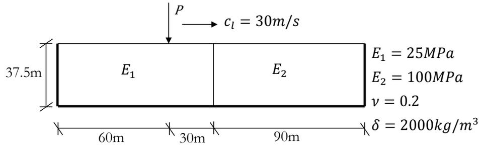
Figure (5.11) Schematic of model with a stiffness discontinuity.
