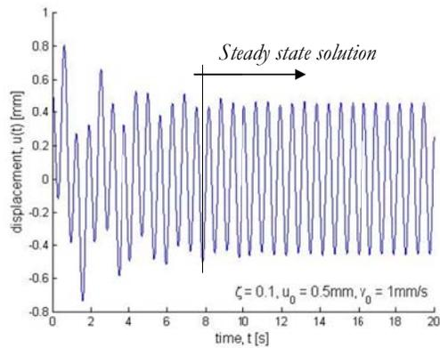
Figure (2.5) Harmonically excited underdamped SDOF-system.
