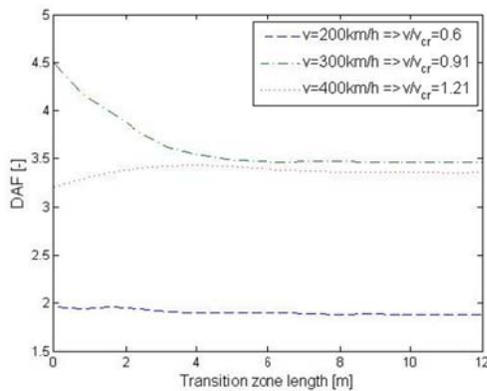
Figure (7.15) Dynamic amplification factor (DAF) as a function of transition zone length.
