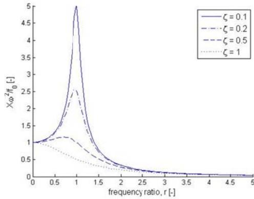
Figure (2.6) *Illustration of resonance expressed in steady state displacement.*
