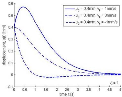
Figure (2.4) Free vibration of a critically damped SDOF-system.
