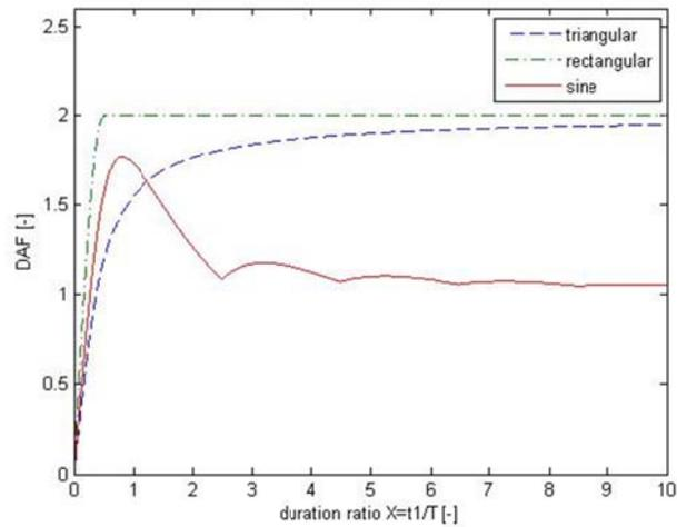
Figure (A.7) *Response spectra for three different impulse forms.*
