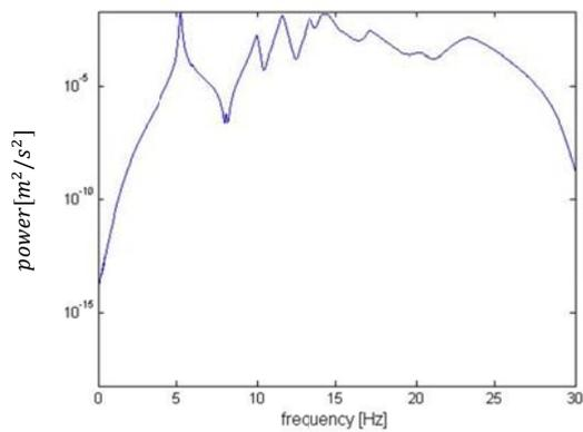
Figure (7.6) *Acceleration PSD at L/4, full model and stiffest transition zone.*
