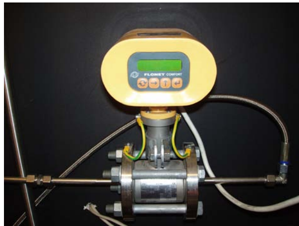
Figure 2.15: Flow meter FLONET FR 2014.
