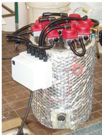
Figure 2.11: Peak heater for black liquor.
