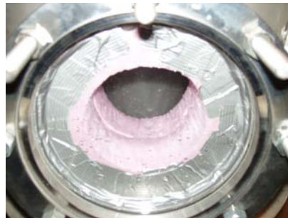
Figure 2.2: Window purging system models mounted in one of the optical access ports in the spray test rig.
