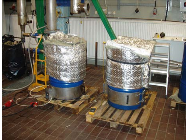
Figure 2.10: Storage and heating of black liquor.
