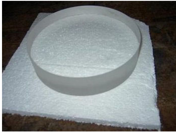
Figure 1.8: Quartz glass for Optical Access Windows.
