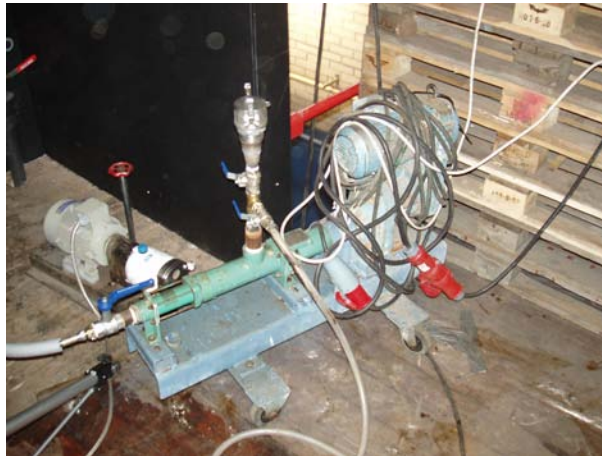
Figure 2.12: N 20 excenterscrew pump.
