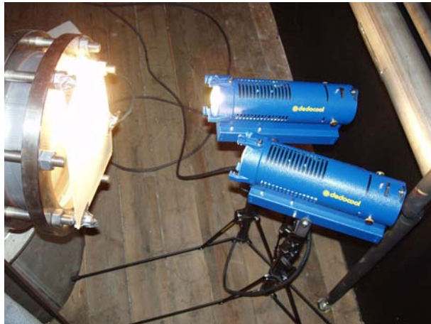
Figure 2.18: COOLH Dedocool Tungsten Light Head with a diffuser between the optical access window and the lighting.
