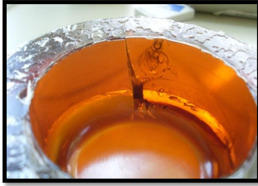
Figure 52 : Samples for electrical breakdown test with an apparent crack (Walls: Epoxy reference, Plate: reference with 30vol% clean Atlas 1/7 glass fabric)
