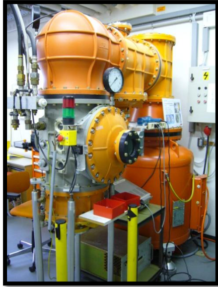
Figure 28 : Chamber for electrical breakdown testing
