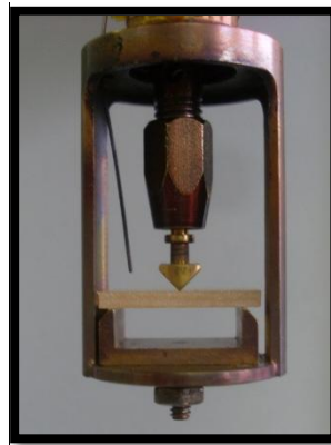
Figure 24 : Storage and loss modulus measurements, for 3-points bending
