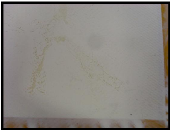
Figure 39 : Stripes on the small plate with 18wt% P2 (70nm) and 30vol% glass fabric
