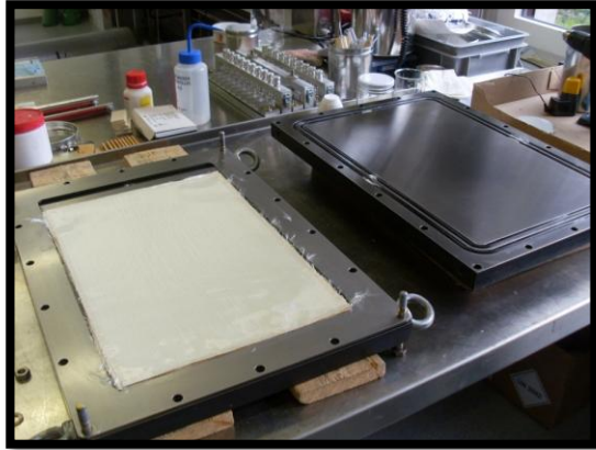
Figure 19 : Mold for preparing laminates of glass fabrics reinforced epoxy resin (on the left: top of the mold with the glass fabrics, on the right: bottom of the mold)
