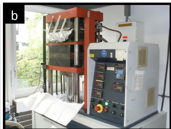
Figure 21 : a: impregnation of the fabrics with a spatula, b: hydraulic press for making wet lay plates
