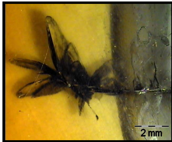
Figure 53 : samples after electrical breakdown test without the walls - Electrical breakdown trees - a: Reference resin only (R02), b: reference resin with 30vol% clean glass fabrics (GR01)
