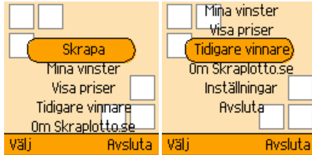
Figure 7.2: The application on a 128x128 pixel display. Note how some of the menu options are off screen.
