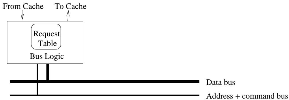
Figure 8. Split transaction bus, the bus logic includes a request table used to keep track of outstanding requests.
