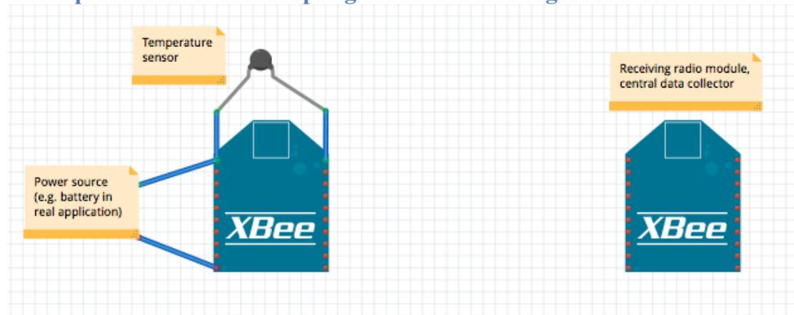
**Figure 5: Experiment setup for wireless (ZigBee protocol) data transfer**
