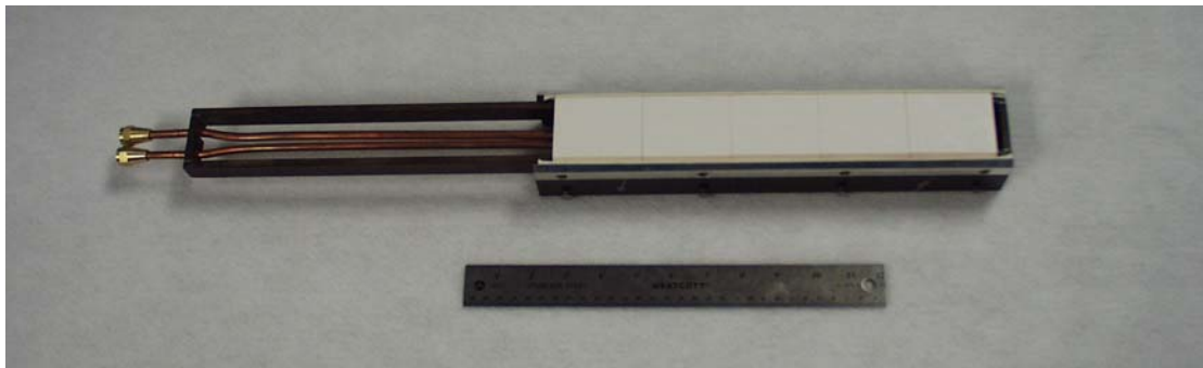
Figure 7 - Induction coil in its "case" made from quartz plates
