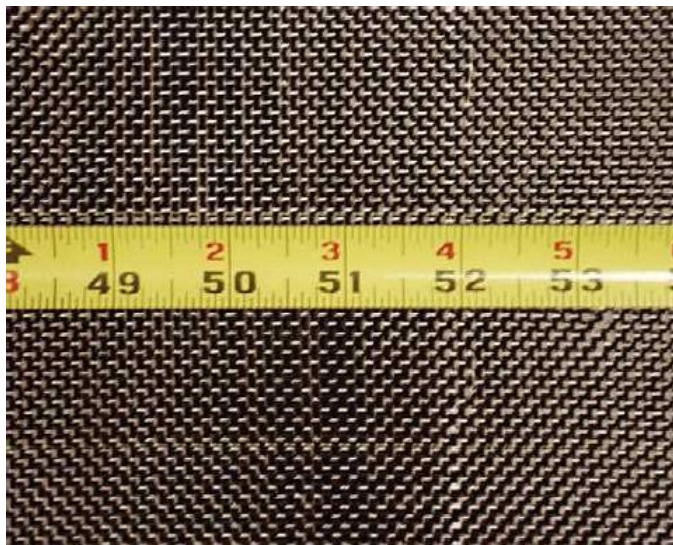
Figure 10 – The carbon fiber weave that was used in the experiments. Scale in inches.
