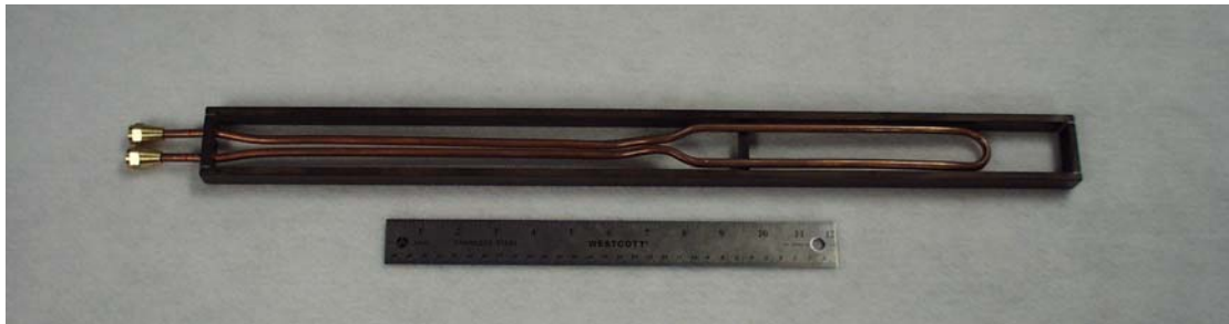
Figure 6 - Copper induction coil optimized for the RAIL process
