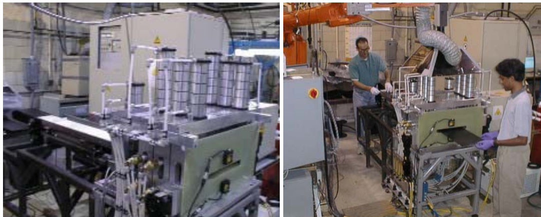
Figures 1-2 - The factory laminator successfully completed trials and is now fully operational at Alliant TechSystem's production line. The photos were taken in the CCM lab during the development work.
