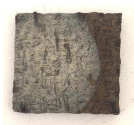
Figure 14 : Picture of visible propagation front on incomplete reaction preforms
