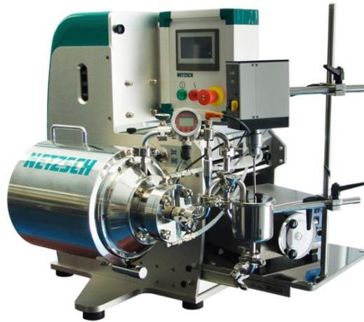
Figure 8 : Wet ball milling and circulation device from NETZSCH; source: <http://www.netzsch-grinding.com>
