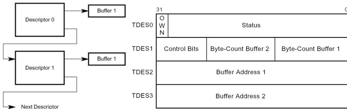
Figure 17: Descriptor chain structure    Figure 18: Transmit descriptor format
