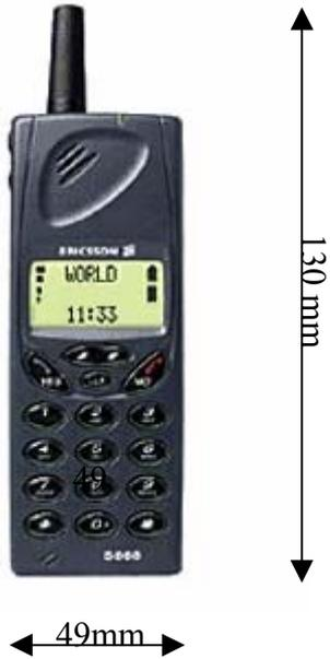
The size of an Ericsson S868 can be seen in the picture, the depth is 23 millimetres and it weights 130 grams with a slim battery.
