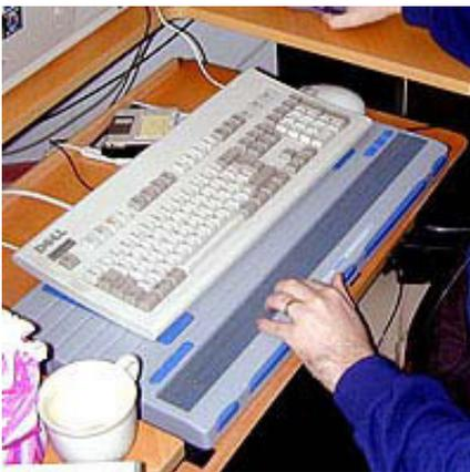
**Figure 10** A setup of a Braille display and a regular keyboard and mouse (Holm & Tenhunen, 2004).
