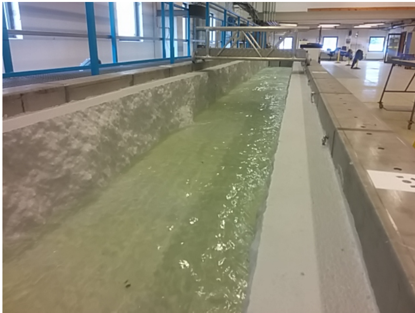
Figure 1.1: Open-channel with rough walls at Vattenfall Research and Development in Älvkarleby.
