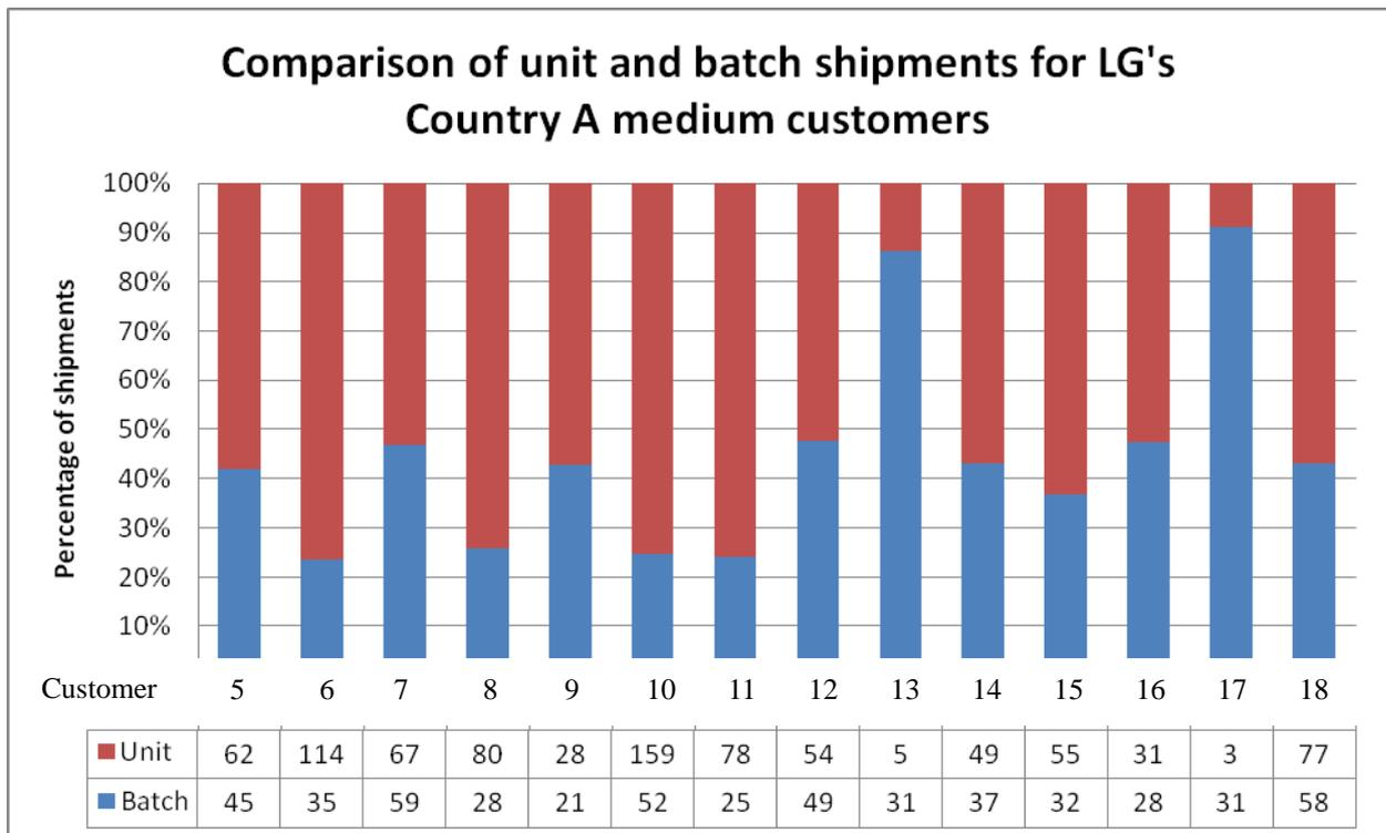
Graph 5.9 Comparison of unit and batch shipments for medium customers in country A (23-80% batch shipments with an average of 8 cubic meters per shipment).
