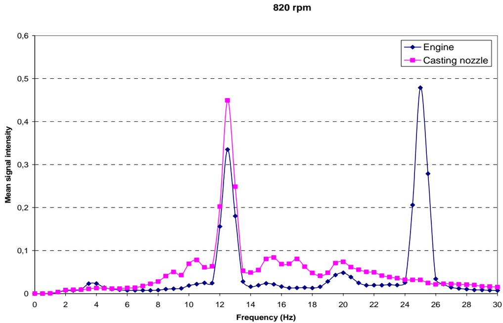
**Figure C 11.** Mean signal intensity for a frequency spectrum of 0-30 Hz at a pumping velocity of 820 rpm
