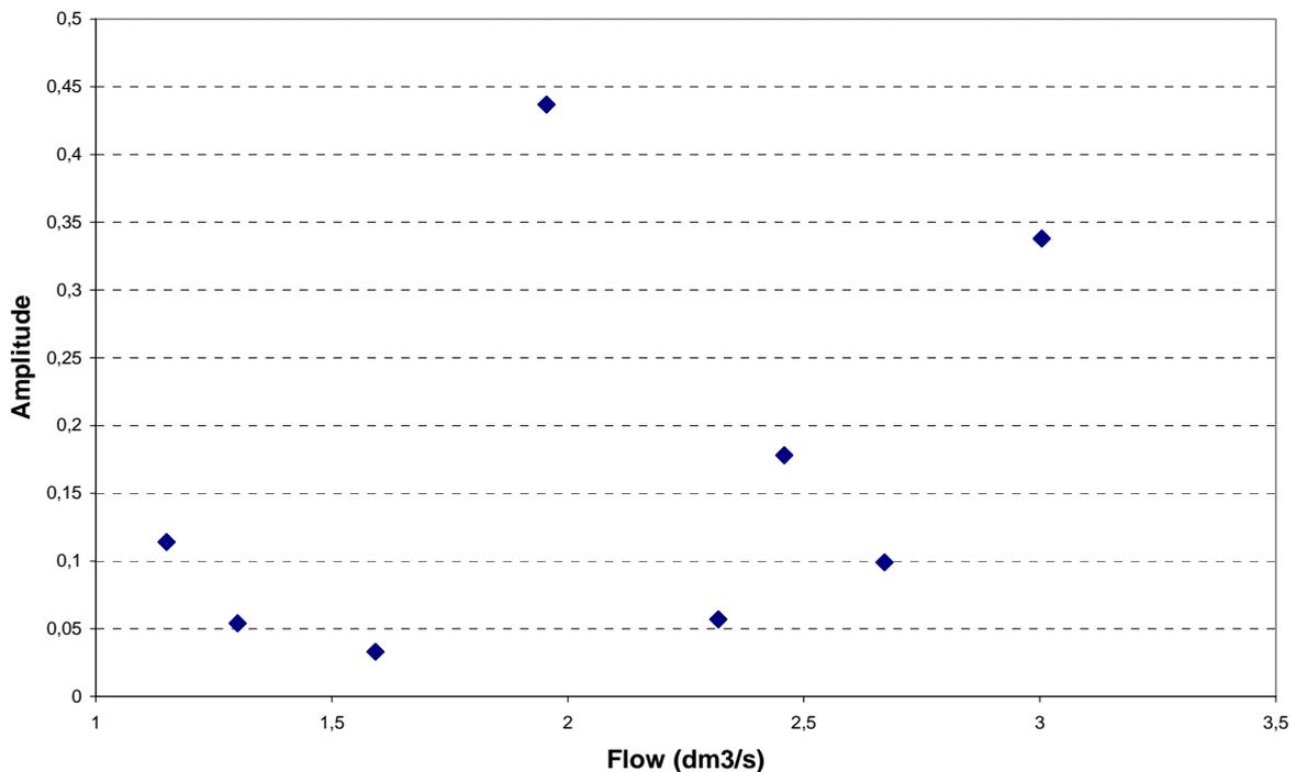
**Figure 26.** Amplitudes as a function of flow of the highest peak of the corrected signal
