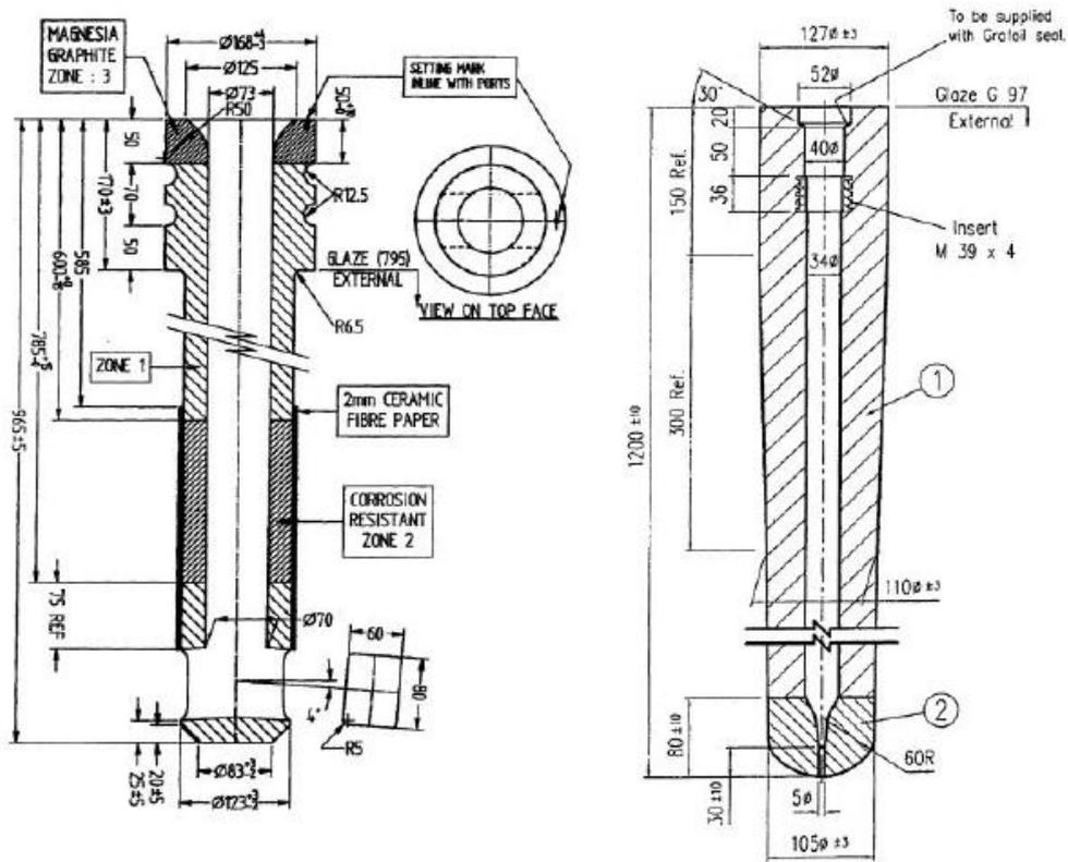
Figure 5. Cross section of an entry nozzle to the left and a stopper rod to the right
