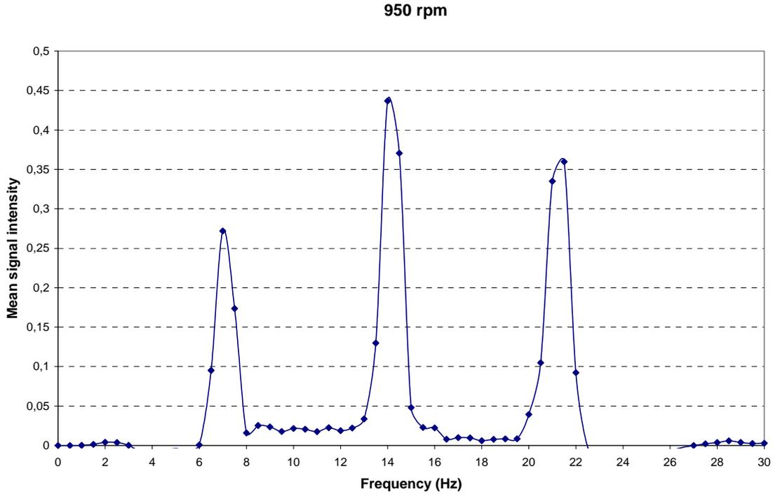
**Figure 19.** Mean signal intensity as a function of frequency in a spectrum reaching from zero to 30 Hz at a pumping velocity of 950 rpm.
