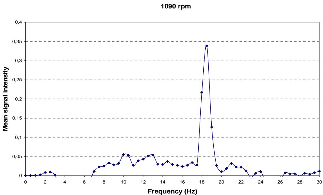
**Figure 23.** Mean signal intensity as a function of frequency in a spectrum reaching from zero to 30 Hz at a pumping velocity of 1090 rpm
