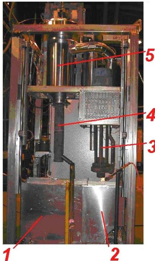
**Figure 10.** Physical model design; 1:Mould; 2:Pump section; 3:Centrifugal pump; 4:Casting nozzle; 5:Tundish
