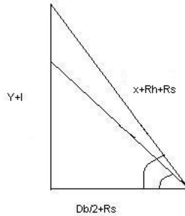
**Figure A 5.** The line of separation between stopper and nozzle seat can be described by the changing hypotenuse, which will be dependent on the lift angle and stopper lift
