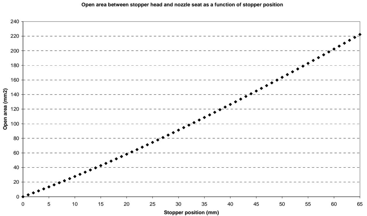
**Figure A 8.** Open area, mm<sup>2</sup>, between stopper and SEN seat as a function of stopper lift (mm).
