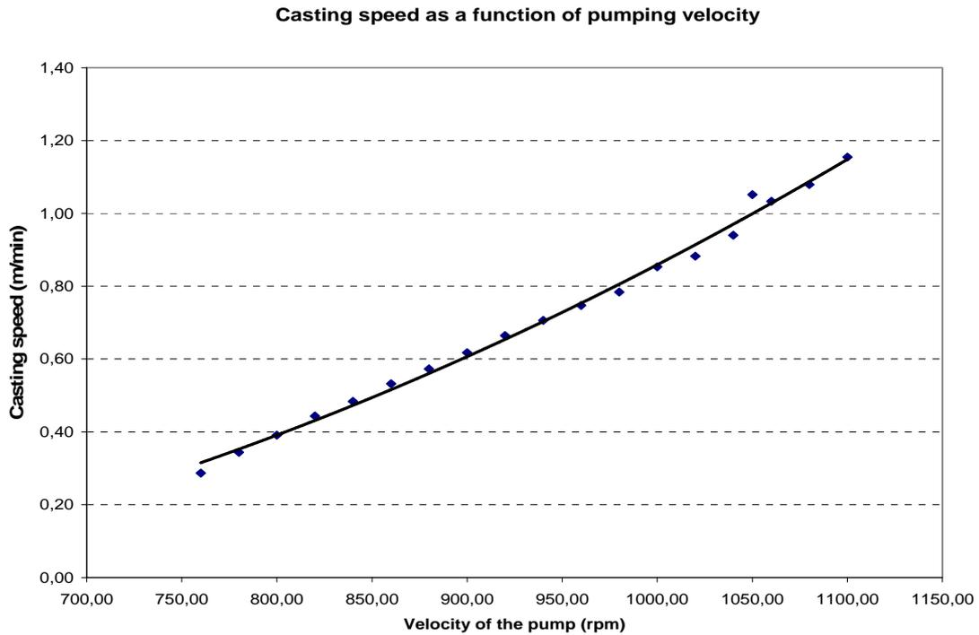
**Figure 14.** Calculated casting speed as a function of pumping velocity
