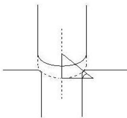
**Figure A 1.** A lift angle can be calculated between stopper head and seat of the submerged entry nozzle.
