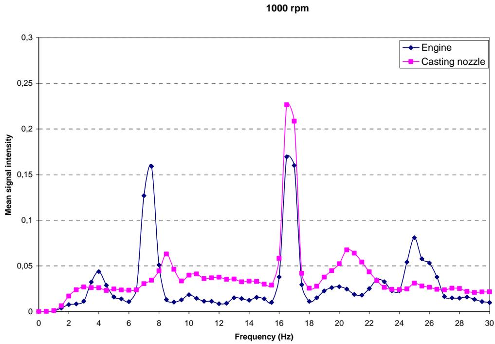
Figure C 15. Mean signal intensity for a frequency spectrum of 0-30 Hz at a pumping velocity of 1000 rpm
