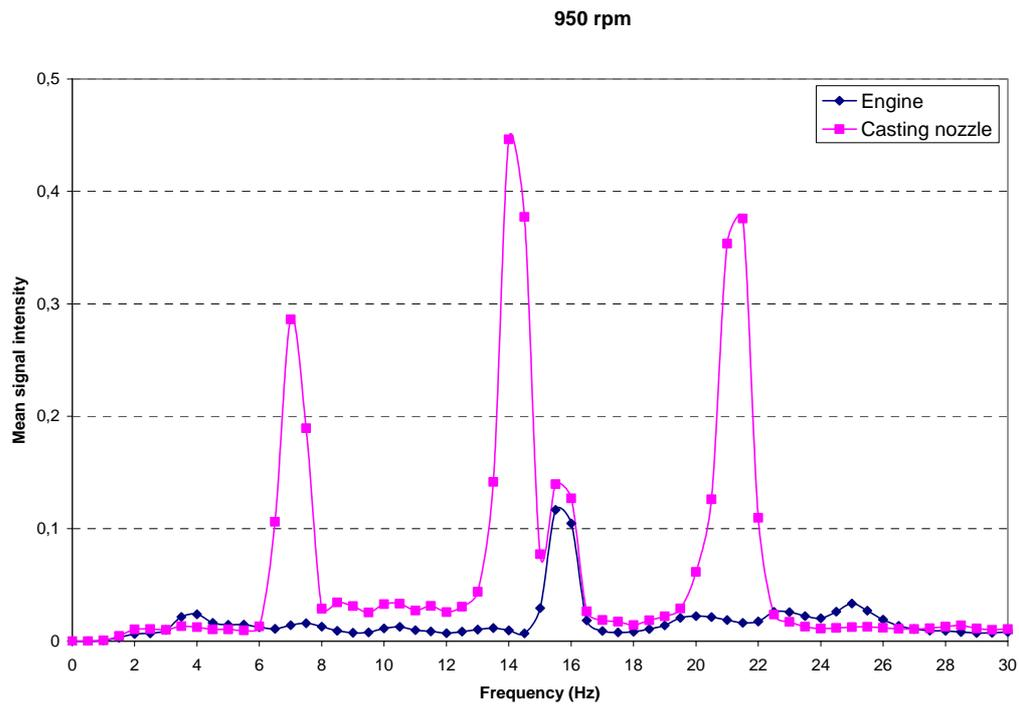
Figure C 14. Mean signal intensity for a frequency spectrum of 0-30 Hz at a pumping velocity of 950 rpm
