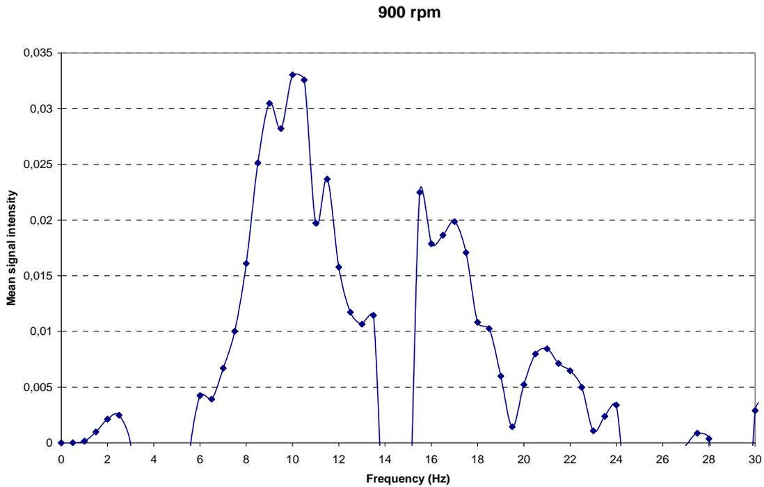
**Figure 18.** Mean signal intensity as a function of frequency in a spectrum reaching from zero to 30 Hz at a pumping velocity of 900 rpm.
