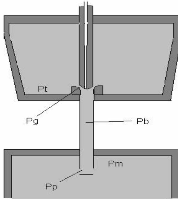
**Figure A 10.** Pressure distribution in tundish and mould can be derived from Bernoulli's equation due to different locations
