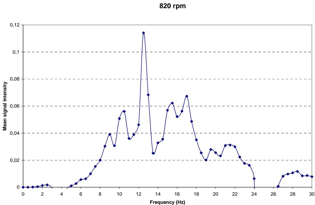
**Figure 16.** Mean signal intensity as a function of frequency in a spectrum reaching from zero to 30 Hz at a pumping velocity of 820 rpm.
