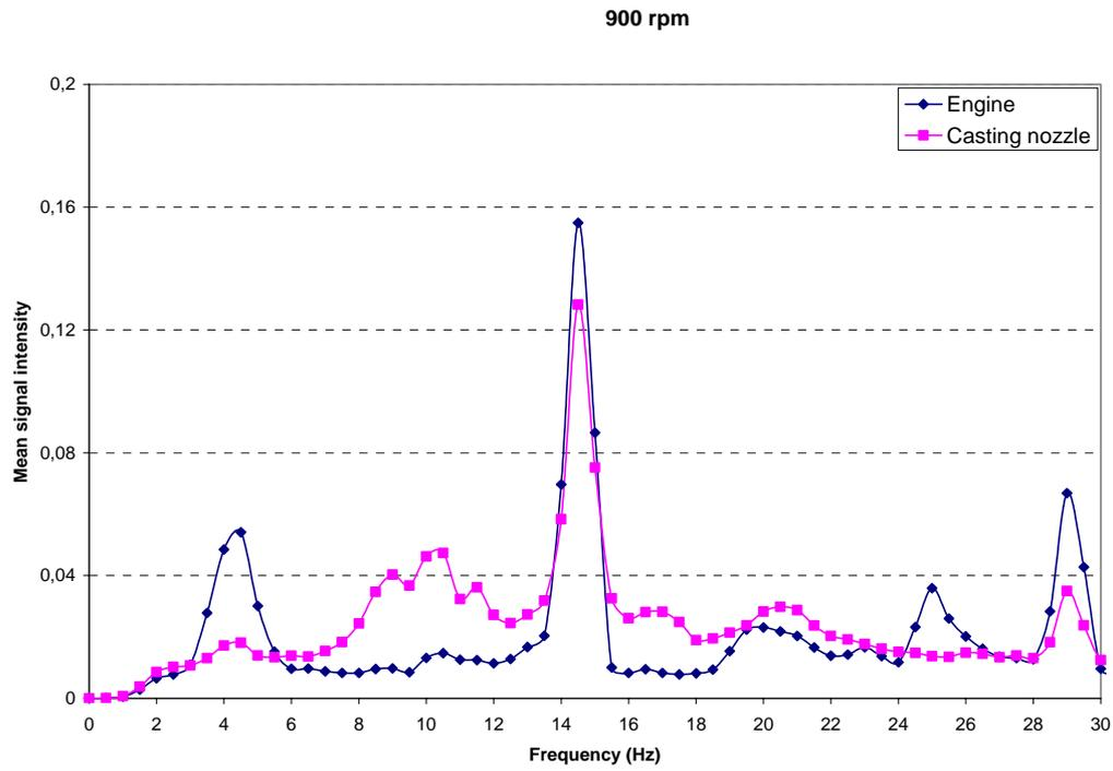
Figure C 13. Mean signal intensity for a frequency spectrum of 0-30 Hz at a pumping velocity of 900 rpm
