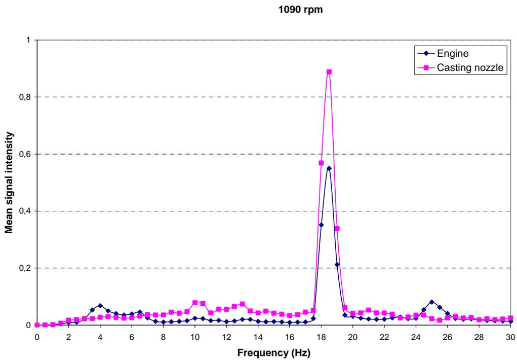
Figure C 18. Mean signal intensity for a frequency spectrum of 0-30 Hz at a pumping velocity of 1090 rpm
