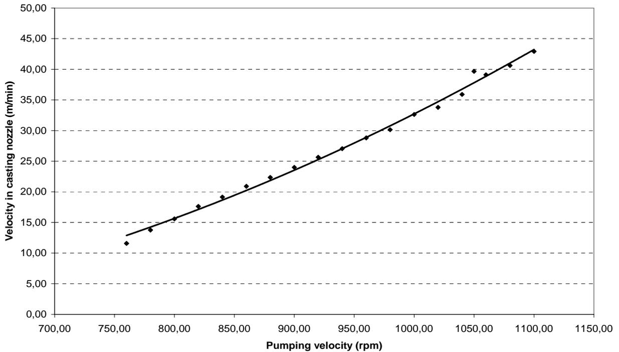
**Figure 13.** Calculated velocity in the submerged entry nozzle as a function of pumping velocity
