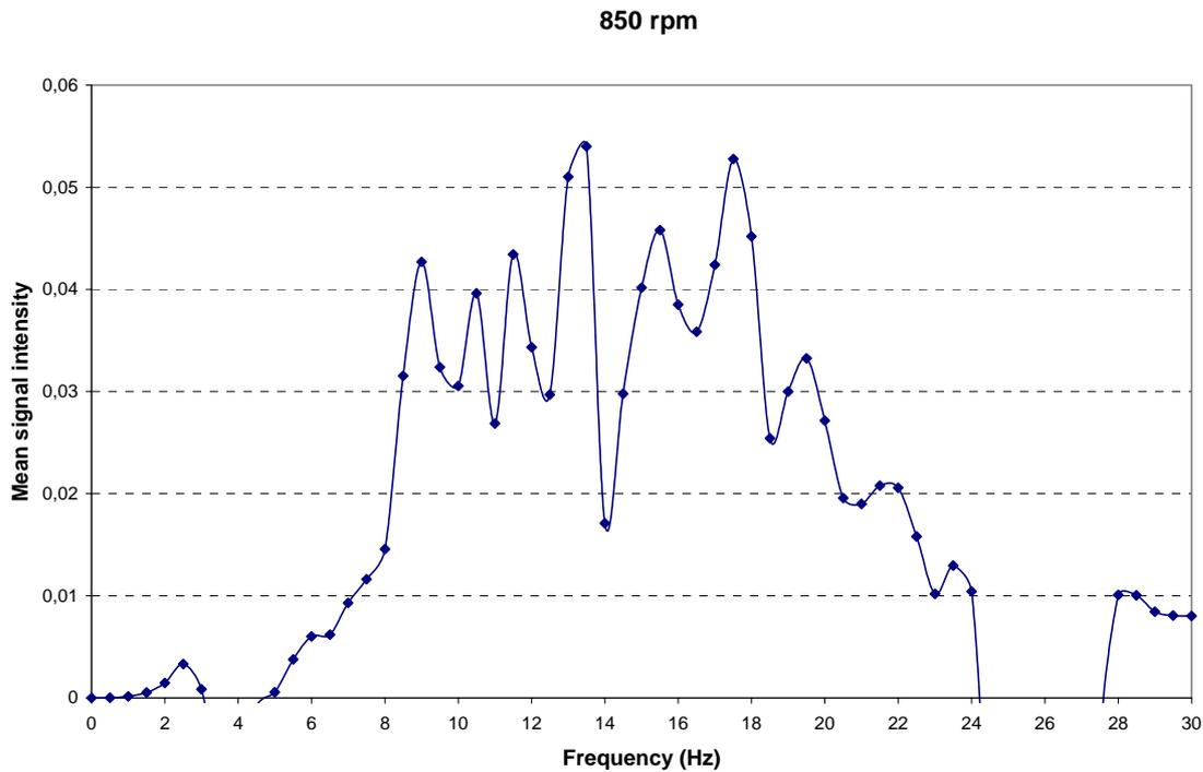
**Figure 17.** Mean signal intensity as a function of frequency in a spectrum reaching from zero to 30 Hz at a pumping velocity of 850 rpm.
