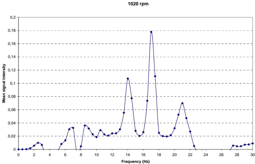
**Figure 21.** Mean signal intensity as a function of frequency in a spectrum reaching from zero to 30 Hz at a pumping velocity of 1020 rpm.
