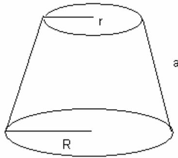
**Figure A 7.** Definition of the sides in the frustum of a right circular cone, which is approximated with the opening of the cross sectional area between the stopper head and the seat of the submerged entry nozzle
