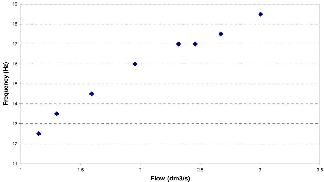
**Figure 24.** Frequency as a function of flow for the largest peak of the measurements made on the casting nozzle for all flows measured
