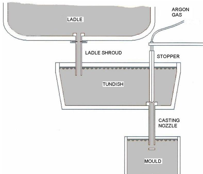
**Figure 3.** Cross section of ladle, tundish and mould [1].
