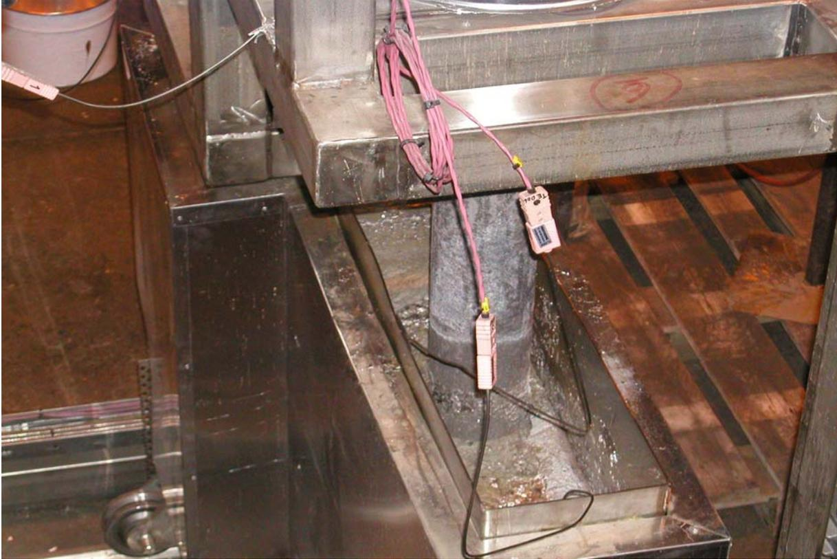
**Figure 11.** Physical model at simulation. The nozzle is submerged into the mould.
