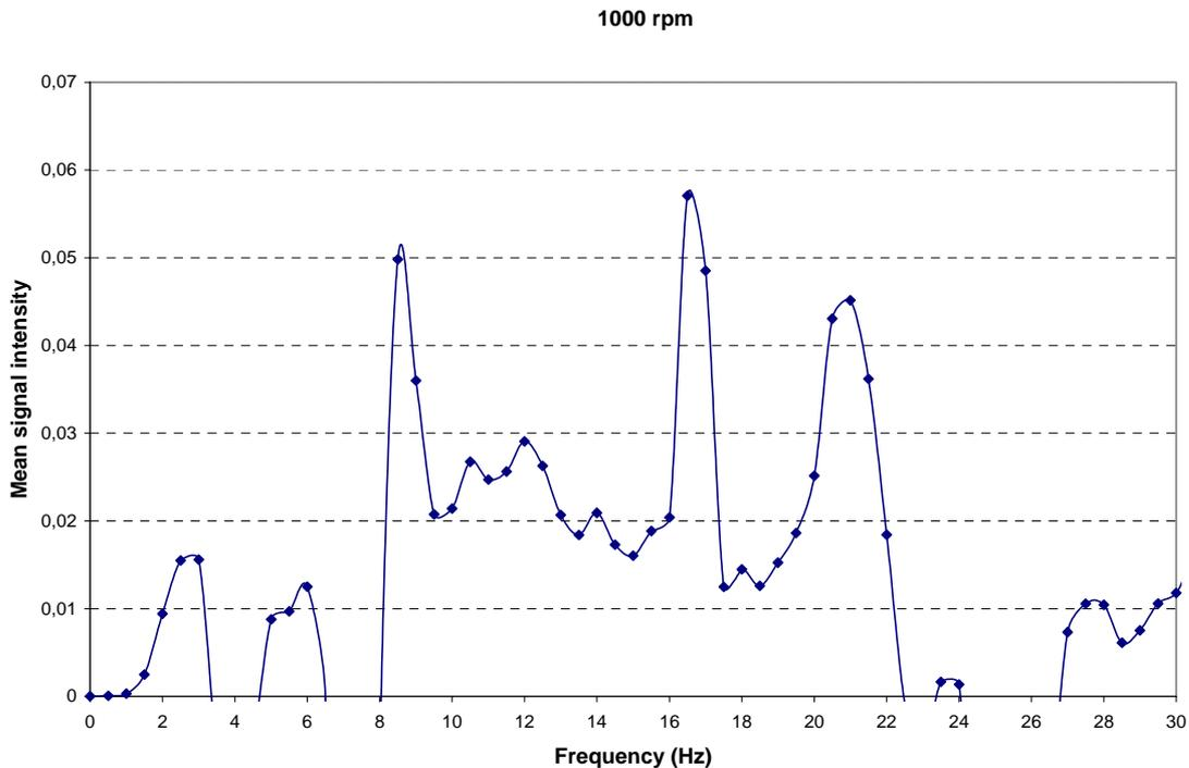
**Figure 20.** Mean signal intensity as a function of frequency in a spectrum reaching from zero to 30 Hz at a pumping velocity of 1000 rpm.
