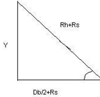
**Figure A 2.** Triangle from figure 14 with defined sides to be able to calculate the closed stoppers lift angle, which refers to the right corner of the triangle in the figure
