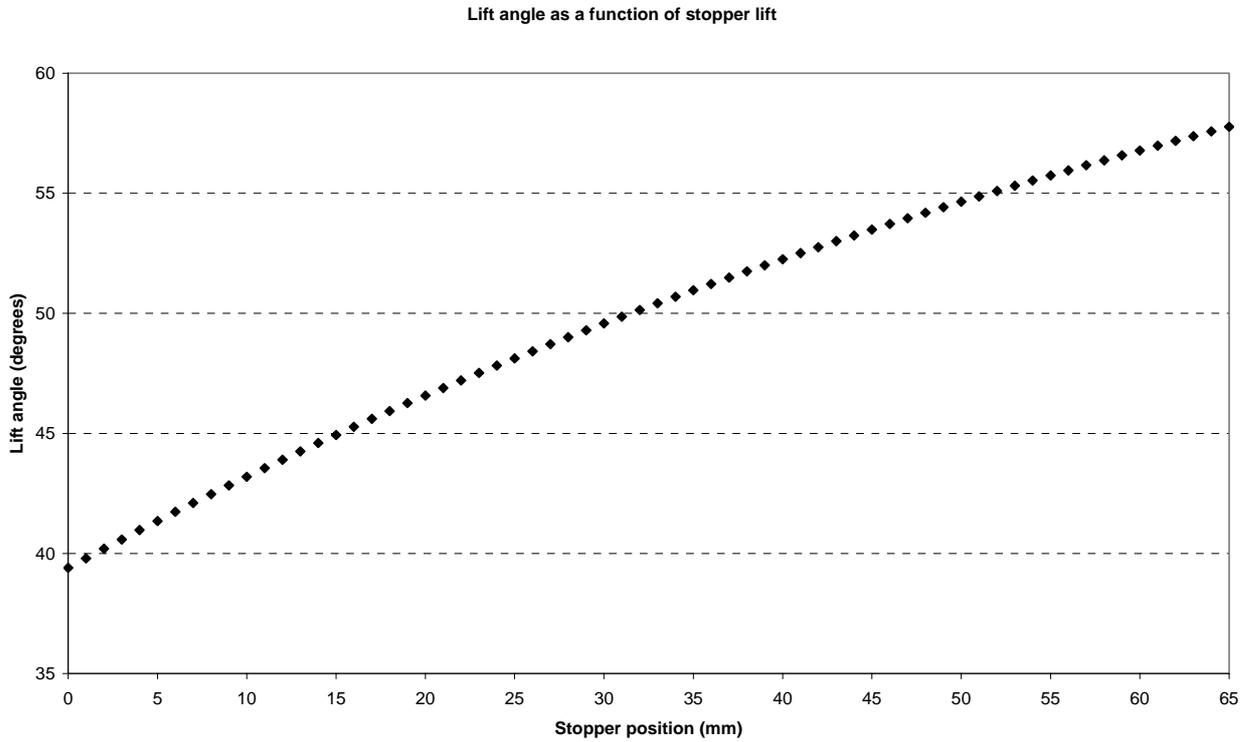
**Figure A 4.** Lift angle as a function of stopper lift.
