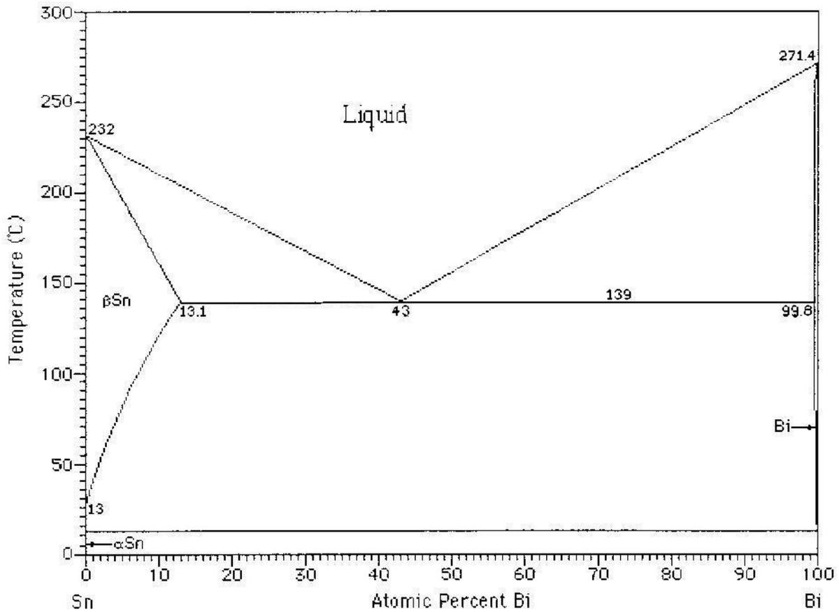
Figure 9. Binary phase diagram of Bismuth and Tin
