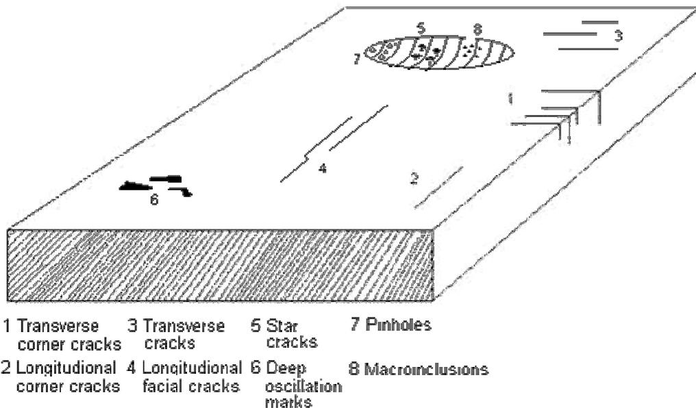
**Figure 4.** Different types of surface defects and cracks on a continuously cast slab [3].
