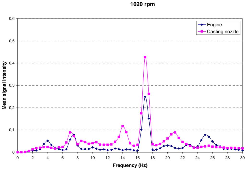
Figure C 16. Mean signal intensity for a frequency spectrum of 0-30 Hz at a pumping velocity of 1020 rpm
