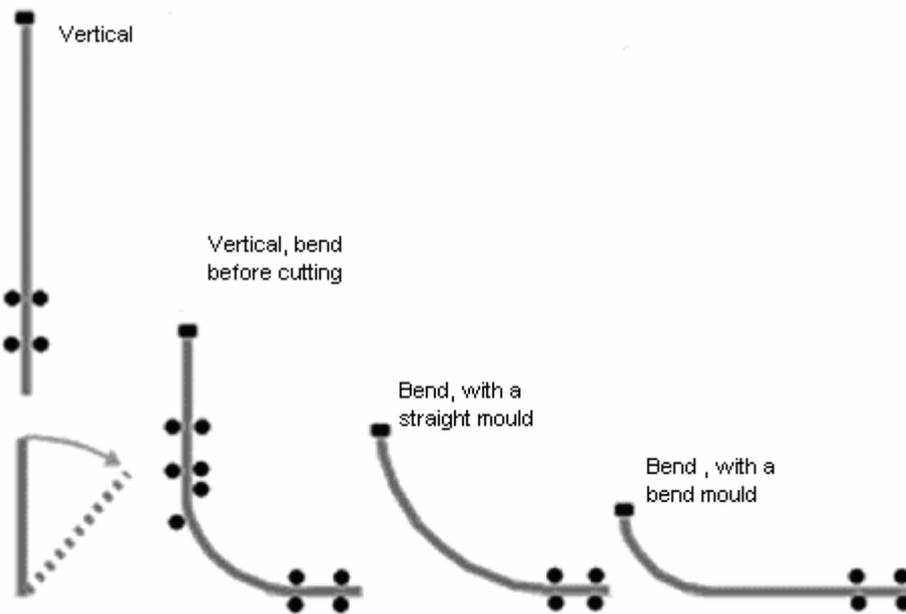
**Figure 1.** Examples of continuously casting machines. The height of the building can be reduced to the right as the height of the machine decreases [2].
