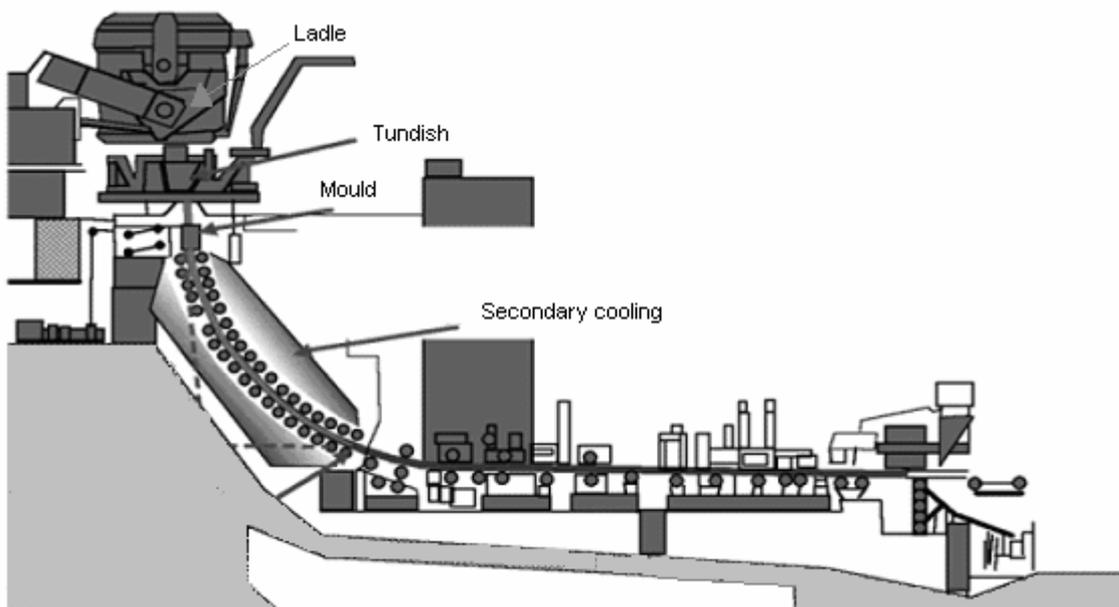
**Figure 2.** Cross section of continuous casting machinery. A ladle is delivered from the secondary steelmaking process with liquid steel. Steel runs through a ladle shroud down to a tundish and further down in the mould [3].
