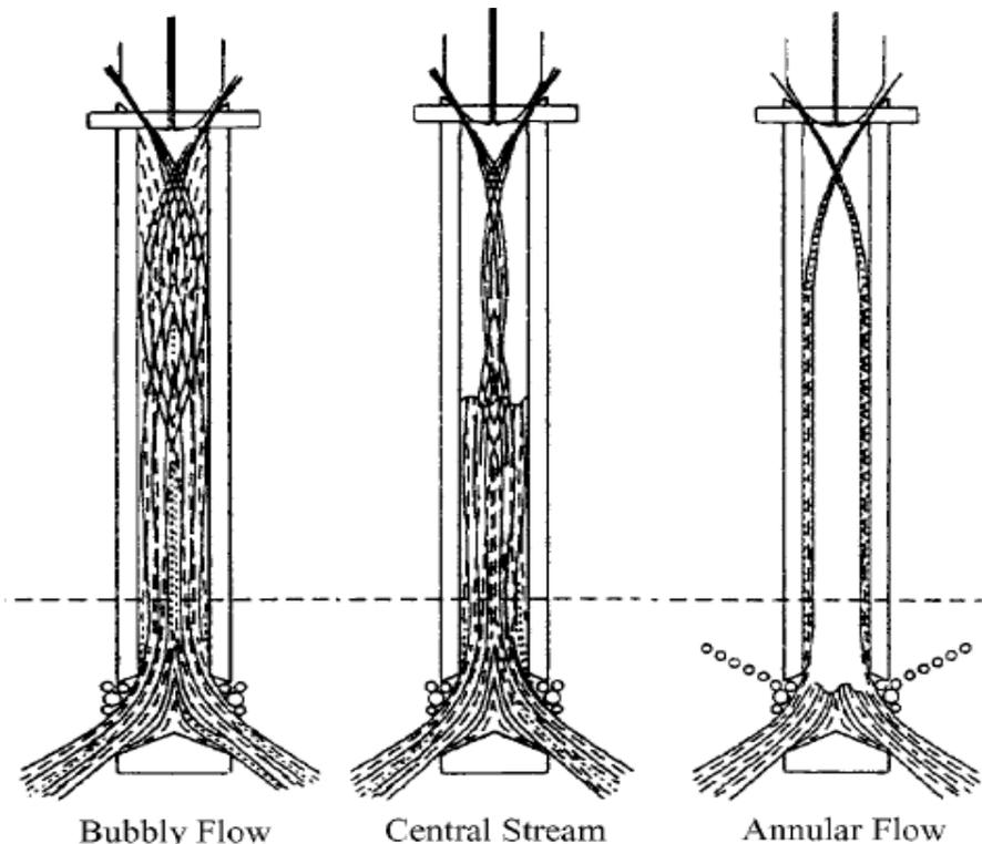
Figure 8. Typical examples of steel flow patterns at casting in a submerged entry nozzle [17].
