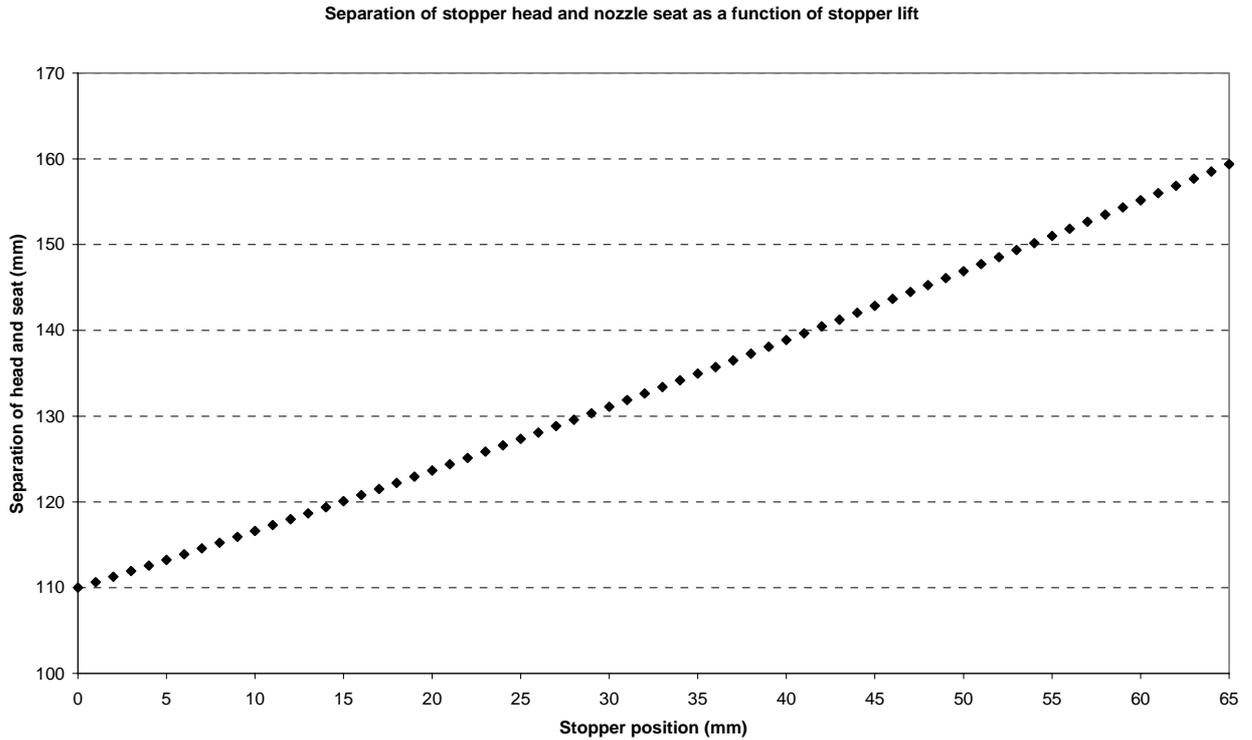
**Figure A 6.** The line of separation between stopper head and nozzle seat is described as a function of stopper lift position
