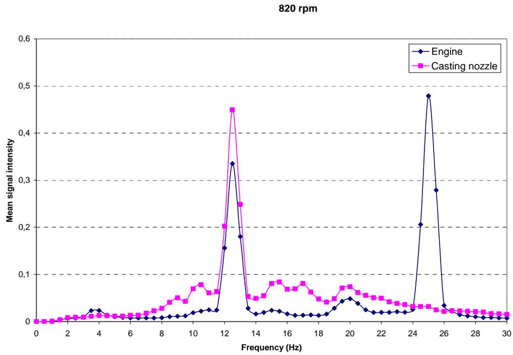
**Figure 15.** The signal from the compact laser vibrometer shows here the mean signal intensity over the frequency spectrum 0-30 Hz at a pumping velocity of 820 rpm
