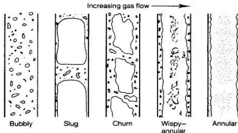
Figure 6. Flow regimes for upward two phase flow in vertical pipes [12].
