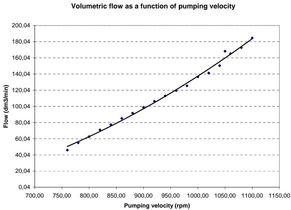
**Figure 12.** Calculated volumetric flow in tundish as a function of pumping velocity
