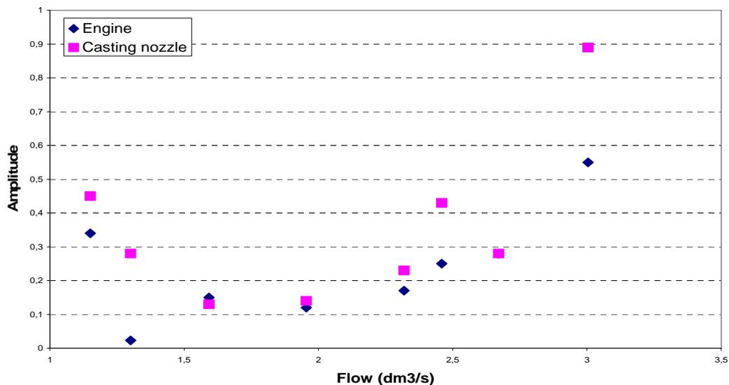
**Figure 25.** Amplitude as a function of flow for the highest peak measured on the casting nozzle. The signal from the engine shows a clear peak at the same frequencies, which is also shown in the diagram
