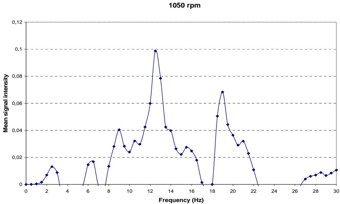
**Figure 22.** Mean signal intensity as a function of frequency in a spectrum reaching from zero to 30 Hz at a pumping velocity of 1050 rpm.
