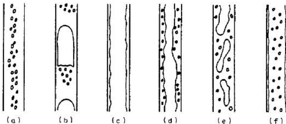
**Figure 7.** Downward co current two phase flow in vertical pipes; a) bubbly flow; b) slug flow; c) falling film flow; d) bubbly falling film flow; e) churn flow; f) dispersed annular flow [14].
