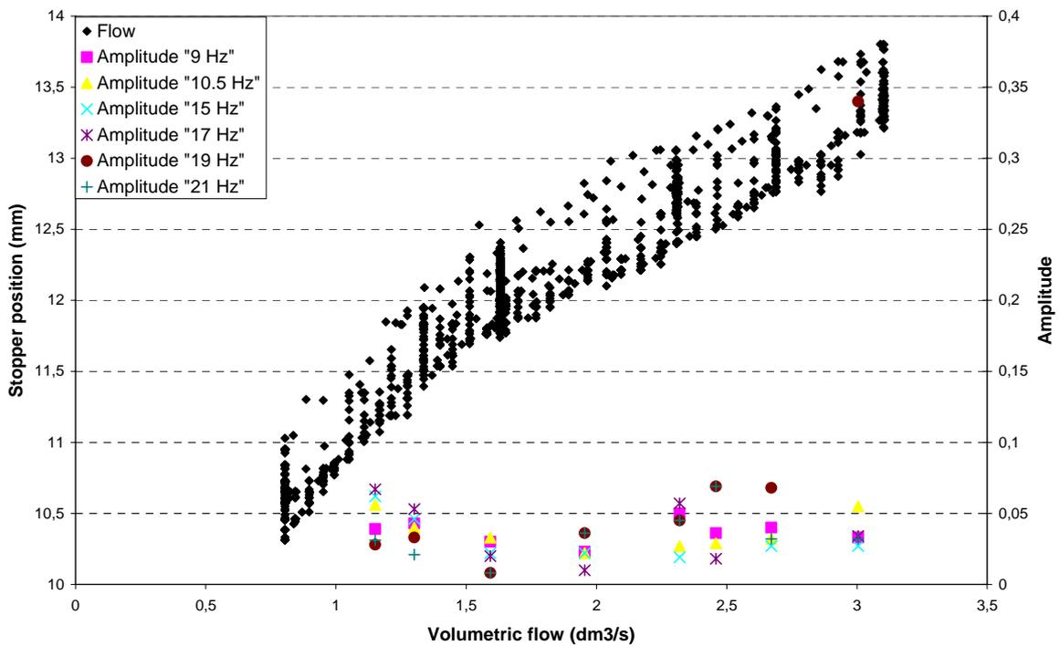
**Figure 32.** Stopper position and amplitude at 9, 10.5, 15, 17, 19 and 21 Hz as a function of volumetric flow in the physical model during the experiments
