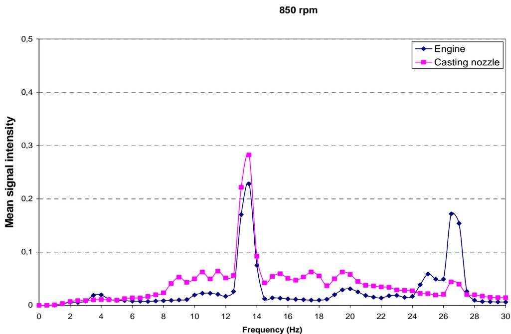
**Figure C 12.** Mean signal intensity for a frequency spectrum of 0-30 Hz at a pumping velocity of 850 rpm
