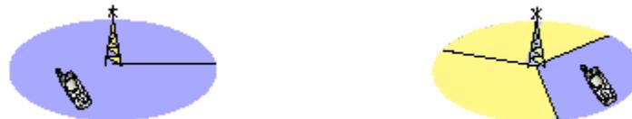
*Figure 3: The result from the CGI represents either a specific circle (omni cell) or a specific circle sector (three-sector cell) in the cell plan.*
