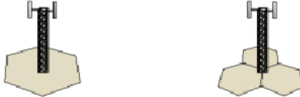
*Figure 2: The left picture shows an omni cell covering 360 degrees, while the right shows a three-sector cell with three smaller cells covering 120 degrees each.*
