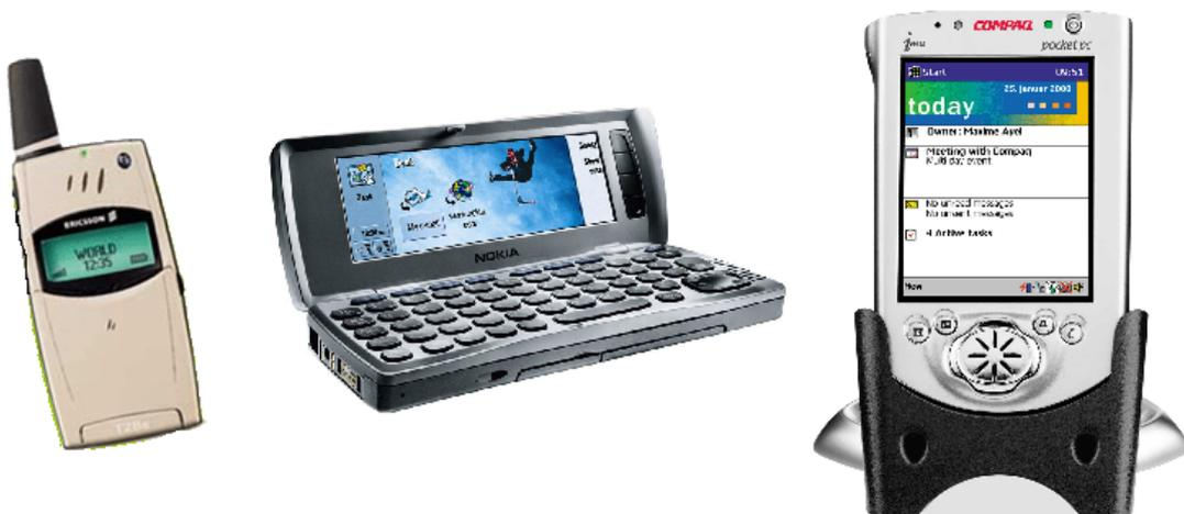
Figure 5: Here is an example of the different kind of terminals available today. The left terminal is a regular mobile phone, the one in the middle is a communicator and the right terminal is a handheld computer. The sizes are not according to scale.
