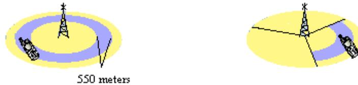
Figure 4: In an omni cell, the result from CGI + TA will be a ring around the base station. If the cell is a three-sector cell the result will instead be a third of a circle. This third is usually called a “banana”.
