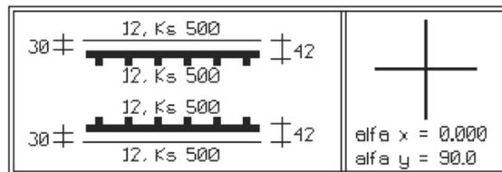
*Figure 4.2* The defined reinforcements and distances of concrete cover.
