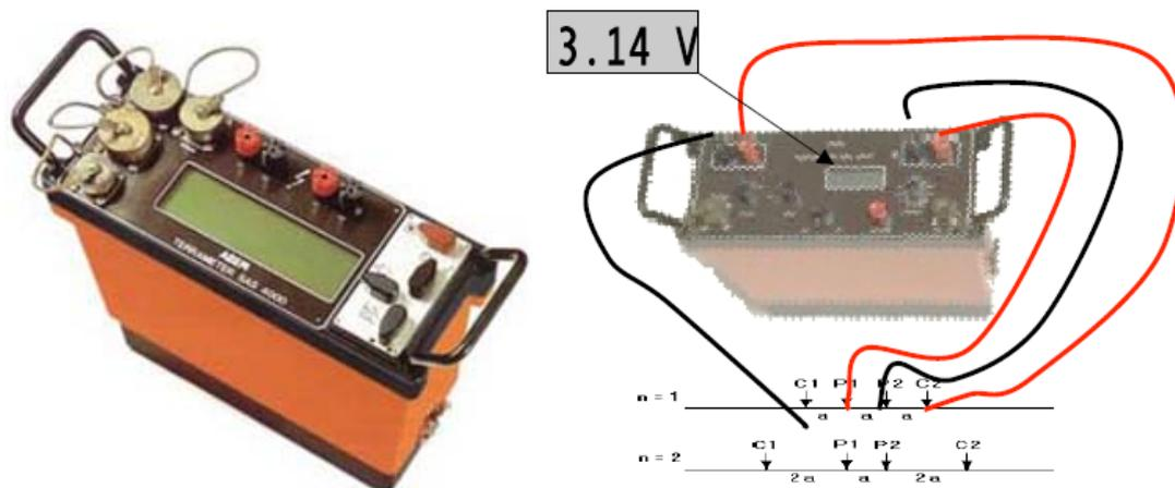
Fig. 3-6: Resistivity instrument and its layout
