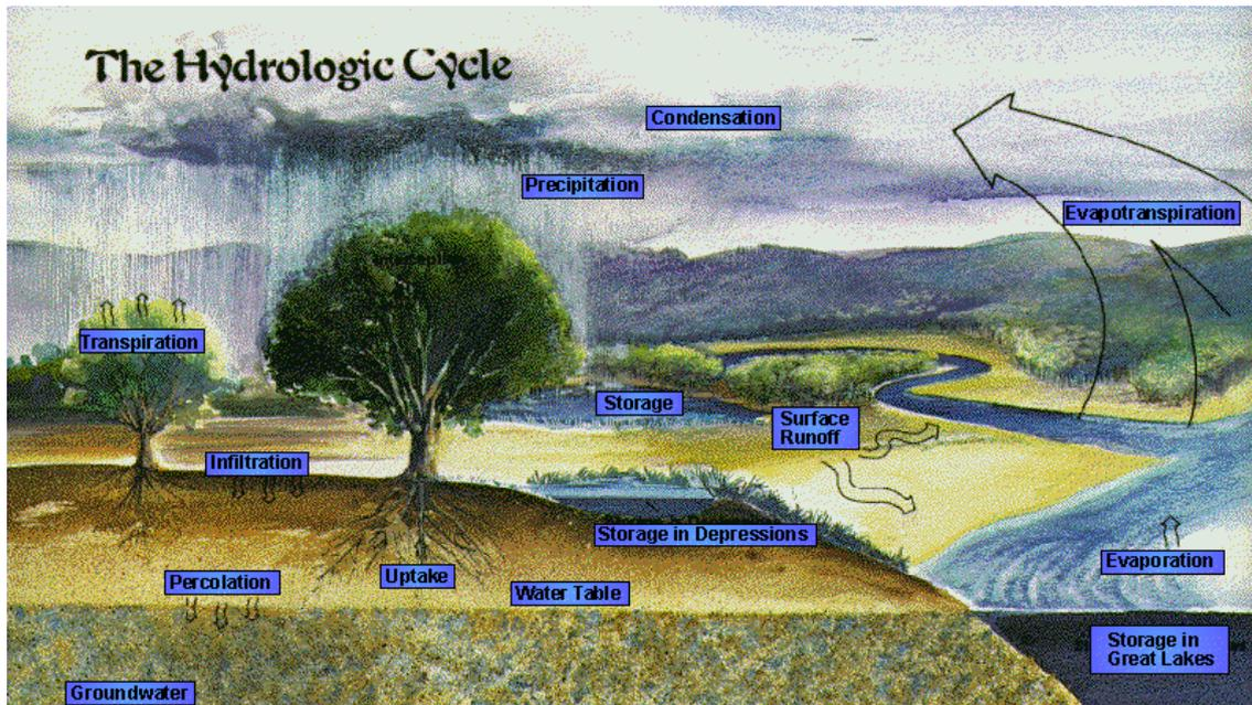
Figure 1-1 Hydrological cycle
