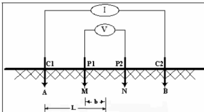
Figure 3.7 The Schlumberger configuration pattern.
