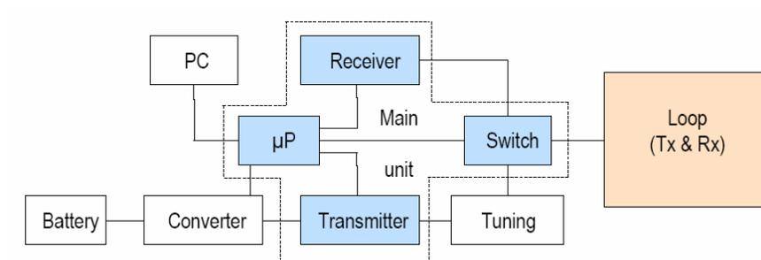
Fig.3-2: NumisPlus Magnetic Resonance System (*Iris Instruments 2002*)
