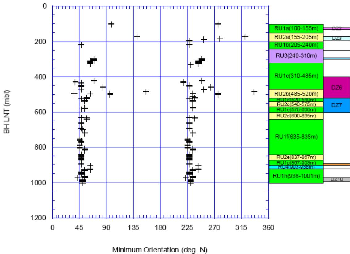
**Figure 32: Correlation of borehole breakouts to lithological rock units and deformation zones in borehole KFM02A.**
