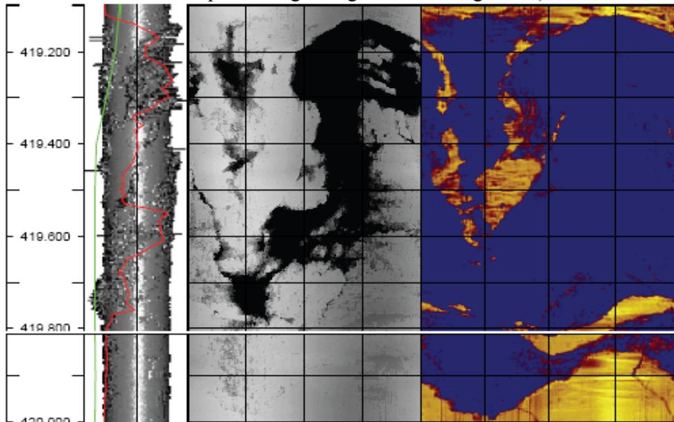
Figure 17: A washout zone (419.0-420.0 mbl) in borehole KFM01B. This zone was clearly visible in three of the BHTV logs (Caliper 3D, travel-time and amplitude log).
