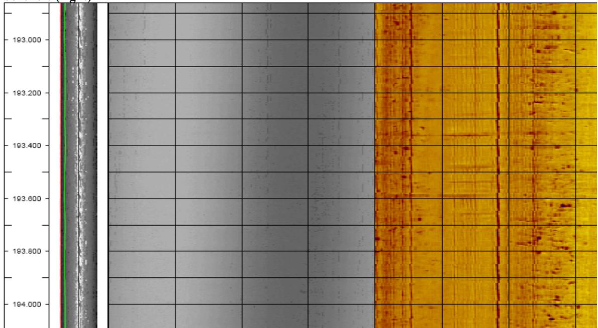
**Figure 23: Example of shallow/low borehole breakout identified in borehole KFM01B from a depth range of about 192.9 to 194.1 mbl. The breakout was only visible in the BHTV amplitude log and appears on both sides of the borehole.**
