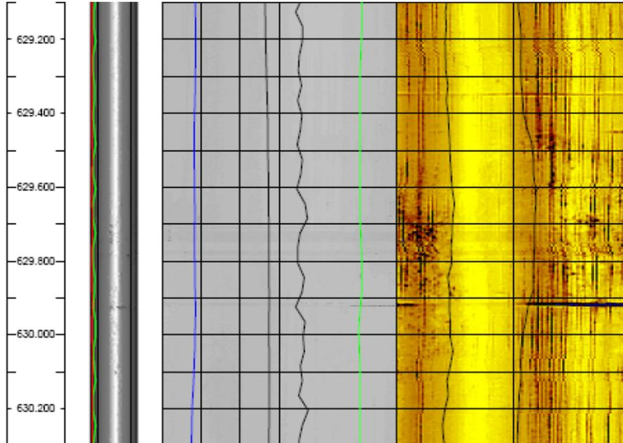
Figure 19: A section (629.1- 630.3 mbl) with a sticky zone in borehole KFM02A. The sticky zone is presented by the blocky patches in BHTV amplitude log.
