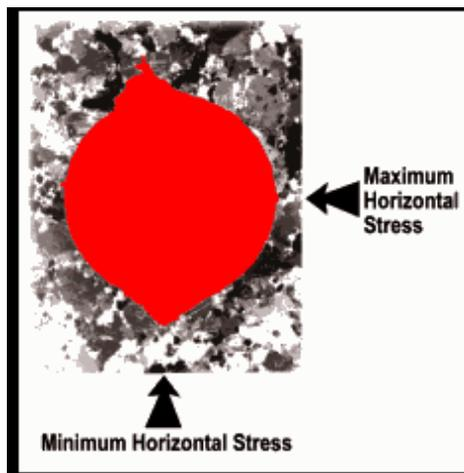
**Figure 3: The laboratory experiment of a borehole breakout in a granite rock [see [http://www.hydrofrac.com/hfb\\_home.html](http://www.hydrofrac.com/hfb_home.html) ]. Note that maximum and minimum horizontal stress concentration at the borehole wall occurs at  $\theta = 90^\circ$  and  $0^\circ$ , respectively.**
