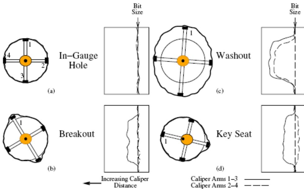
Figure 7: Common types of enlarged borehole and their caliper log response [lifted from *Plumb and Hickman, 1985*]
