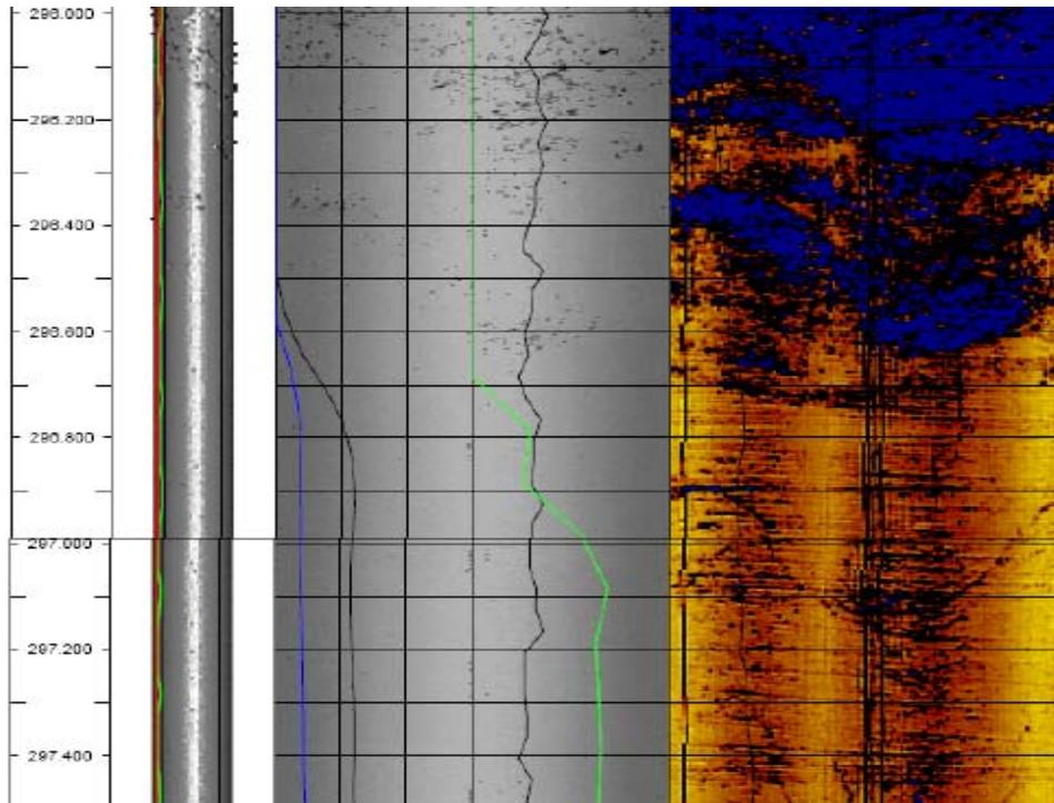
**Figure 28: Borehole breakout identified at 296-297.5 mbl in borehole KFM02A. The breakout was partly concealed by a washout at 296-.296.7 m.**
