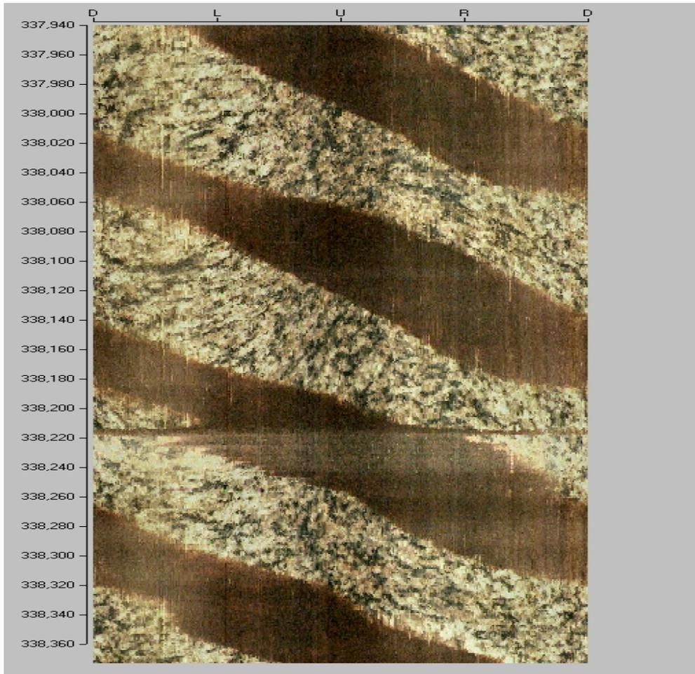
**Figure 13:** Showing a section (337.94-338.36 mbl) of BIPS image in borehole KFM02A with spiral grooves, which appear as a dark diagonal bands that run across the borehole wall (i.e., across the crystalline rock).
