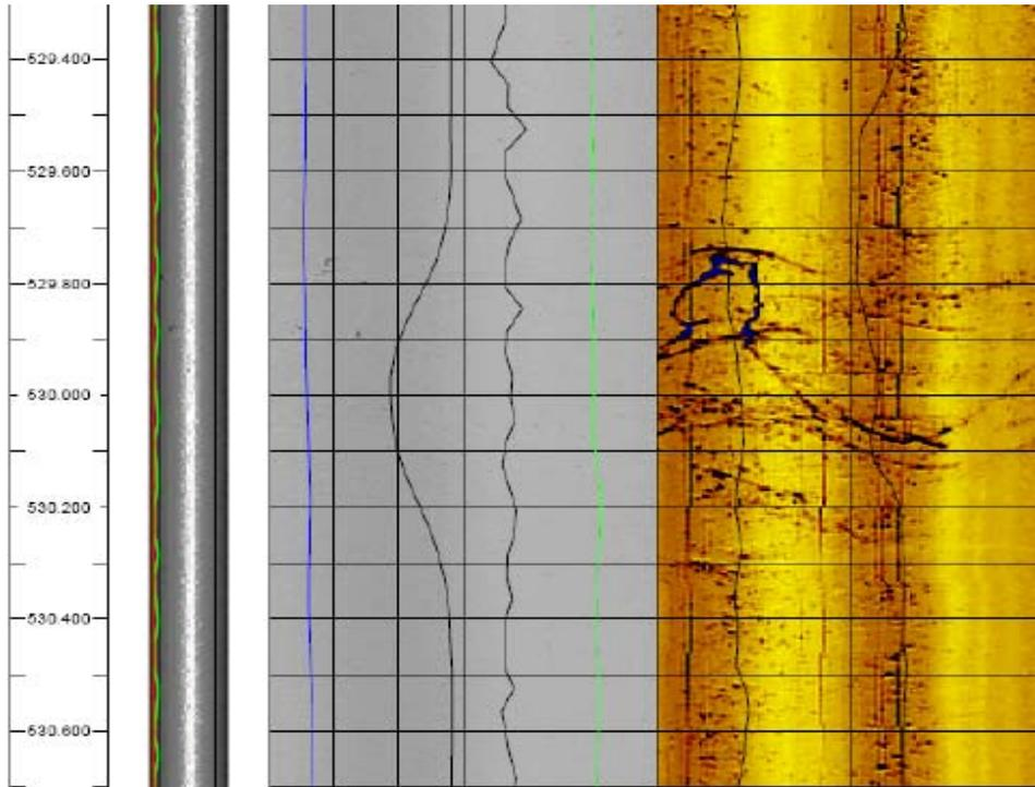
**Figure 27: A shallow/low borehole breakout identified between 529.3 – 530.7 mbl in borehole KFM02A. Note that the majority of borehole breakouts observed in the borehole are Shallow breakouts.**
