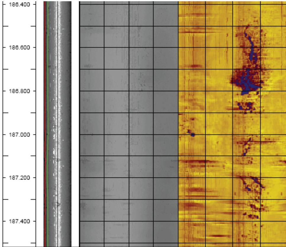
**Figure 22: Single borehole breakout identified at 186.4 – 187.5 mbl in boreholeKFM01B. The borehole breakout is only visible in the BHTV amplitude log and appears only on one side of the borehole (right)**
