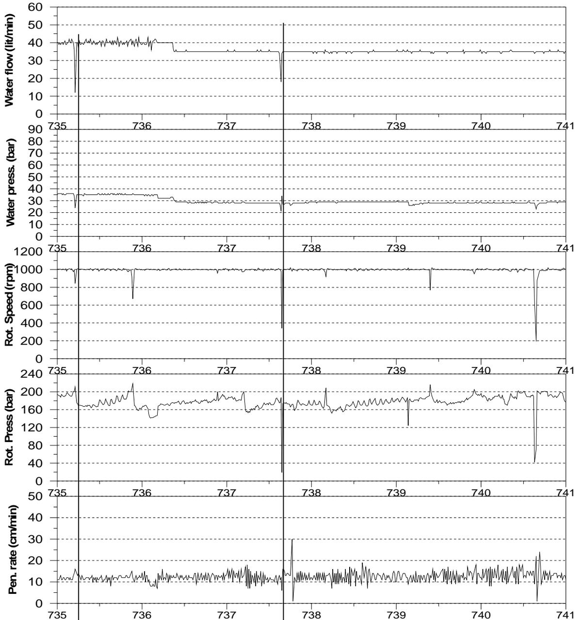
Figure 35: Correlated plot for the MWD parameters versus borehole length in a section (735 to 741 mbl) without borehole breakouts or major deformation zones.
