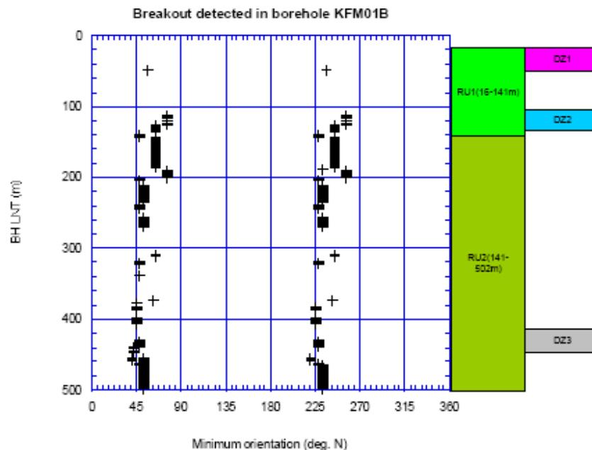
Figure 30: Correlation of borehole breakouts, to lithological rock units and deformation zones in borehole KFM01B.
