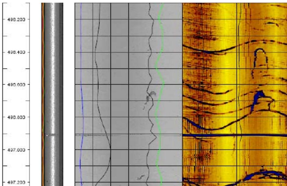
**Figure 26: A single borehole breakout identified at 496.1-497.2 mbl in borehole KFM02A. The borehole breakout was intercepted with several diagonal fractures and was only visible in the BHTV amplitude log.**
