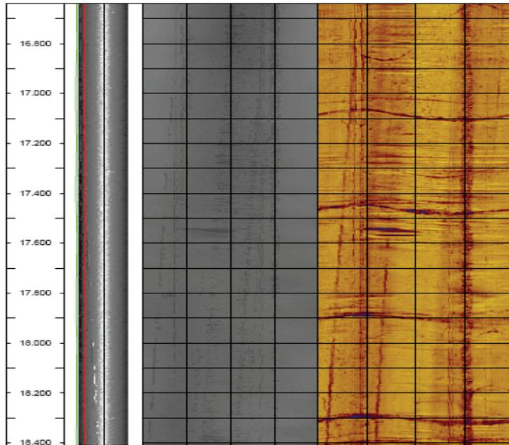
**Figure 15: A section (16.7-18.4 mbl) in borehole KFM01B with keyseat. The keyseat was visible in the BHTV amplitude log and has its azimuth from 264° - 284°N.**
