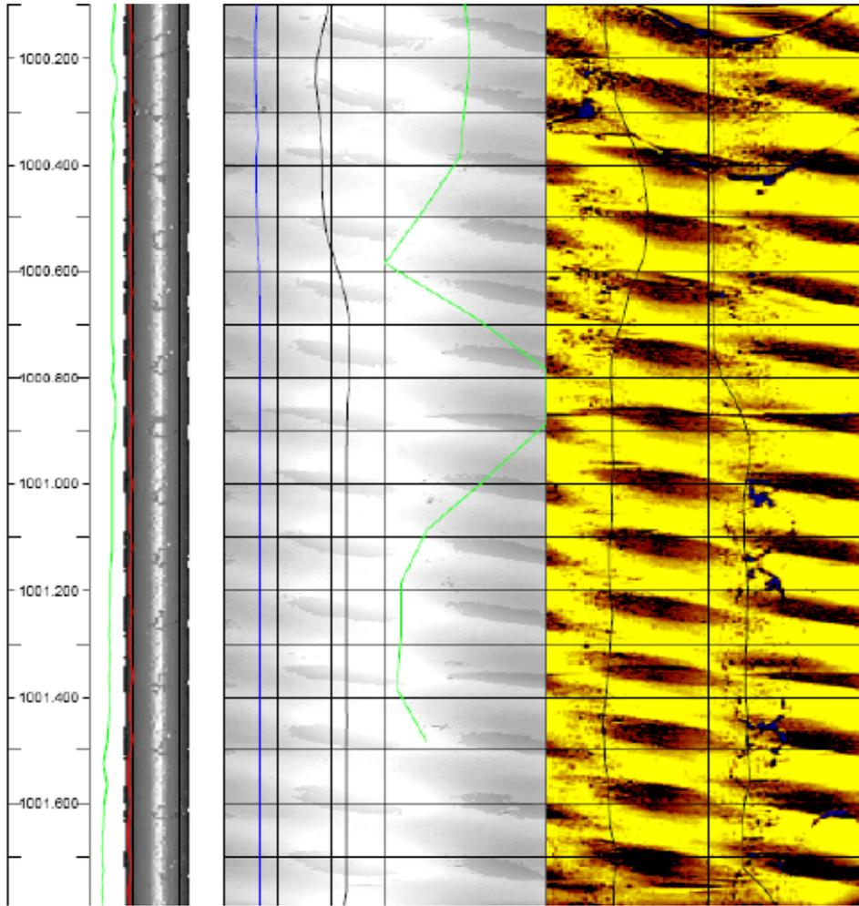
**Figure 29: Borehole breakout partially concealed by spiral grooves at 1000.1- 1001.8 mbl in borehole KFM02A.**
