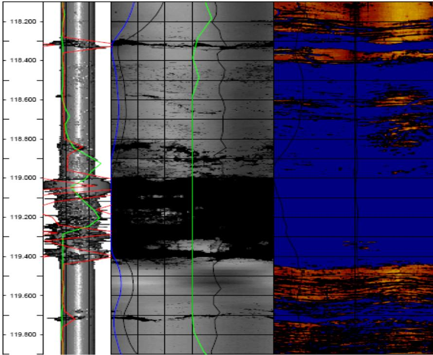
**Figure 18: A washout zone (118.1-119.9 mbl) in borehole KFM02A. This zone was clearly visible in three of the BHTV logs (Caliper 3D, travel-time and amplitude log).**
