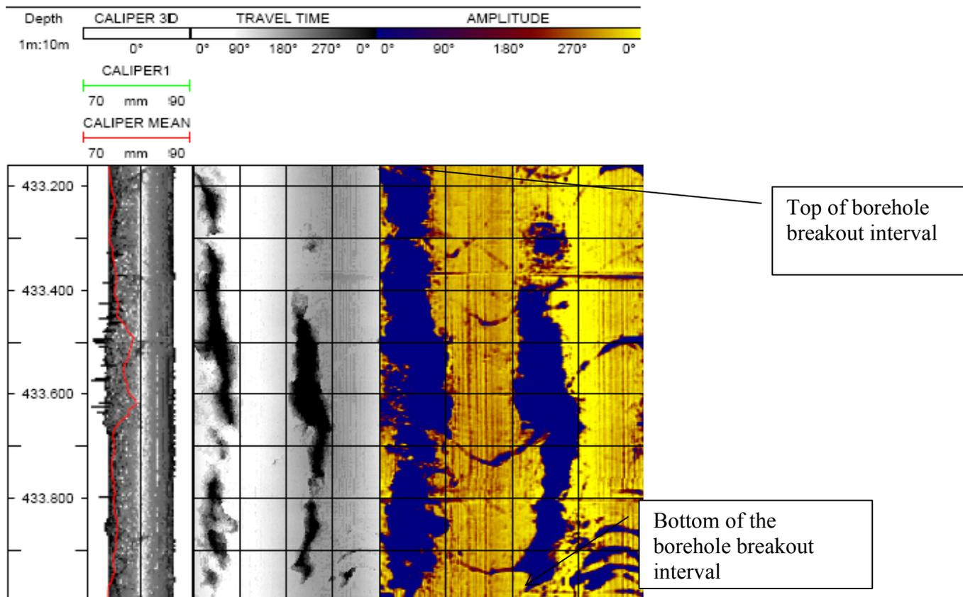
Figure 6: Example of diametrical borehole breakout identified in borehole KFM01B at the Forsmark site. Note that the figure indicated the top and the bottom of the borehole breakout.
