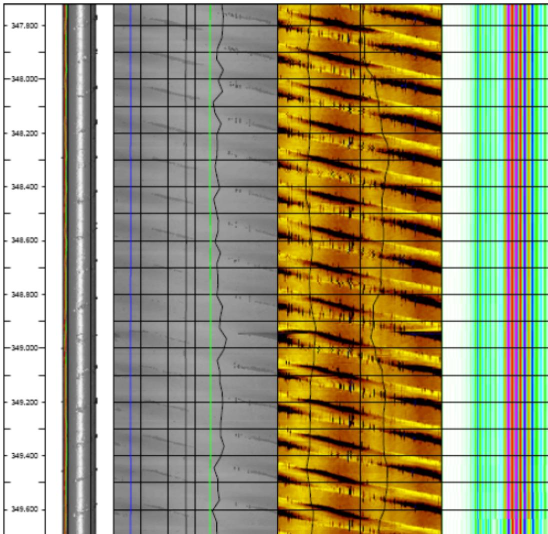
**Figure 14: Example of spiral grooves identified from 347.8 – 349.6 mbl in borehole KFM02A. Note that the spiral grooves is so thick that it was visible in three of the BHTV logs (i.e., caliper 3d, traveltime and amplitude log. But the severity was more in the amplitude log.**
