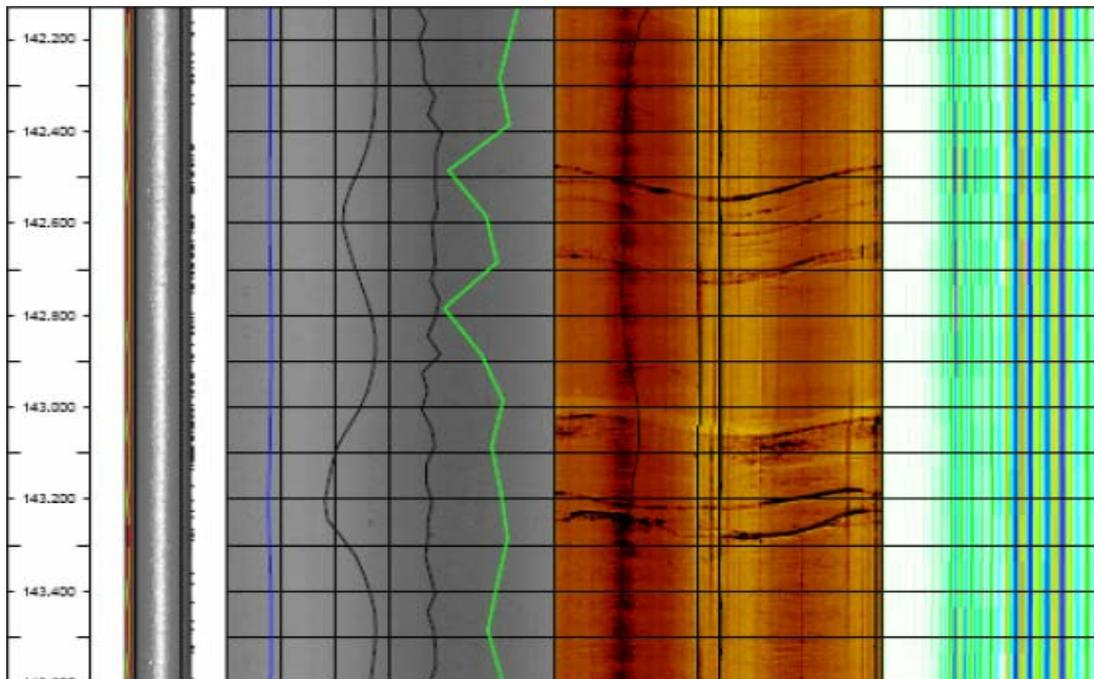
**Figure 16: One of the section in borehole (142.2-143.5 mbl) in KFM02A with keyseat. The keyseat was visible in the BHTV amplitude log and has an azimuth from 73-90°N.**
