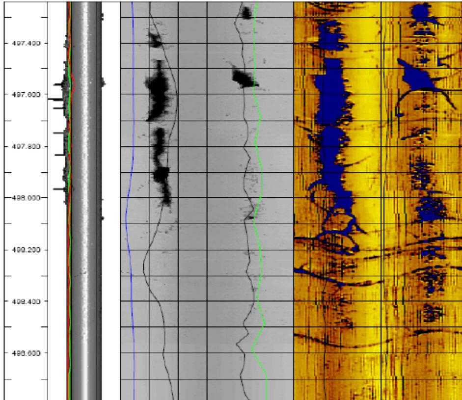
**Figure 25: Diametrical and deep borehole breakout identified at 497.2-498.1 mbl in borehole KFM02A. The borehole breakout was clearly observed in three of the BHTV logs.**
