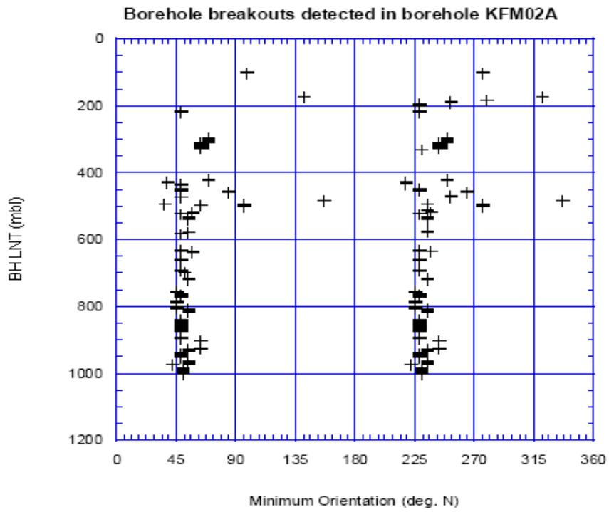
Figure 24: Downhole distribution of borehole breakouts versus depth in borehole KFM02A.
