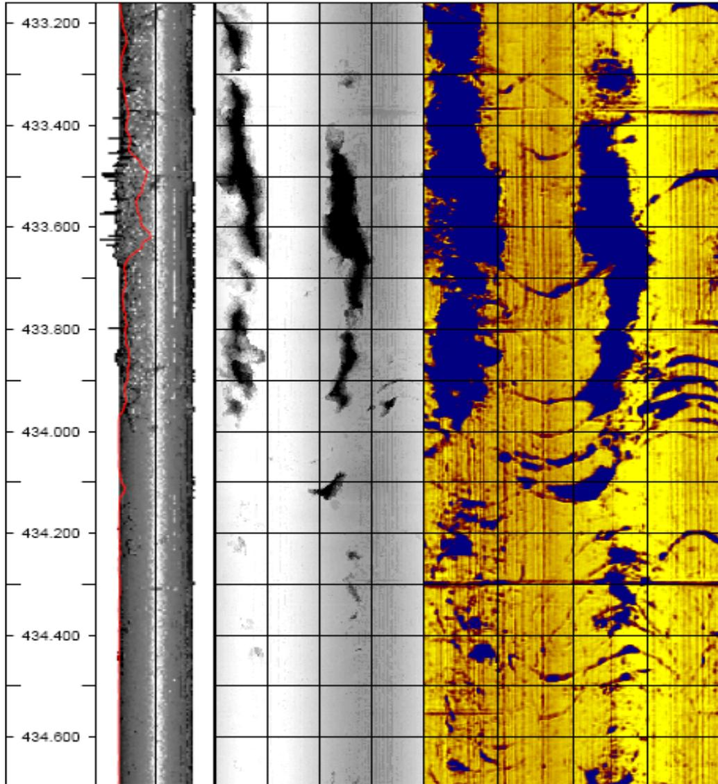
**Figure 21: Diametrical borehole breakouts identified from 433.2-434.7 mbl in borehole KFM01B. This is the most outstanding deep borehole breakout observed in the borehole. The borehole breakout is visible in three of the BHTV logs (caliper 3D, traveltime and amplitude log. Note that the breakout was intersected with several diagonal fractures.**
