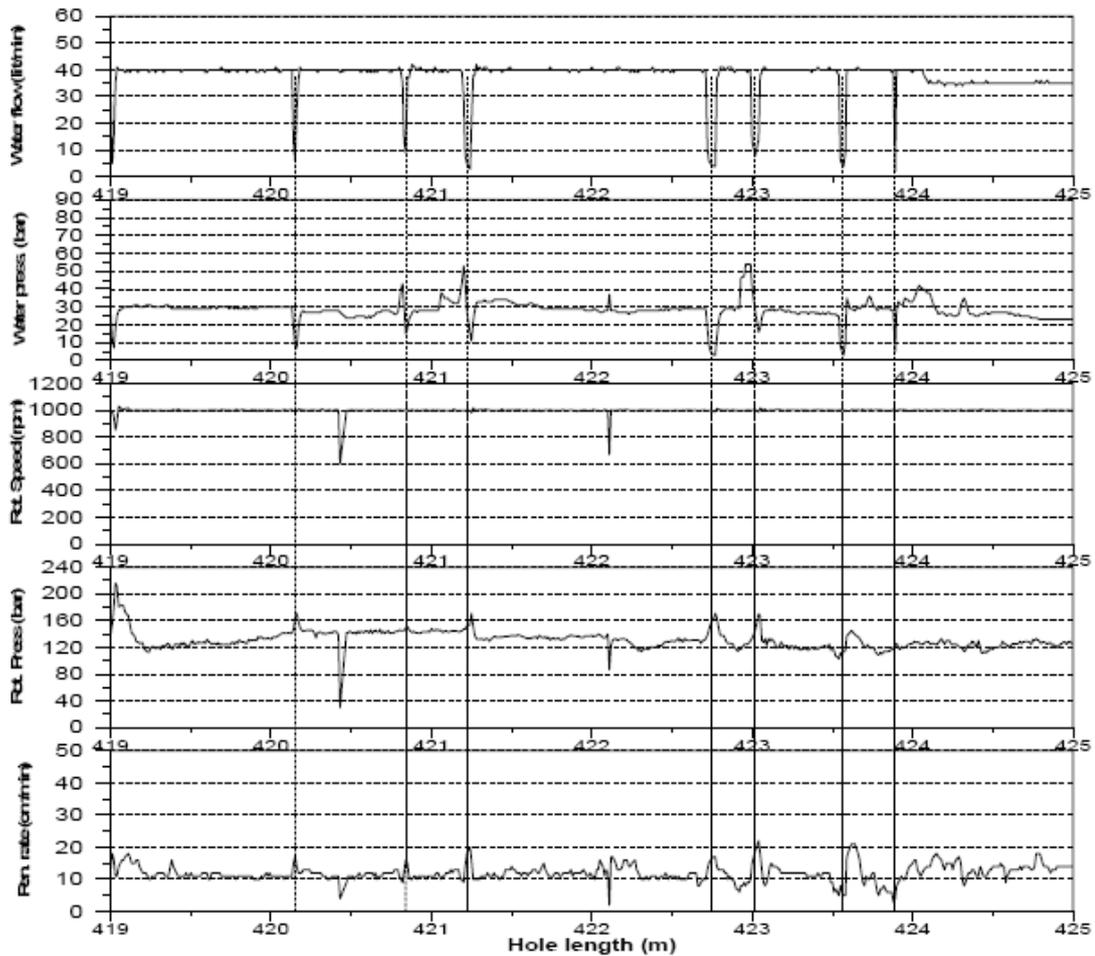
Figure 34: Correlated plot for the MWD parameters for section (419 to 425 mbl) in KFM02A with borehole breakout. Note that this section is mainly a rock unit (G3) and occurs across the major deformation zone DZ6.
