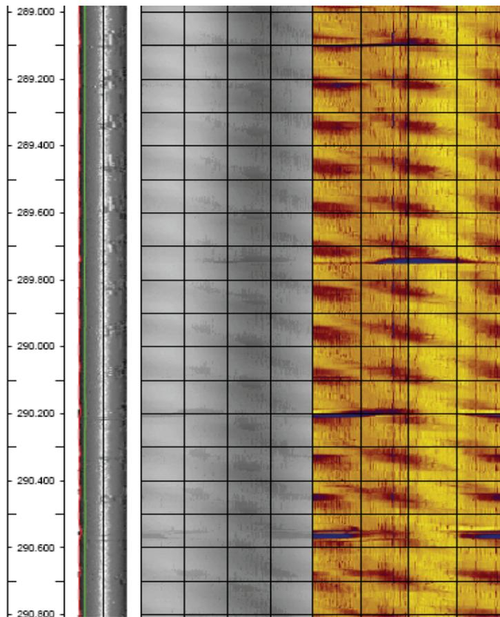
**Figure 12: A spiral grooves identified from 289.0-290.8 mbl) in borehole KFM01B. The spiral grooves are the dark diagonal bands that run across the BHTV log. The section with spiral grooves is more often visible in the BHTV amplitude log than in BIPS image.**
