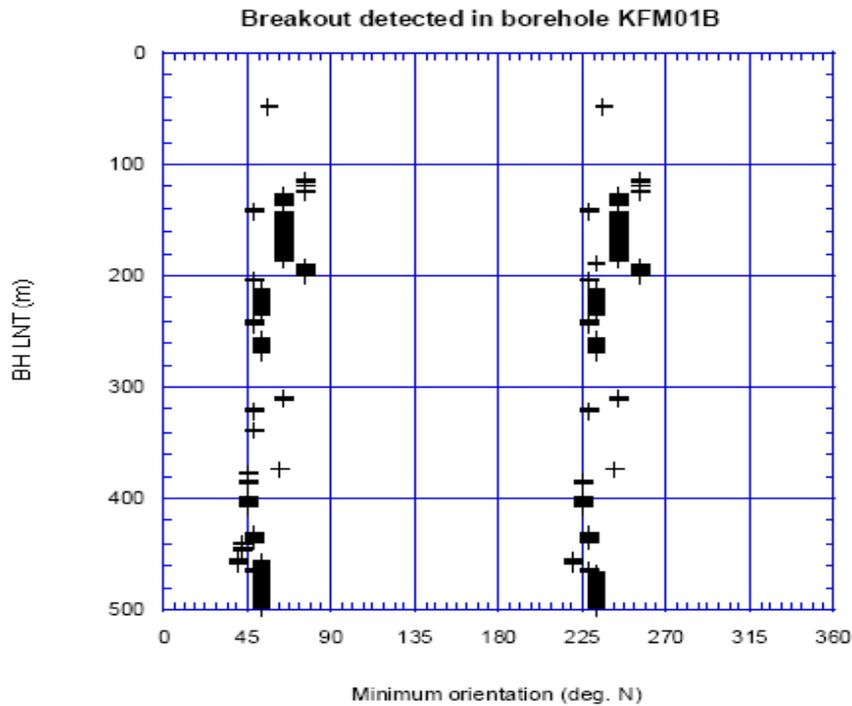
**Figure 20: Downhole distribution of borehole breakouts with depth in borehole KFM01B. Note that the borehole breakouts occurred more in abundant especially from 118 to 270 mbl and from 398 to 499 mbl. Note that minimum orientation (deg.N) is referring to orientation of the minimum horizontal stress (in degrees), whereas BH LNT is referring to borehole length (in meters)**
