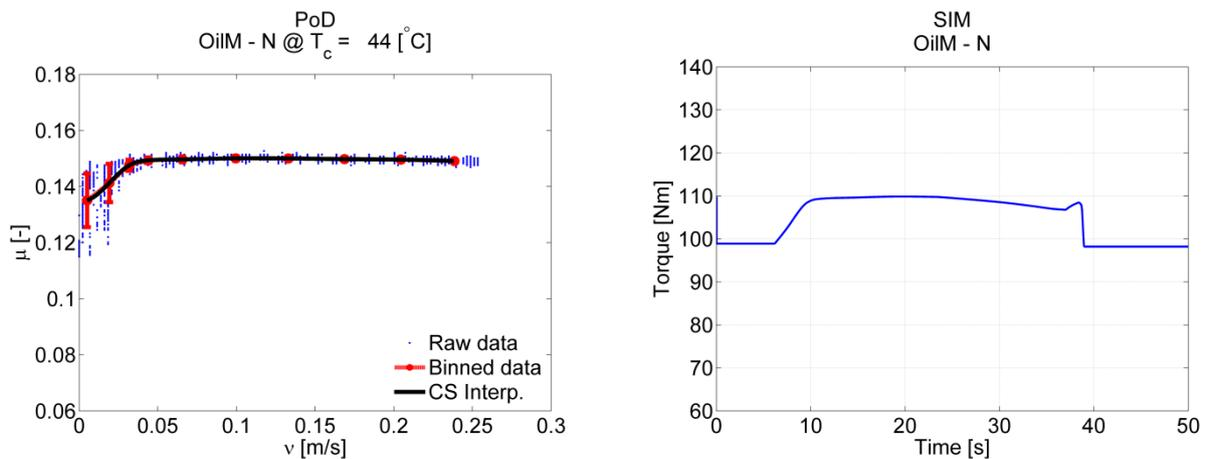
Figure 53. Low bin density gives a smoother  $\mu$ - $v$  curve and therefore also smoother predicted torque in the simulation.
