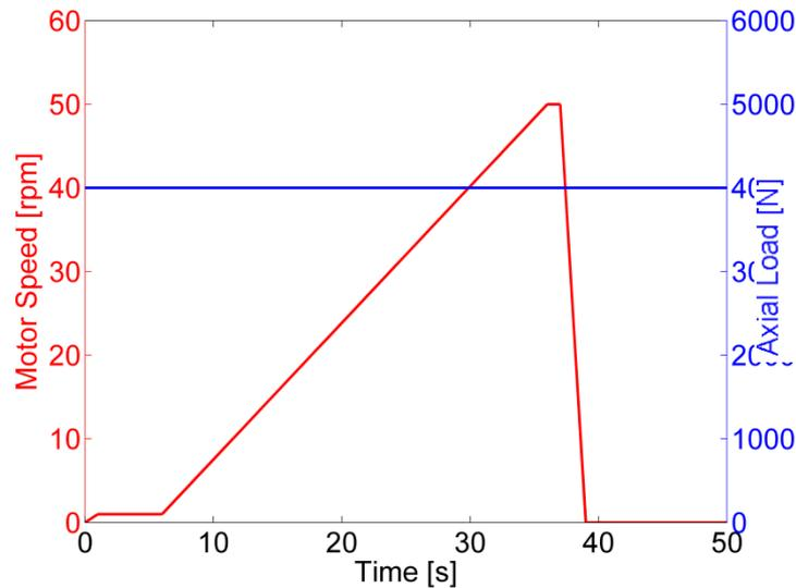
Figure 45. Controlled motor speed and applied axial load used in dynamic simulation.
