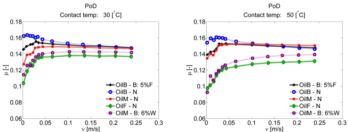
Figure 42. Friction versus sliding speed at a nominal contact temperature of 30 °C to the left, and 50 °C to the right, for the five different oil samples investigated in this range.
