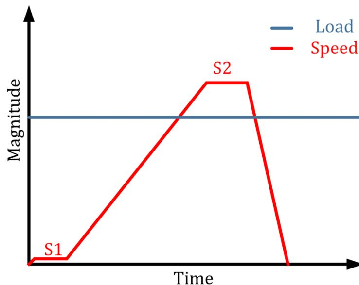
Figure 37. Test procedure for shudder limit in wet clutch test rig.
