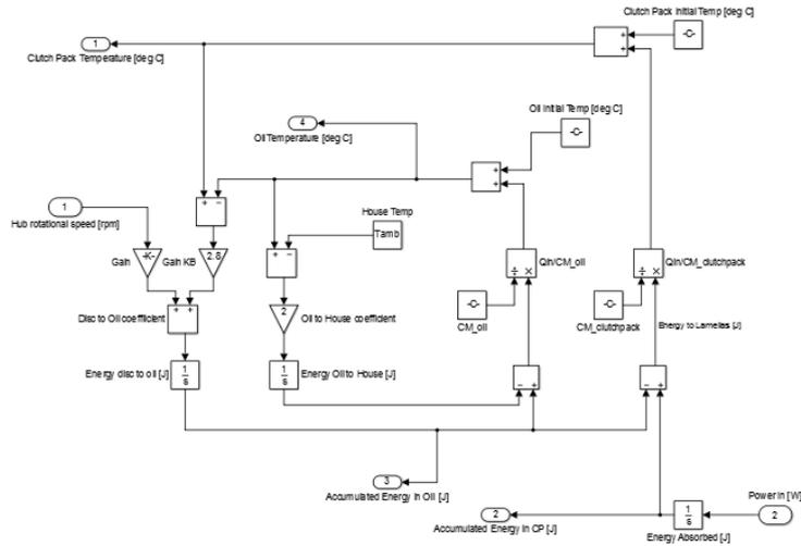
**Figure 35. Thermodynamic sub-system with three layers; clutch pack, oil supply, and housing.**
