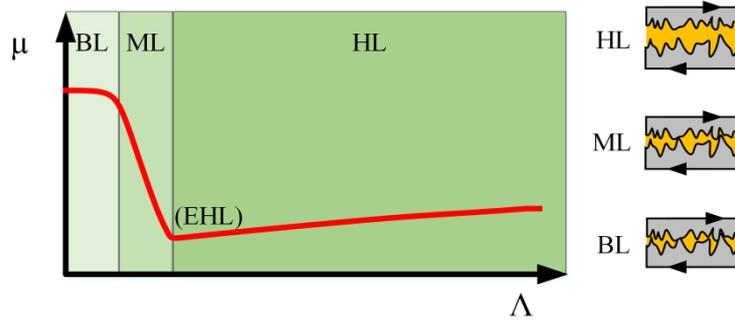
Figure 4. Schematic Stribeck curve showing the relation between surface separation ( $\Lambda$ ) and friction coefficient ( $\mu$ ) for lubricated contacts.
