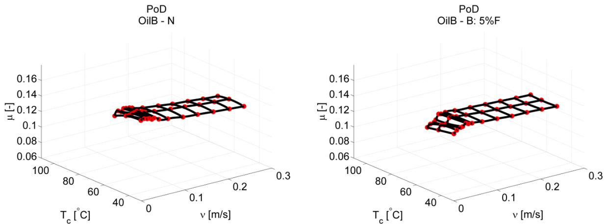
Figure 44. Friction versus sliding speed on the-x axis and contact temperature on the y-axis for fully OilB to the left and OilB blended with 5% OilF to the right, as measured in the pin-on-disc, with cubic spline interpolation between binned data points.
