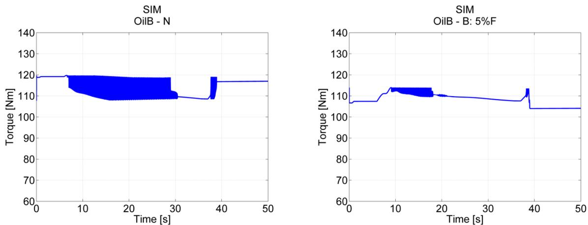
Figure 46. Torque predicted with dynamic simulation exhibiting severe shudder for OilB – N, and milder shudder for OilB blended with 5% OilF, both simulations at 30 °C initial contact temperature.
