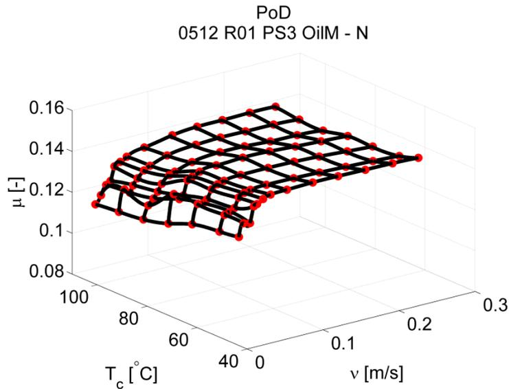
Figure 29. Lookup points in three dimensions, connected with cubic spline function.
