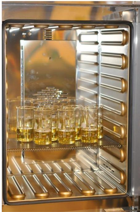
**Figure 38. Thermal ageing in Memert Laboratory oven at 120°C.**
