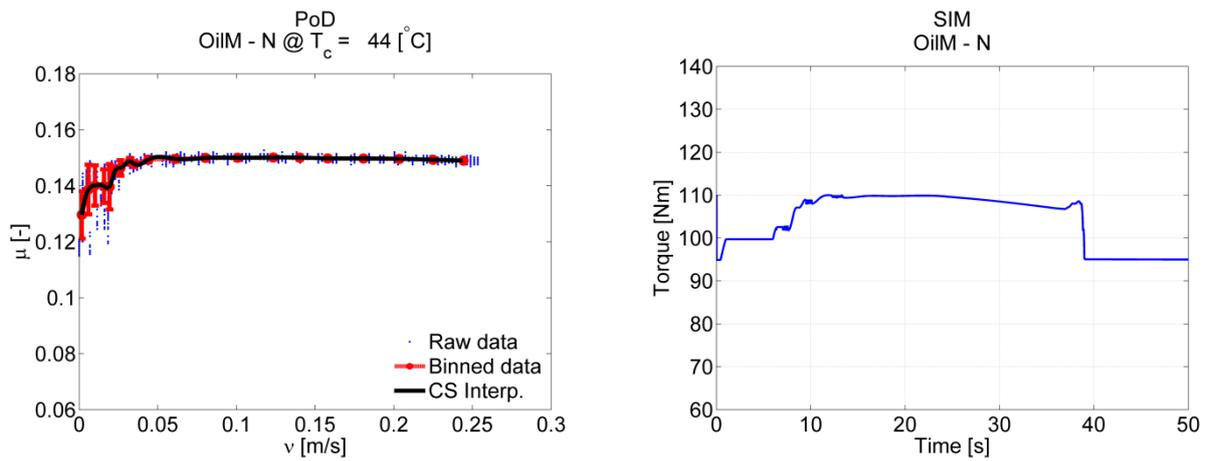
Figure 54. High bin density allows fluctuations to be represented in the  $\mu$ - $v$  curve which can affect the predicted torque in the simulation.
