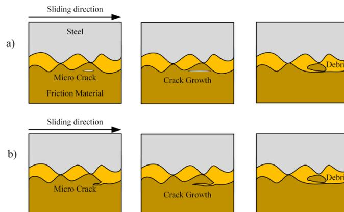
Figure 11. Schematics of delamination wear caused by either fatigue (a) or oil-wedge effect (b) reproduced from [18].
