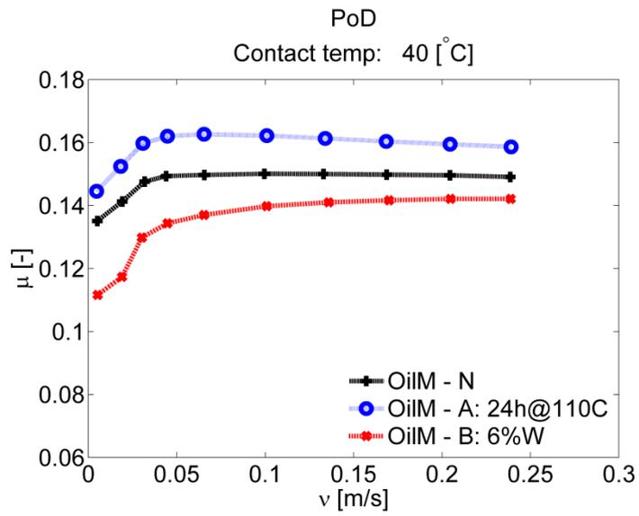
Figure 60. Friction versus sliding speed at a nominal contact temperature of 40 °C for one aged oil sample compared to the water degraded sample and a reference sample of OilM.
