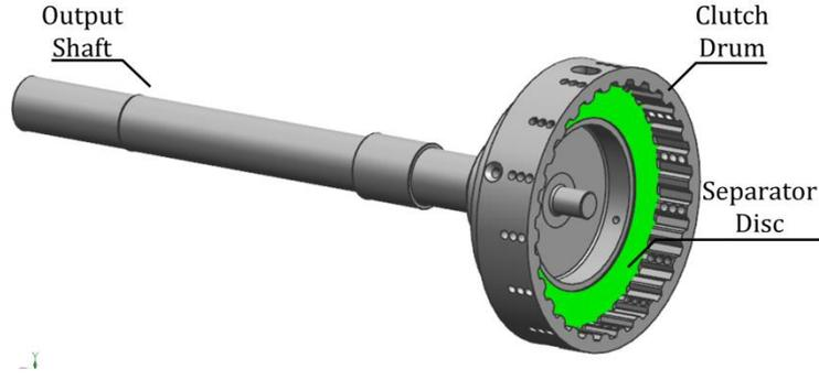
**Figure 32. Output shaft with a single separator disc in clutch drum.**
