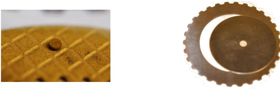
Figure 18. Friction and separator disc material. Pin on disc test pieces are cut out from the actual clutch discs.
