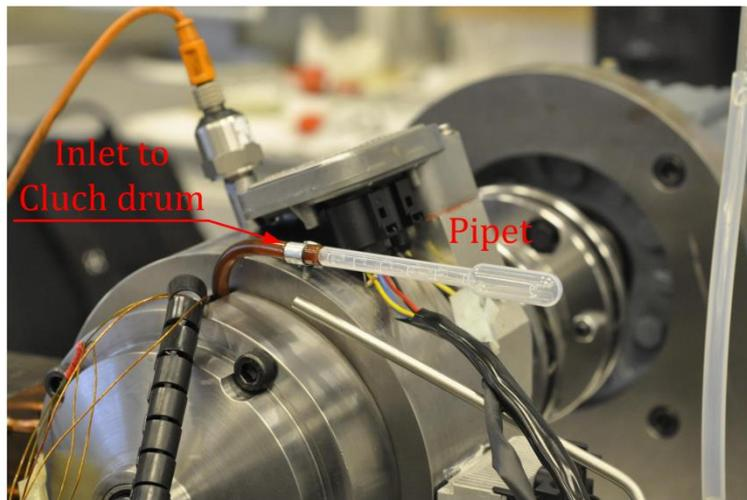
Figure 36. Injection of fully formulated oil into the clutch drum inlet.
