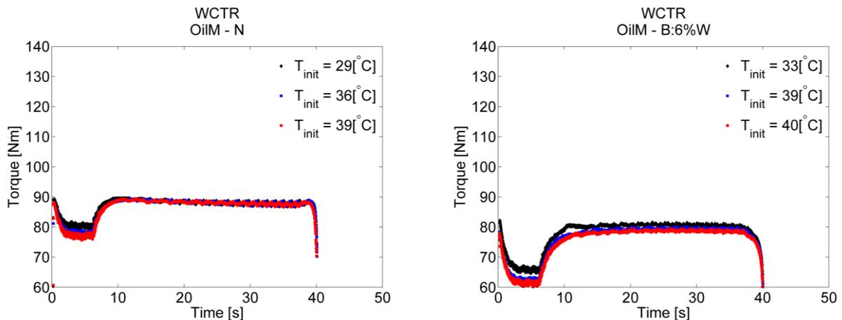
Figure 50. Measured torque in WCTR exhibiting no shudder for pure OilM to the left, and for OilM blended with 6% distilled water to the right.
