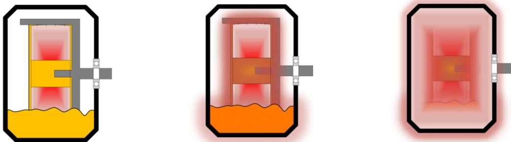
Figure 34. Illustration of the three layers in the thermodynamic sub-system, from left to right; heat generated in clutchpack is transferred to the oil, and finally to the constant temperature housing.
