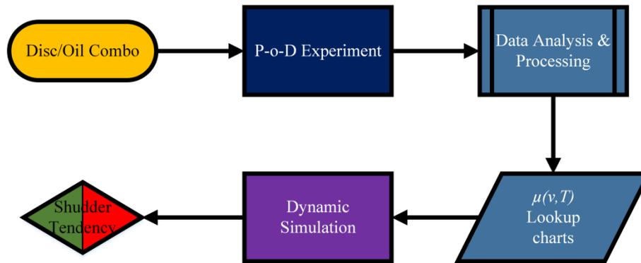
Figure 23. Friction assessment for shudder tendency evaluation routine.
