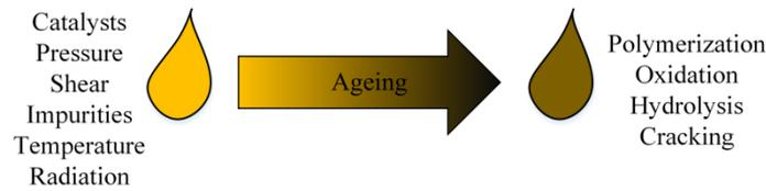
Figure 12. Various factors causing different types of degradation in oil [17].
