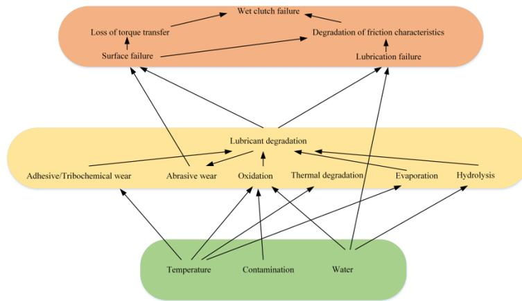
Figure 10. Factors leading to failures of wet clutches reproduced from [4].
