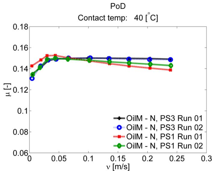
Figure 51. Friction versus sliding speed at a nominal contact temperature of 40 °C for four test runs with the same oil and materials, but different state of running in.
