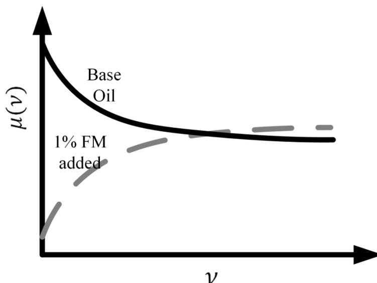
Figure 9. Schematic figure showing the dramatic effect on friction characteristics in a specific base oil for 1% treat rate of friction modifiers.
