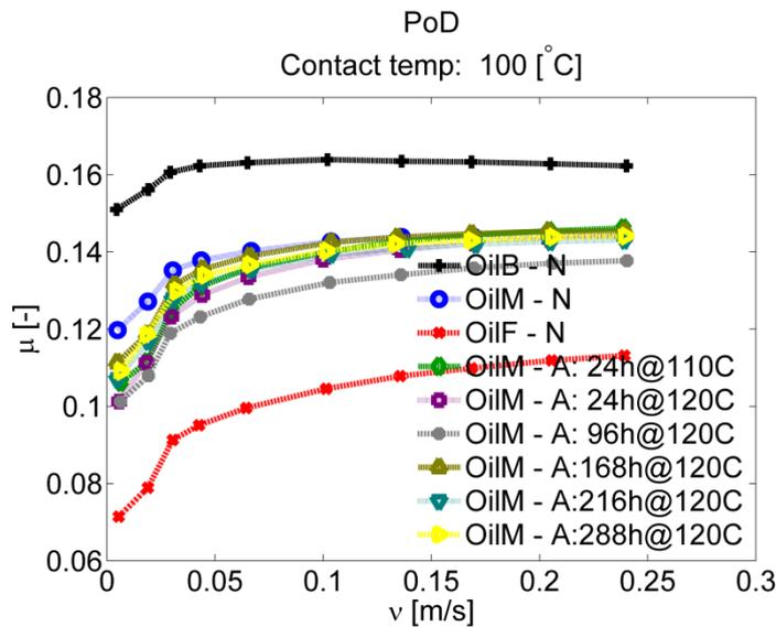
Figure 56. Friction versus sliding speed at a nominal contact temperature of 100 °C for the six aged oil samples compared to the three reference samples.
