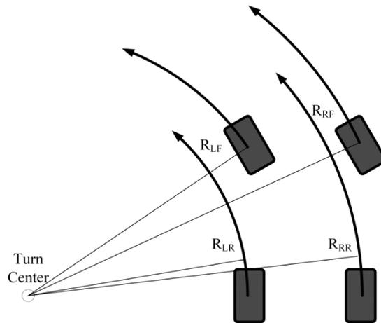
Figure 1. Wheels must rotate at different speeds when turning, due to individual arc length for each wheel when turning.
