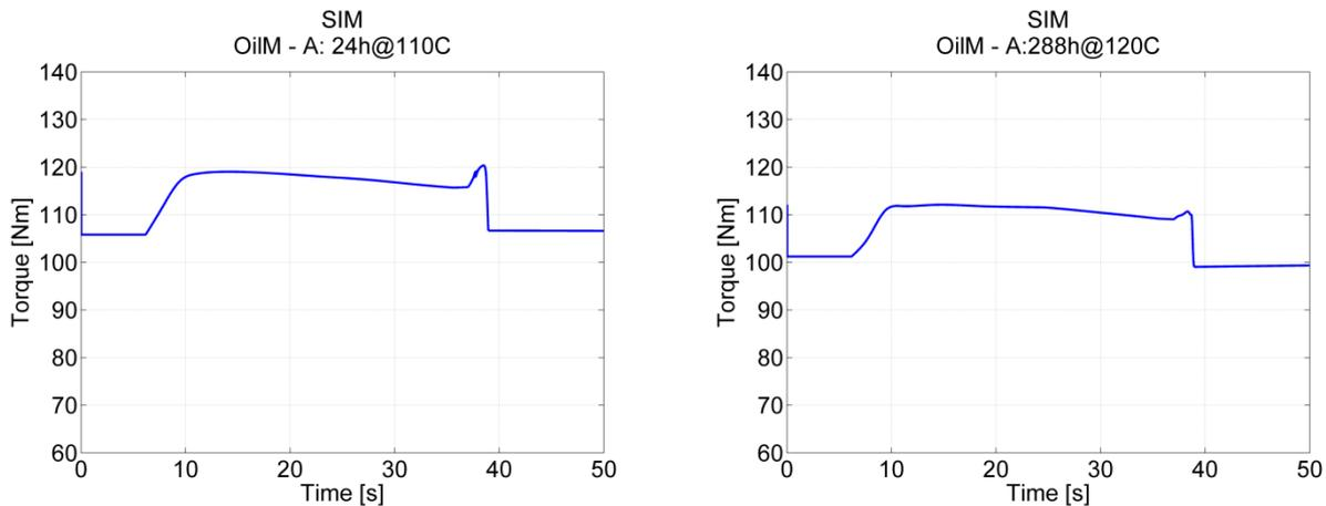
Figure 57. Torque predicted with dynamic simulation exhibiting minimal tendency of shudder at 38s for OilM aged for 24h at 110°C to the left, and no tendency for OilM aged for 288h at 120°C to the right, both simulations at 40 °C initial contact temperature.
