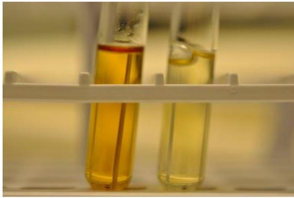
**Figure 58. Color shifting in OilF, aged 168h at 120 °C to the left compared to fresh oil sample to the right.**
