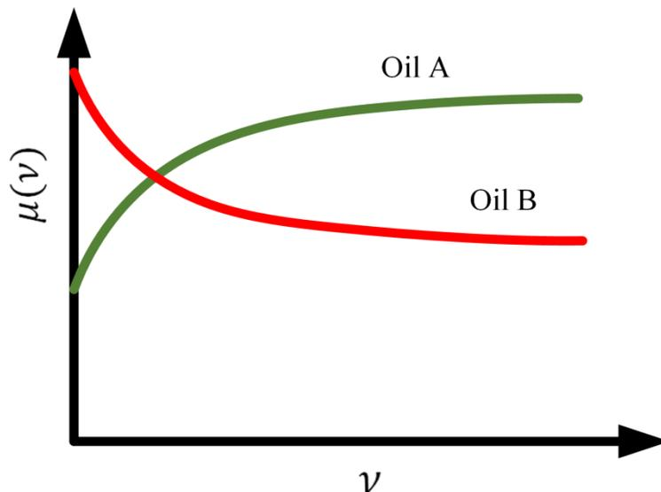
Figure 8. Schematic figure showing difference in friction characteristics for different oils in a wet clutch.
