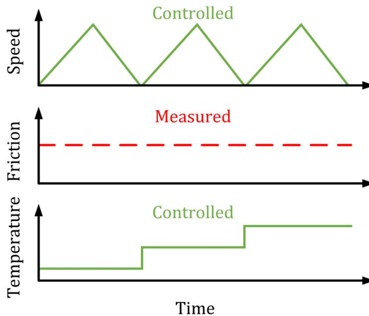
**Figure 24. Principle of test procedure to determine friction characteristics over full operational range in pin on disc.**
