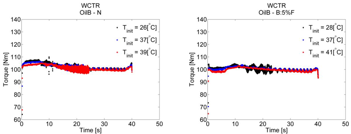
Figure 49. Measured torque in WCTR exhibiting shudder for OilB - N for three consecutive speed ramps, and for the first speed ramp with low initial temperature when using OilB blended with 5% OilF.
