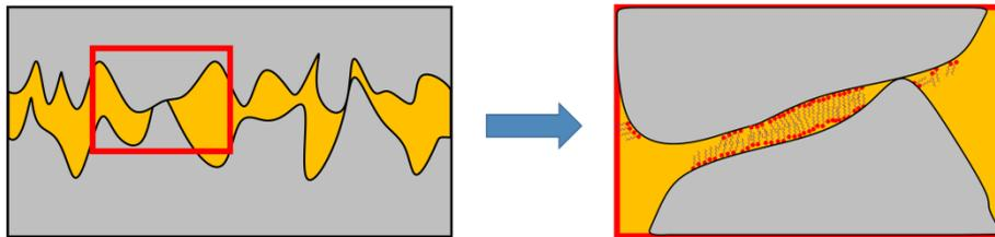
Figure 5. Schematic monomolecular layer adhered to metal surfaces preventing metal to metal contact.
