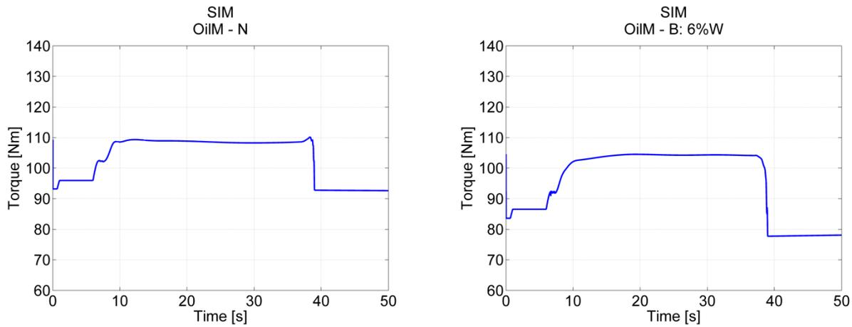
Figure 47. Torque predicted with dynamic simulation exhibiting no tendency of shudder for neither OilM – N to the left, nor OilM blended with 6% distilled water to the right, both simulations at 30 °C initial contact temperature.
