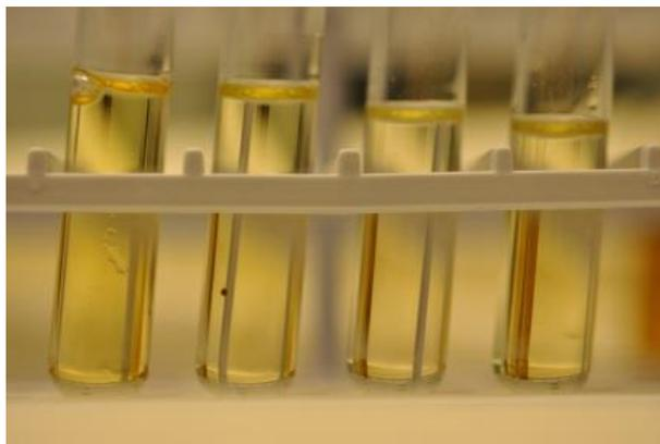
**Figure 59. Minimal color shifting in OilM, from left to right, aged 288h, 168h, 24h and 0h at 120 °C.**
