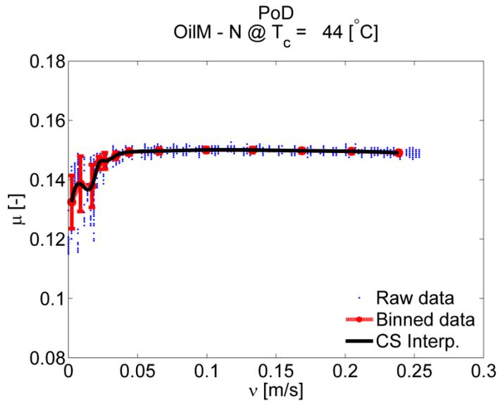
Figure 28. Raw data points grouped in Bins which can be interpolated with Cubic spline function to produce continuous curve.
