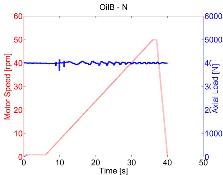
Figure 48. Motor speed and applied load in the wet clutch test rig during experiment with OilB - N.
