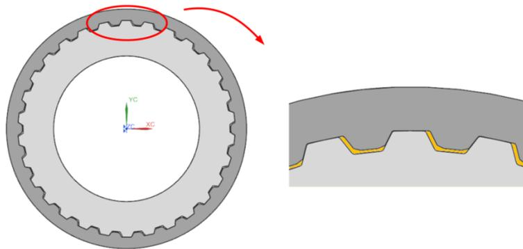
**Figure 62. Gap in spline coupling which cause backlash.**
