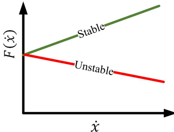
Figure 17. Schematic diagram showing the effect of sliding speed dependent friction force on the stability of a dynamic system.
