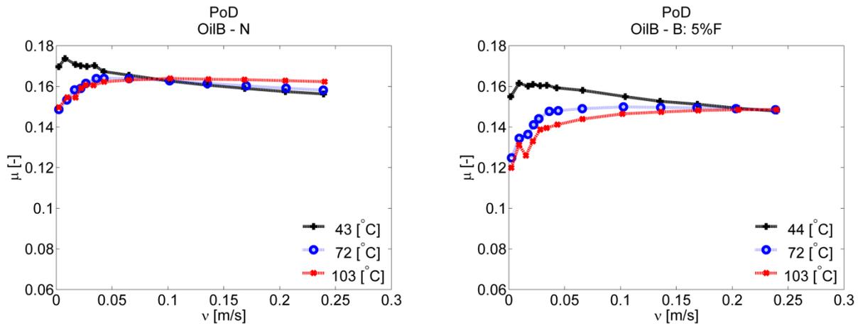
Figure 39. Friction versus sliding speed at three different temperature levels for pure OilB to the left and OilB blended with 5 % fully formulated oil (OilF) to the right.
