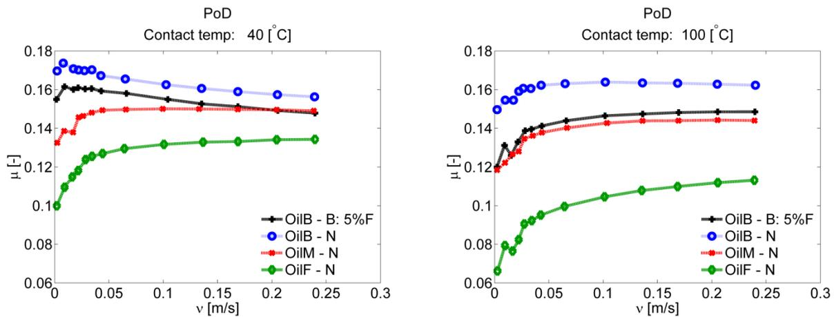
Figure 41. Friction versus sliding speed at a nominal contact temperature of 40 °C to the left, and 100 °C to the right, for the four different oil samples investigated in this range.
