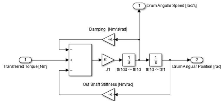
Figure 33. 1-DOF dynamic motion sub-system of WCTR.
