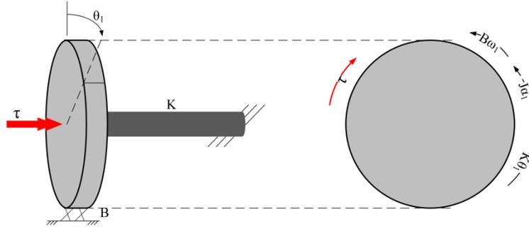
Figure 15. Simple 1-DOF rotational mechanical system, with free body diagram to the right.
