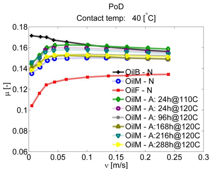
Figure 55. Friction versus sliding speed at a nominal contact temperature of 40 °C for the six aged oil samples compared to the three reference samples.
