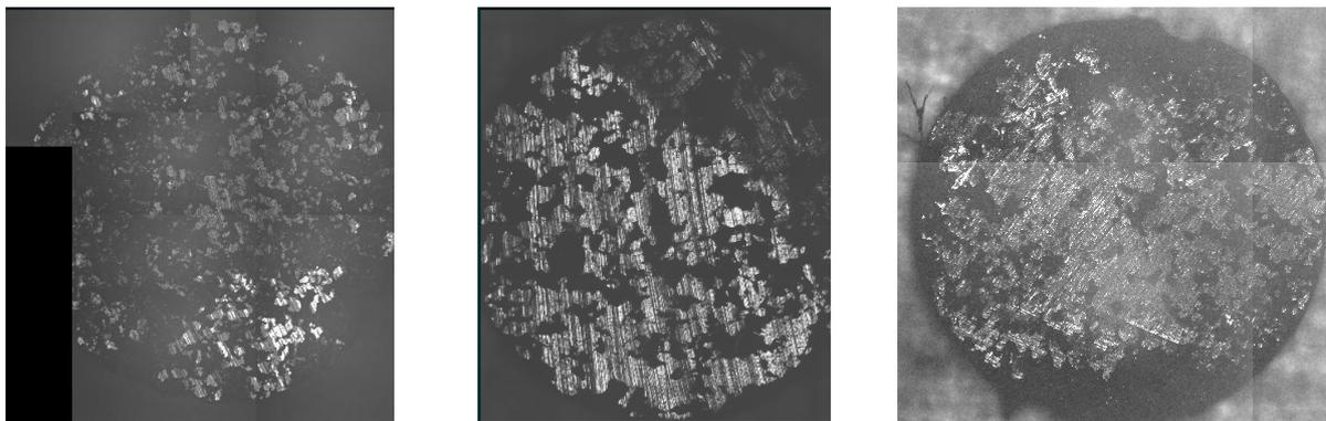
Figure 52. Different states of PS, from left to right, PS2 without run in showing a very small contact area, compared to PS1 and PS3 with approximately 75% of the nominal area being in contact.
