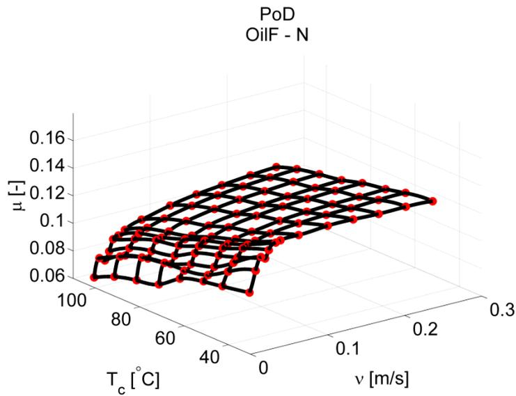
Figure 43. Friction versus sliding speed on the-x axis and contact temperature on the y-axis for fully formulated oil as measured in the pin-on-disc, with cubic spline interpolation between binned data points.
