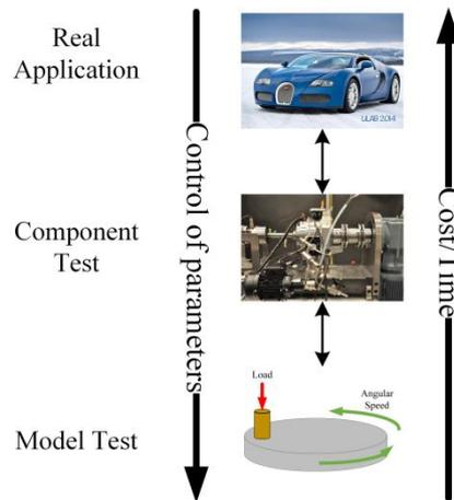
Figure 3. Three broad categories of test methods for wet clutch evaluation.
