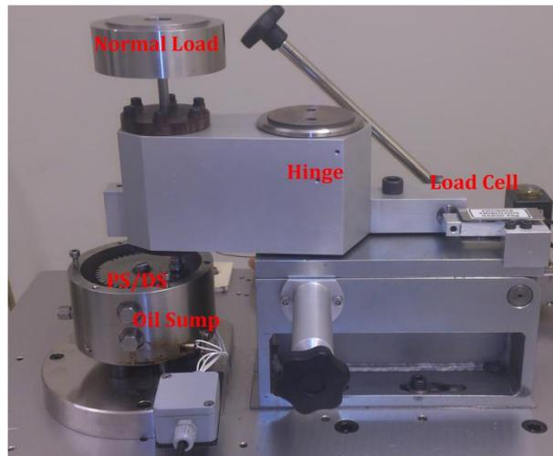
Figure 19. Phoenix Tribology TE67 pin-on-disc test rig.
