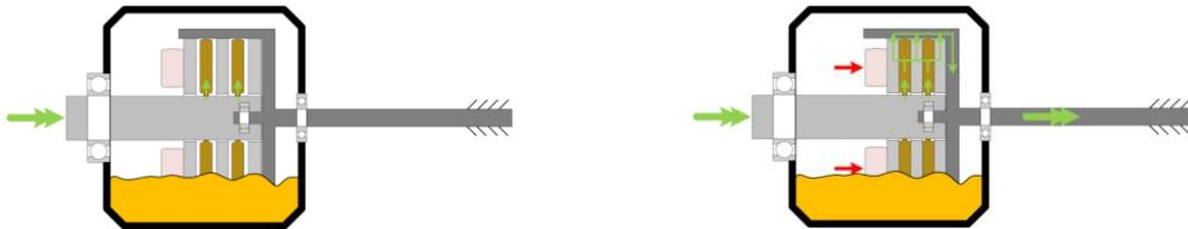
Figure 22. Component test rig schematics; open clutch to the left, closed to the right.
