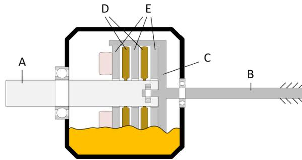
Figure 2. Schematics of important components in a wet clutch.
