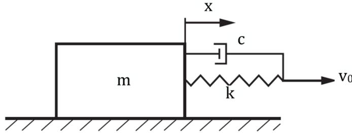
Figure 16. Block pulled over surface by spring and damper.
