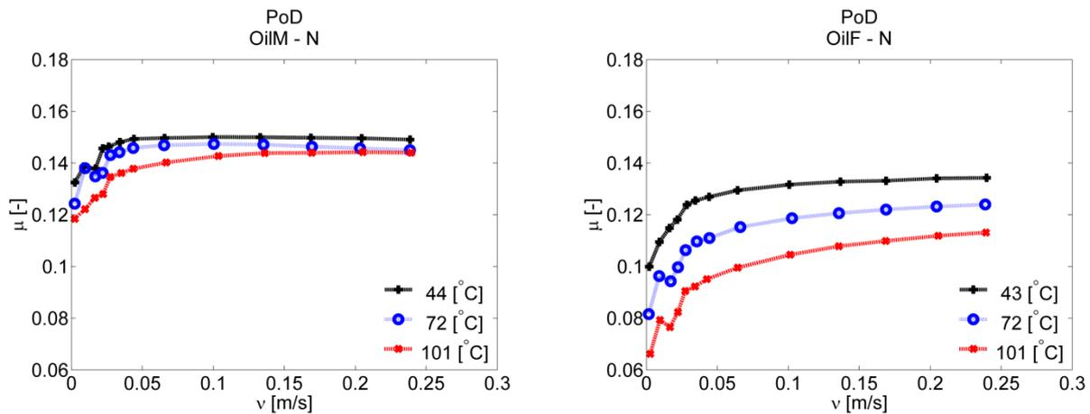
Figure 40. Friction versus sliding speed at three different temperature levels for pure model oil to the left and fully formulated oil to the right.
