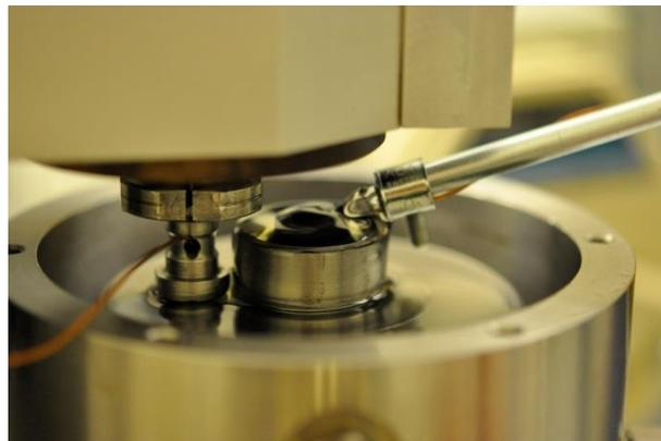
Figure 20. Oil pumped into oil dispenser located at the center of the disc. Temperature measured in contact and oil outlet.
