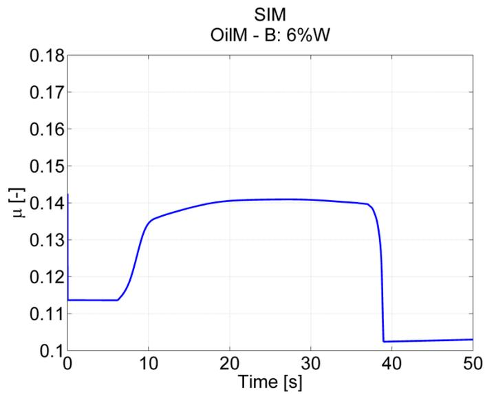
Figure 61. Torque predicted with dynamic simulation exhibiting a very smooth torque transfer for OilM blended with 6% distilled water, simulated with 40 °C initial contact temperature.
