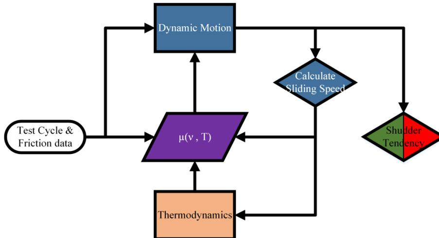
Figure 30. Dynamic simulation consisting of three major subsystems; motion, thermal and friction functions.
