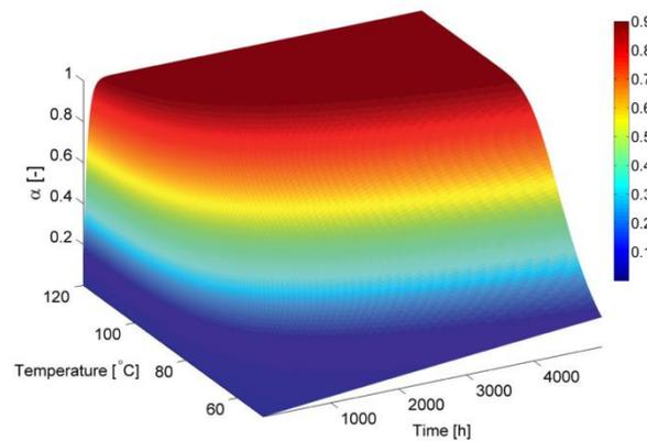
Figure 14. Effect of oil ageing on the parameter alpha, with alpha = 1 corresponding to depleted additives causing increased friction [4].
