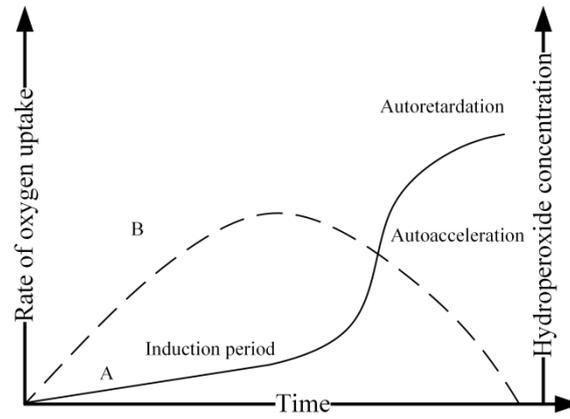
Figure 13. Termination of the oxidation occurs when the hydroperoxide concentration is low. A is the rate of oxygen uptake and B is hydroperoxide concentration. Reproduced from [13].
