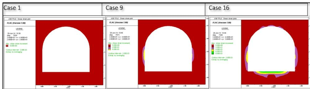
**Figure 10:** Shear strain plot for cases 1, 9 and 16 of the PEM model
