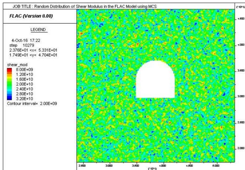
Figure 6: Random distribution of shear modulus in a MCS model
