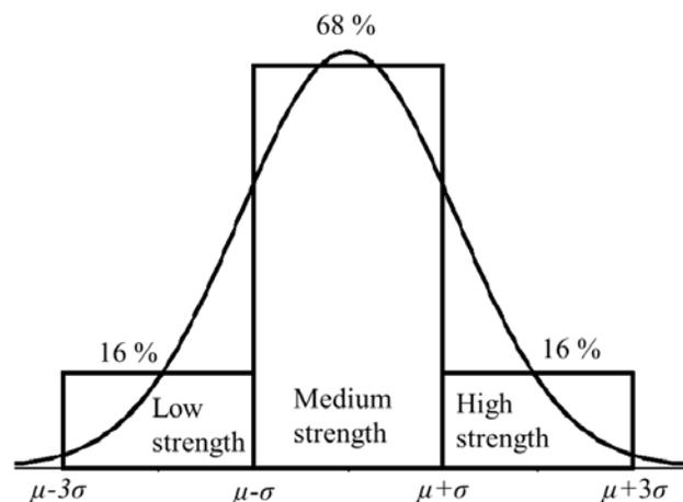
**Figure 7:** Interval for each class of the random input parameters and their corresponding probabilities
