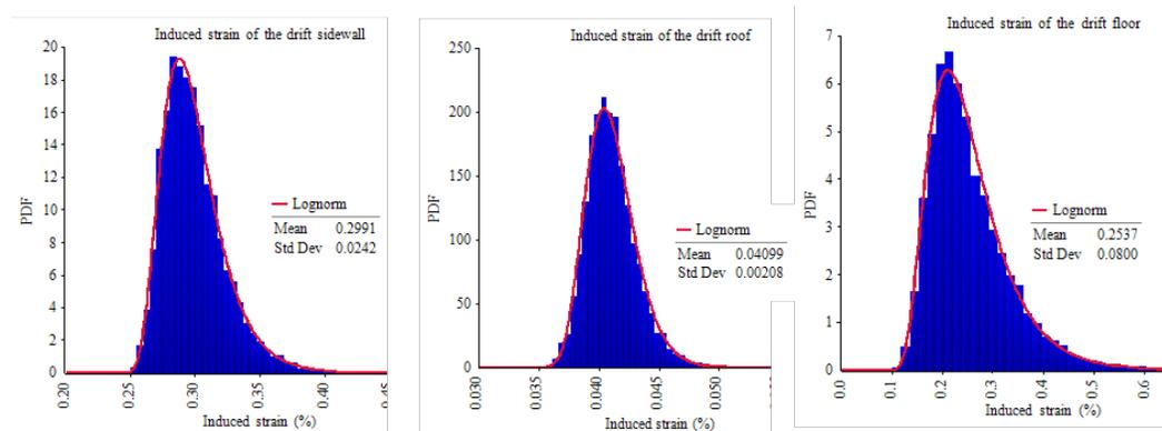
Figure 7: PDFs of induced strain of the drift sidewall, roof and floor for MCS Model
