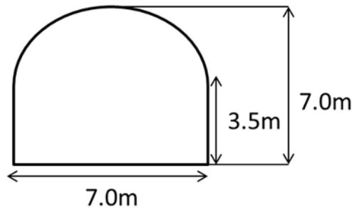
**Figure 2:** Geometry of the drift
