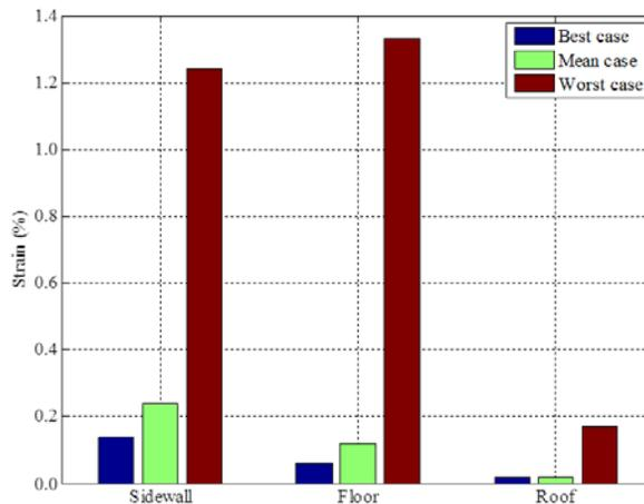
**Figure 5:** Strains around the drift for the best, mean and worst case models
