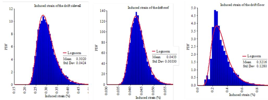
**Figure 8:** Assessed PDFs of induced strain of the drift sidewall, roof and floor for SCM Model
