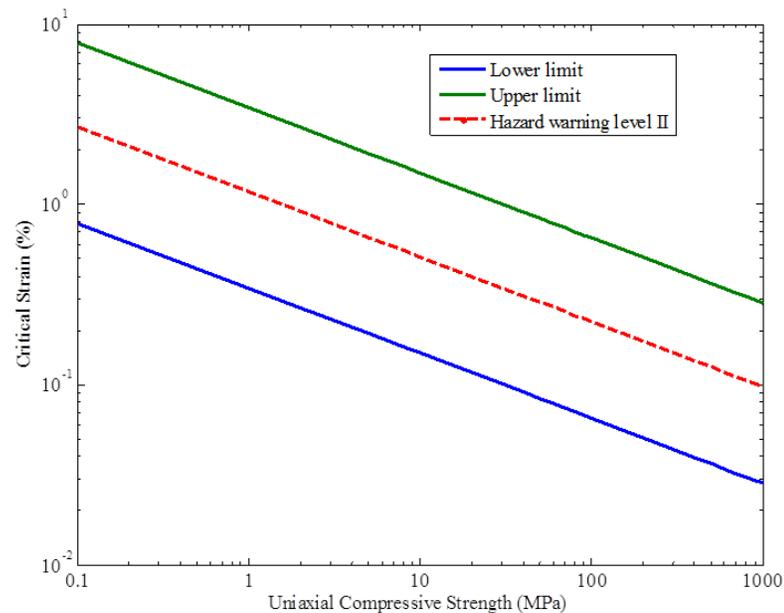
**Figure 3:** Sakurai's relationship between critical strain and UCS, also indicating hazard warning level II for assessing stability of tunnels (adapted from [49, 50])
