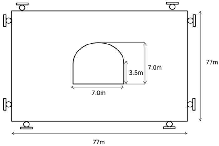
**Figure 4:** FLAC model size for the simulations
