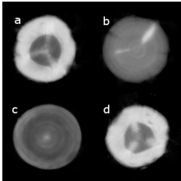
**Figure 1:** Four examples of cross-section CT images where a) is the Douglas-fir log of data set 1, b) is the white spruce log of data set 1, c) is the western redcedar log of data set 2, and d) is the Douglas-fir log of data set 2.
