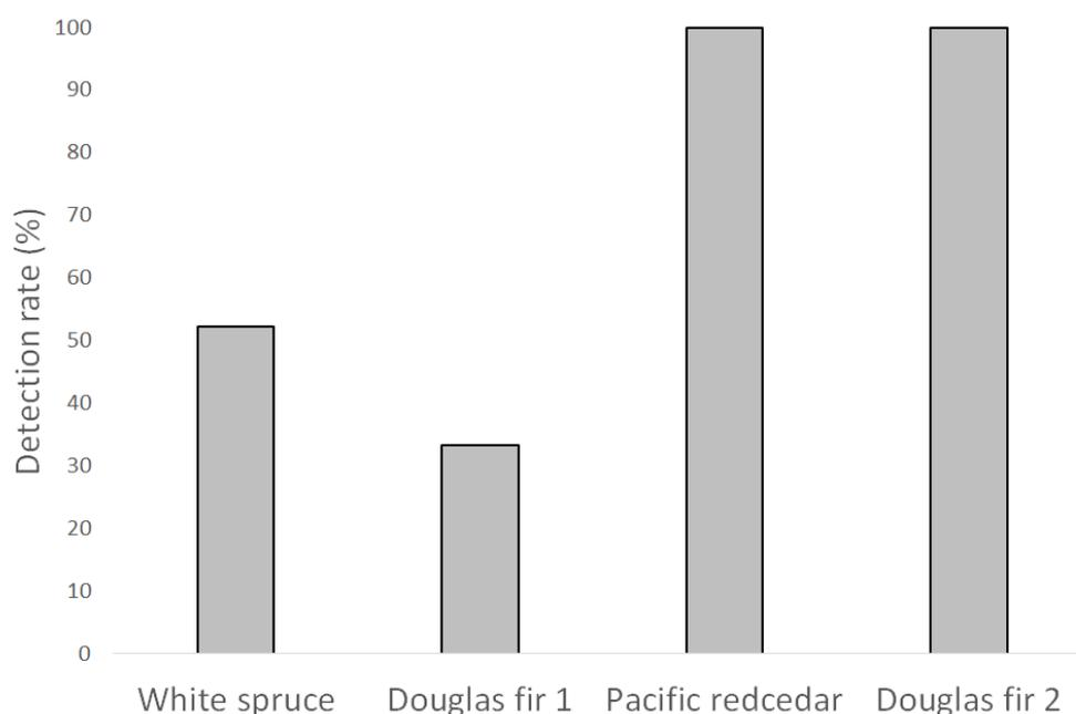
**Figure 2:** Knot detection rate for the four logs.
