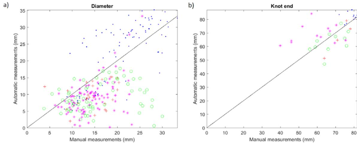
**Figure 3:** Automatic and manual measurements of knot diameter (a), and knot end position (b). Each point in (a) corresponds to one measurement of a knot in a concentric surface, while each point in (b) corresponds to one single knot. Magenta stars = white spruce, red plus signs = Douglas-fir 1, blue points = western redcedar, and green circles = Douglas-fir 2.
