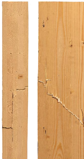
Figure 15: Shearing failure in CLT ±45°, top and side view
