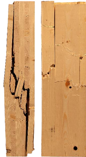
Figure 13: Compression sample, crushing and splitting failure in CLT 90°, sample top and side view
