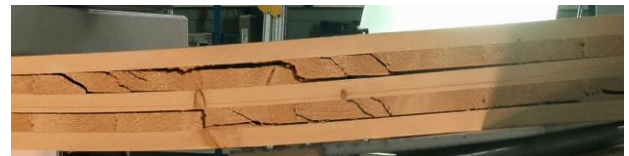
Figure 9: Failure caused by initial rolling shear near to bondlines appeared as shear stress transverse to the grain
