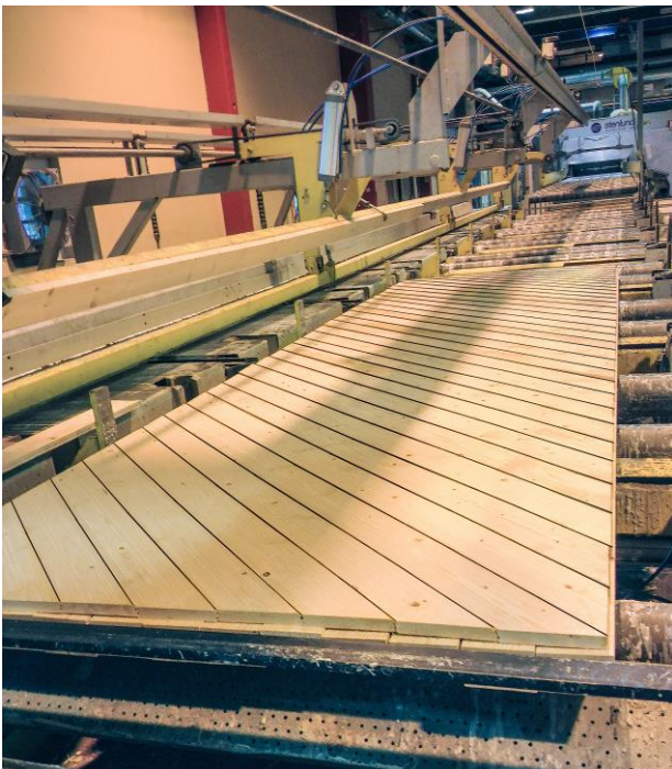
Figure 4: Industrial production line used for manufacturing conventional CLT 90° and modified CLT ±45° panels
