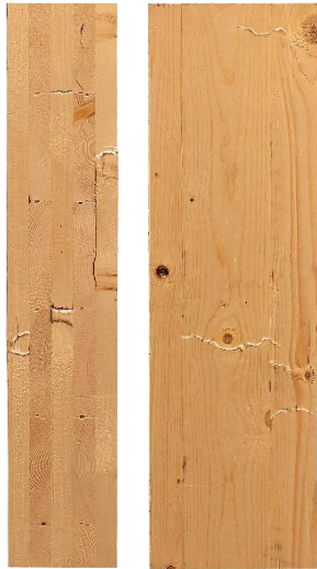
Figure 14: Failure due to crushing in CLT 90°, top and side view
