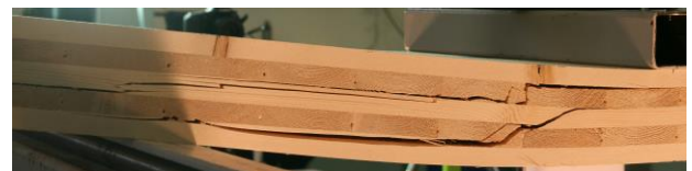
Figure 11: Failure due to a combination of longitudinal shear and initial rolling shear near to the bondlines
