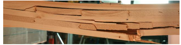
Figure 8: Bending failure due to tension in the lowest outer layer
