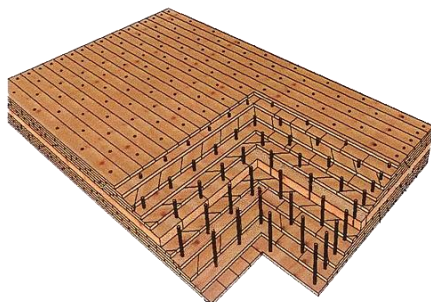
Figure 2: Thoma Holz100 uses wooden dowels to assemble boards in orientations of \pm 45^\circ [9]
