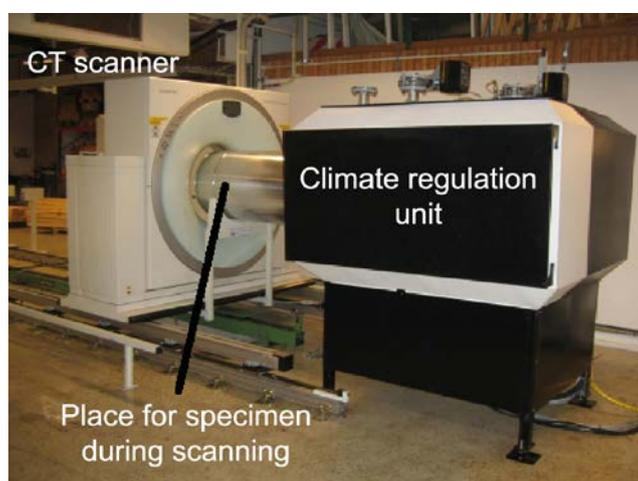
**Figure 1:** X-ray computed tomography (CT) with the climate chamber installed for CT measurements
