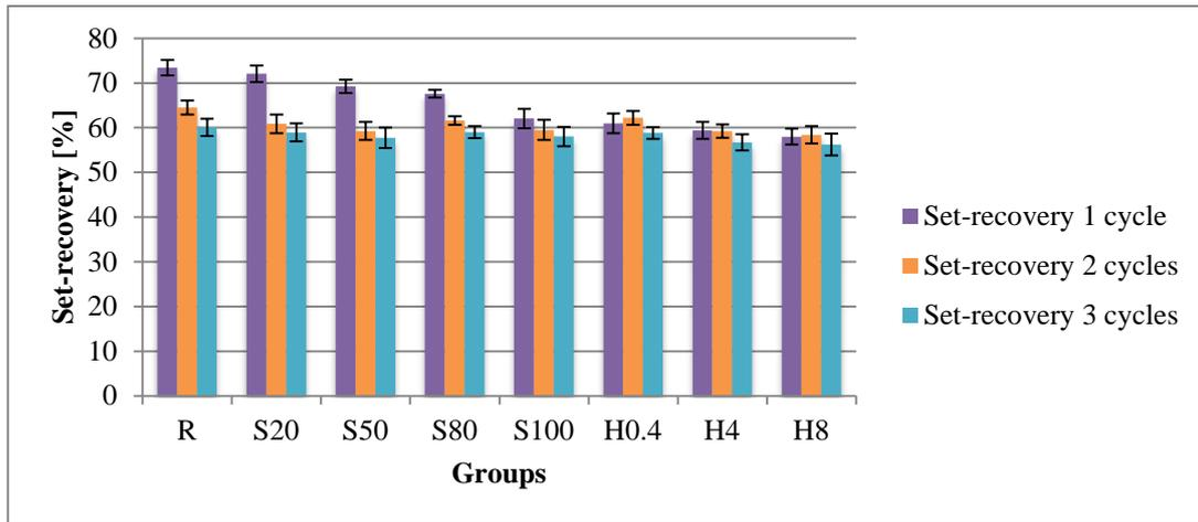
Figure 1: Set-recovery of all groups after one, two and three wet-dry cycles. The colored bars show the average of the 15 specimens in each group. The error bars show the standard deviation.
