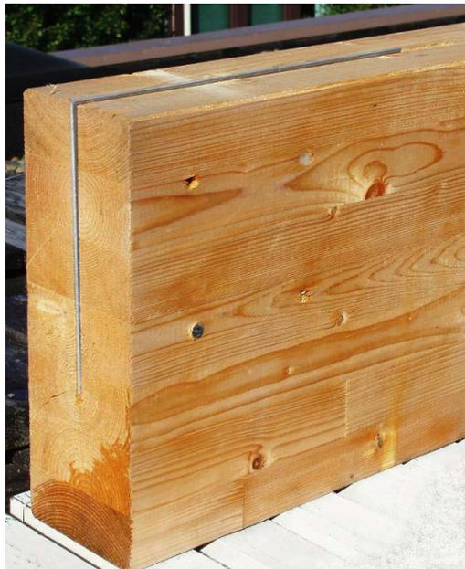
**Figure 1: Glulam beam with the connector parts replaced by aluminium.**
