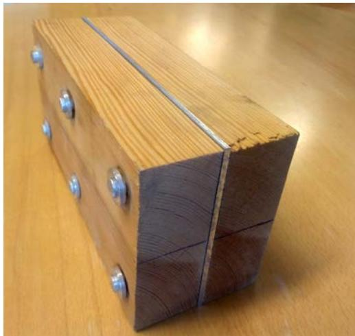
**Figure 2:** Two pieces of Scots pine attached to a 3 mm thick aluminium plate.
