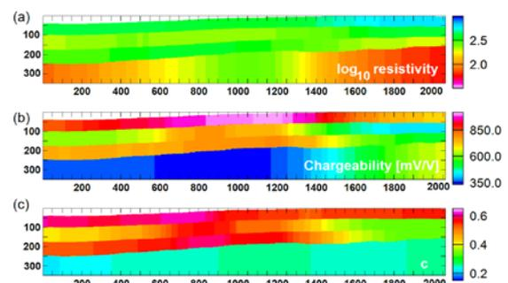
**Figure 5.** Model obtained from inversion of data from Line 104801 (data are shown in Figure 6)
