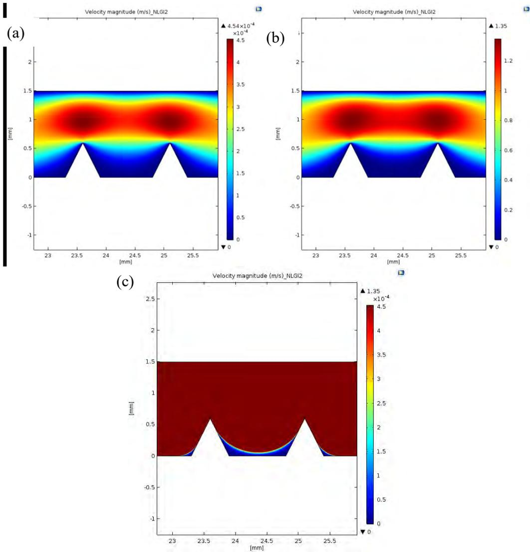
Figure 10: The average velocity field for the NLGI2 grease at (pressure drop): (a) 30 kPa, (b) 250 kPa, (c) 250 kPa with same range of colour bar as in (a).
