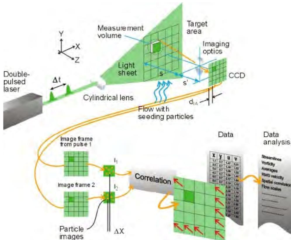
Figure 5: The principle of PIV. The correlation between images is made via Fast Fourier Transform (FFT) in the PIV software. The calculations does hence not track individual particles, but capture the statistical behaviour of all particles in the sub-frames (interrogation areas) of each image.
