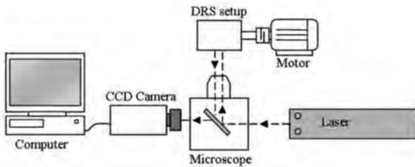
Figure 4: A typical  $\mu$ PIV setup with microscope, camera, test rig, motor/pump to drive the flow, laser, and computer.
