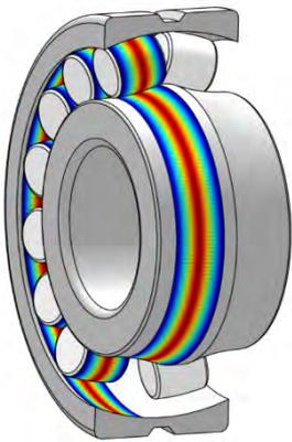
Figure 1: Oil layer distribution on a spherical roller bearing where the oil flow is induced by the tangential component of the centrifugal forces on inner ring and rollers (van Zoelen, 2010). Red colour indicates the thinnest lubricant film.
