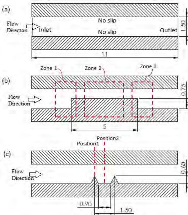
Figure 2: Progression of straight channels used in the CFD modelling for validation with flow visualizations: without restrictions (a - also used in the analytical
