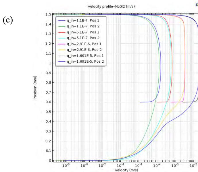
Figure 11: Velocity profile measured at position 1 and position 2 in Fig. 2c: (a) NLGI00 grease, (b) NLGI1 grease, (c) NLGI2 grease. The flow rate  $q$  is the flow across the channel height for each corresponding position.
