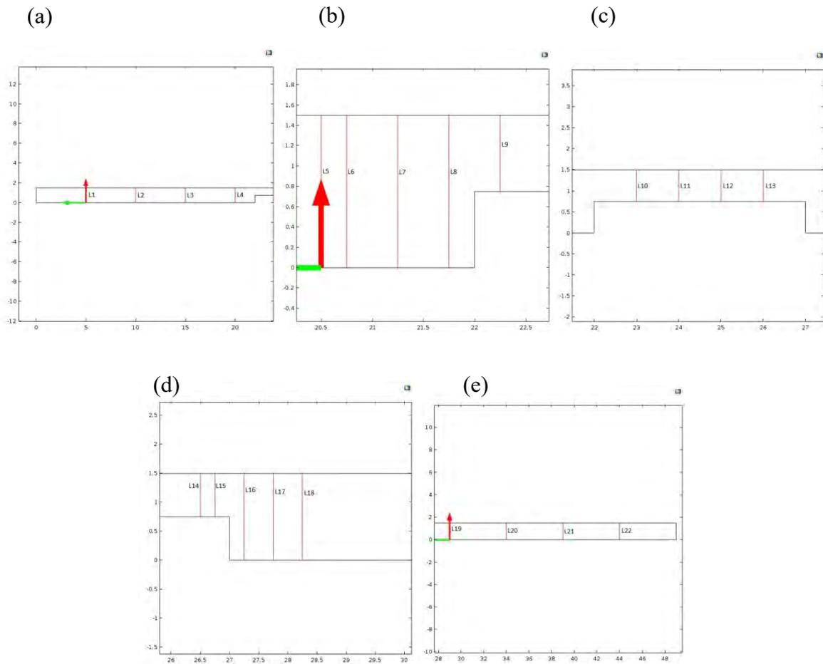
Figure 8: Sketches of cutline (a) L1, L2, L3, L4 along the inlet, (b) zone 1: L5, L6, L7, L8, L9 before the restriction, (c) zone 2: L10, L11, L12, L13 in the restriction, (d) zone 3: L14, L15, L16, L17, L18 after the restriction and (e) L19, L20, L21, L22 along the outlet
