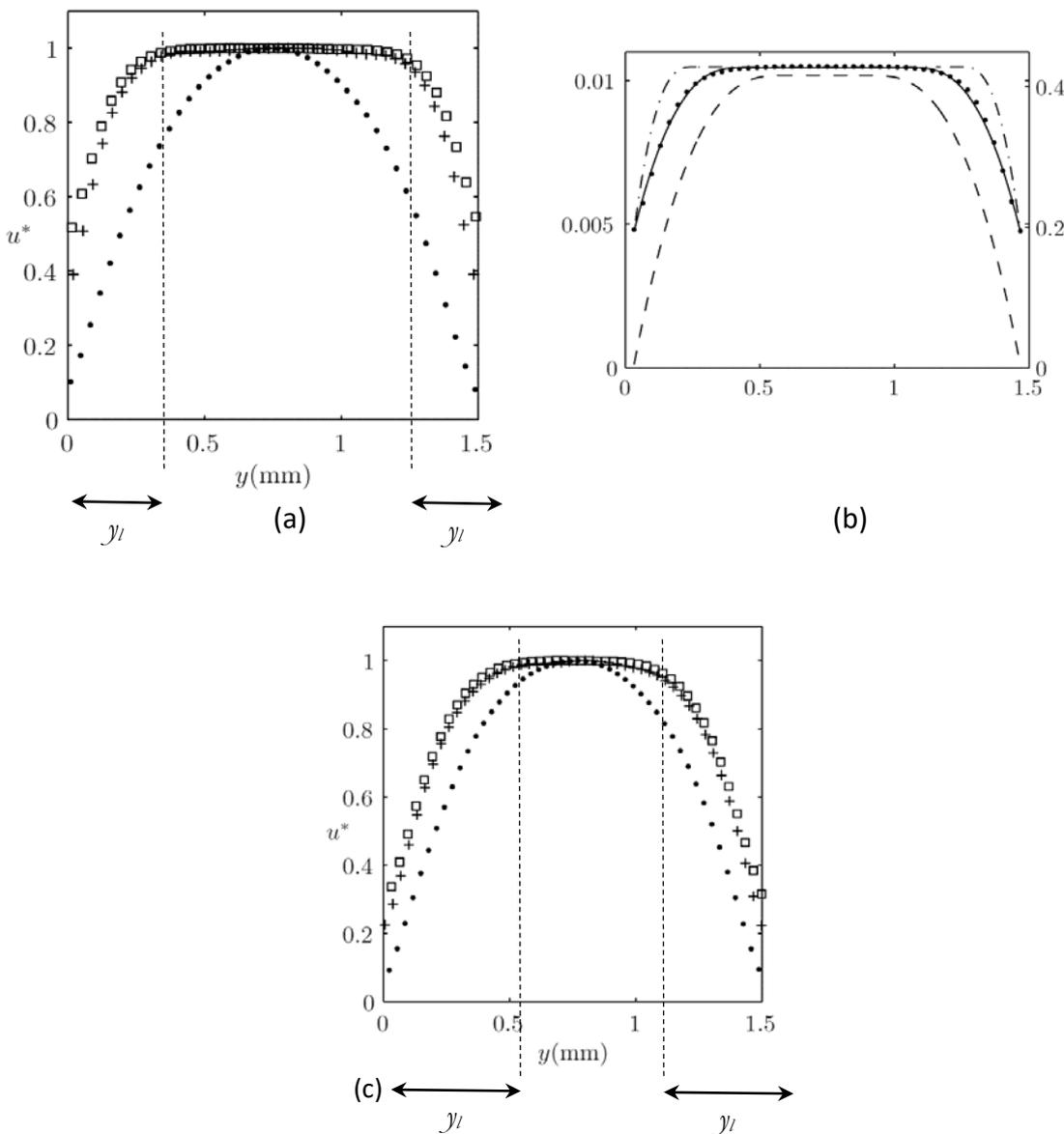
Figure 3: (a) Velocity profiles from flow visualizations across a straight channel without restrictions for three lithium greases with different thickness; see Tab. 1 for rheological data. The different labels represent different grease thickness such that □: NLGI 2, +: NLG I1, and •: NLGI 00.  $y_l$  denotes the distance to the yield point. (b) Velocity profiles across a straight channel of width 1.5 mm. The profiles show dimensionless quantities, scaled with the
