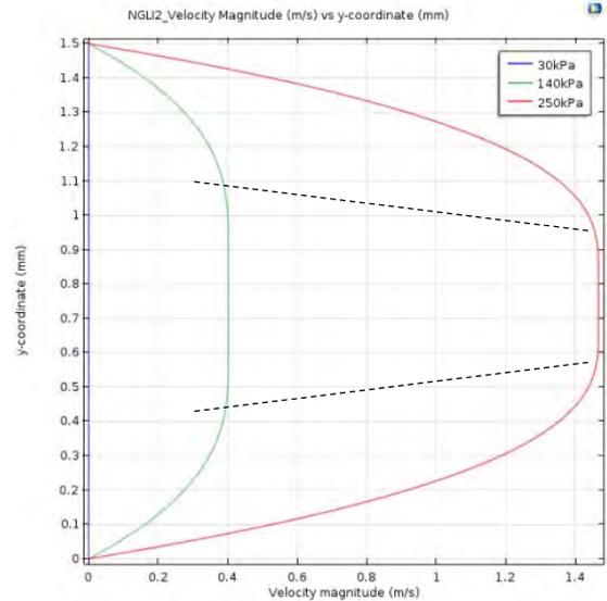
Figure 6: Velocity profiles (fully developed) of (a) NLGI00 (b) NLGI1 and (c) NLGI2 greases in the straight channel without restrictions. The pressures represent the pressure drop between inlet and outlet, and the dashed lines shows the evolution of the plug region with increasing pressure.
