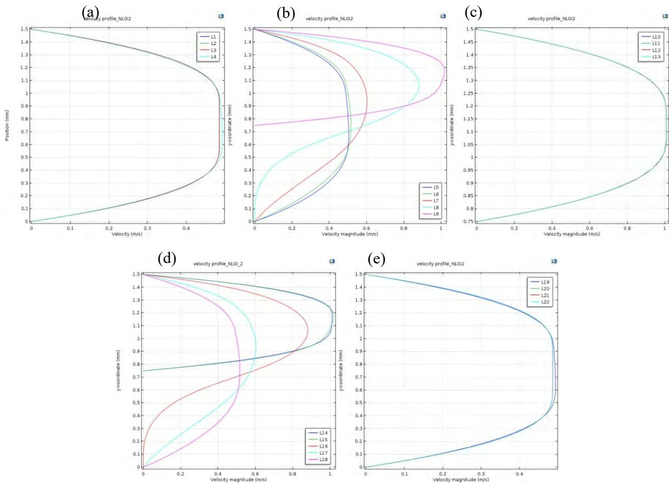
Figure 9: Velocity profiles of the NLGI2 grease at the position of the cut lines presented in Fig. 8. Each subfigure in this figure correspond to the same set of cut-lines as in corresponding subfigure in Fig. 8.
