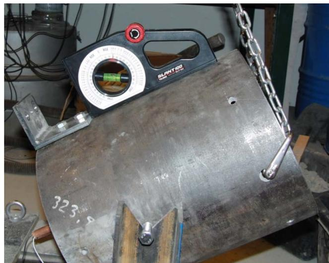
**Figure 13:** Angle of repose measurement
