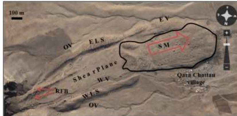
Fig.9: Flash Earth image facing south showing the slid mass (SM), the Eastern longitudinal strip (ELS), Western Longitudinal Strip (WLS), eastern valley (EV), western valley (WV), recently fallen blocks (RFB). Note the concentration of the large blocks on the top of the slid mass.
