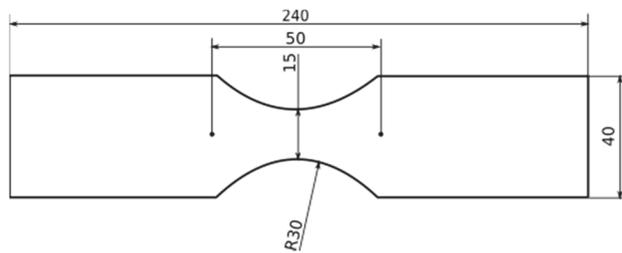
**Figure 1:** Notched tensile specimen; Sheet thickness: 1.2mm; Gauge length: 50mm
