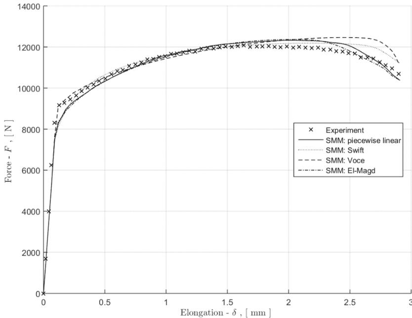
**Figure 3:** Comparison of the force-elongation relations from the experiment with FEM simulations based on SMM material-models
