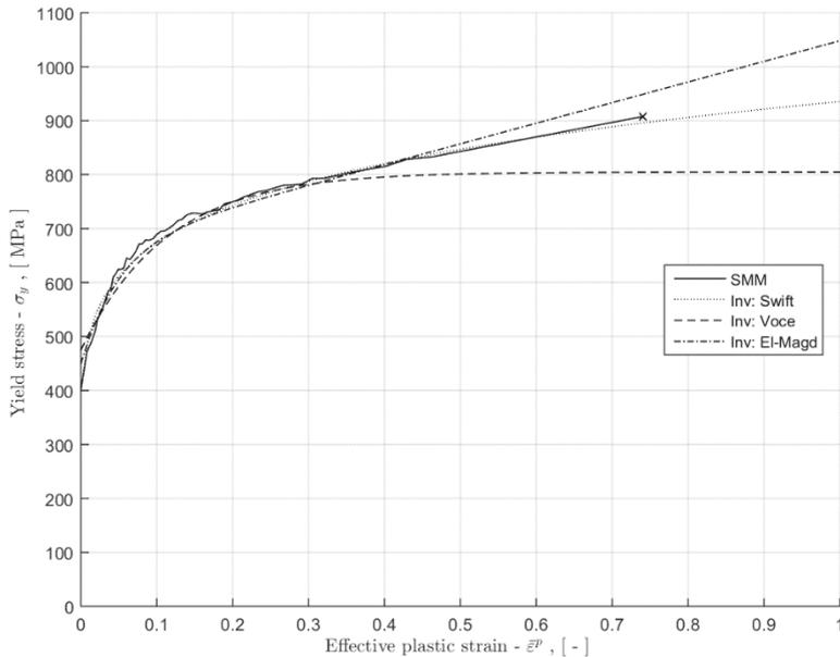
**Figure 2:** Resulting stress-strain relation from SMM and Inverse modelling
