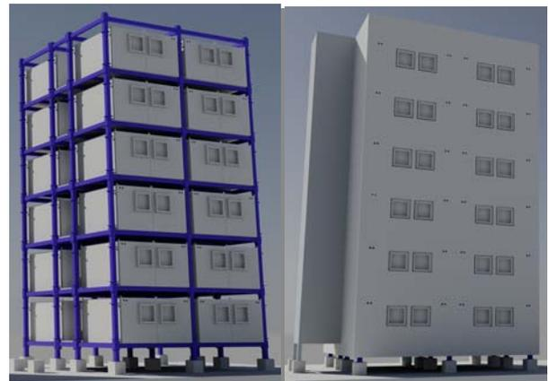
Figure 4. Conceptual view neglecting façade (left side) and with façade (right side) [4]
