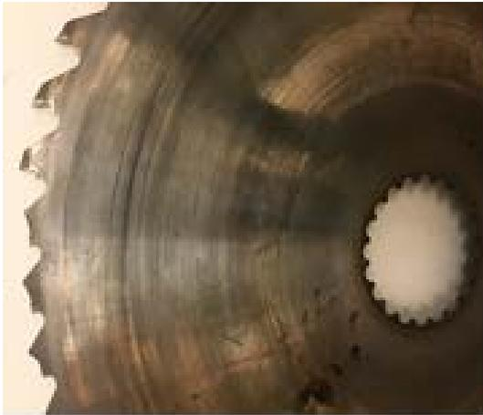
**Figure 1:** Teeth damage due to overload
