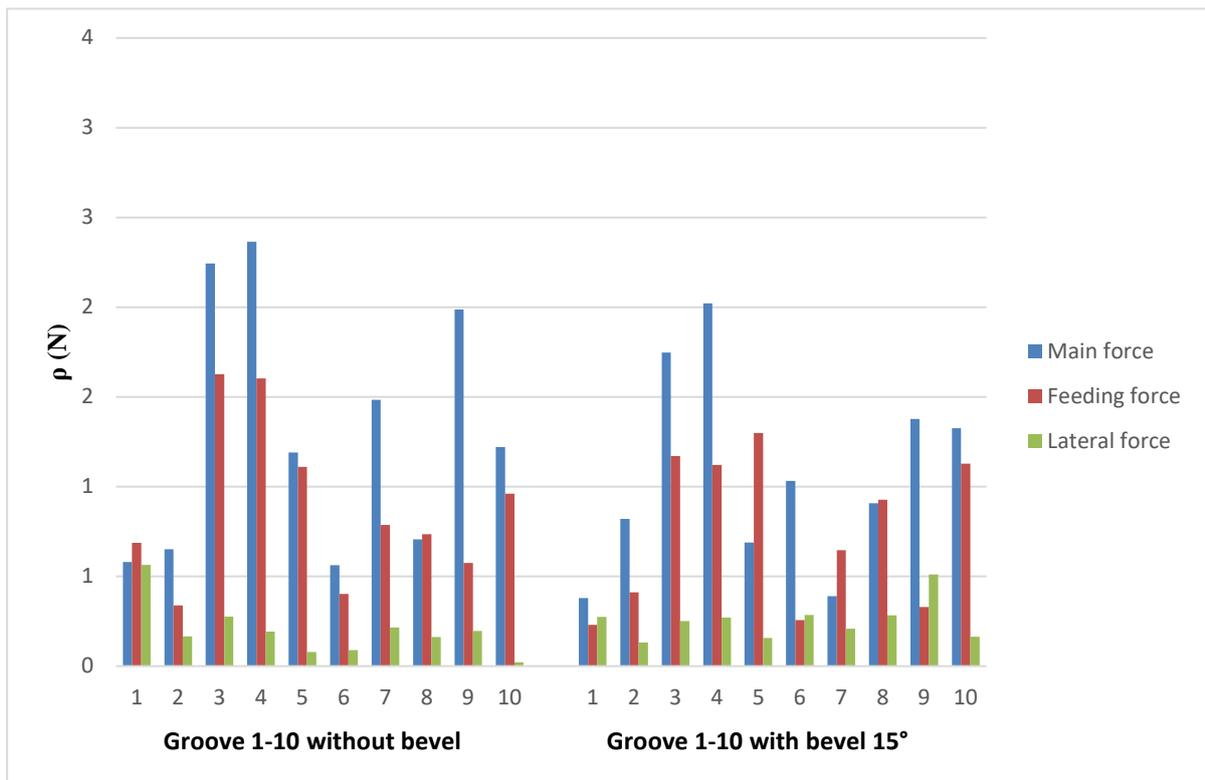
**Figure 13:** Standard deviation values ( $\rho$ ) for sample B (at room temperature)
