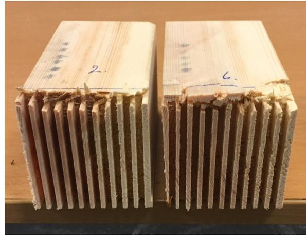
**Figure 4:** Two samples of Scots pine with grooves cut by the cutting tool shown in Fig.3
