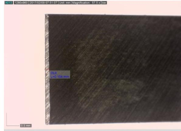
**Figure 6:** Cutting edge (left side) made of a hard-metal material DH10 with a bevel width of 0.15 mm. View towards rake face
