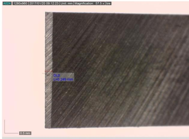
**Figure 2:** Cutting edge with a bevel (left side). View towards rake face. Rake angle  $30^\circ$ , bevel rake angle  $15^\circ$ , bevel width 0.25 mm, cutting width 4.2 mm
