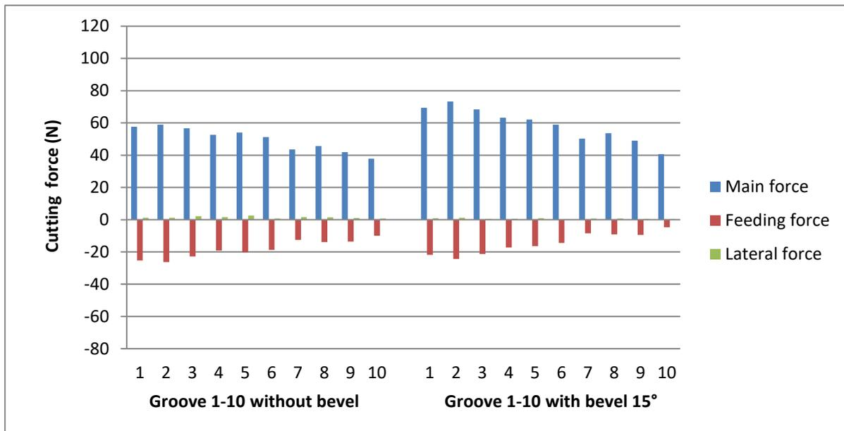
**Figure 11:** Cutting forces for sample B (in room temperature condition)
