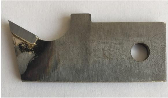
**Figure 3:** Cutting tool with a tooth made of hard-metal material
