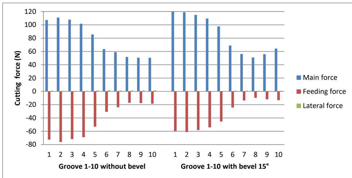
**Figure 10:** Cutting forces for sample A (in frozen condition)
