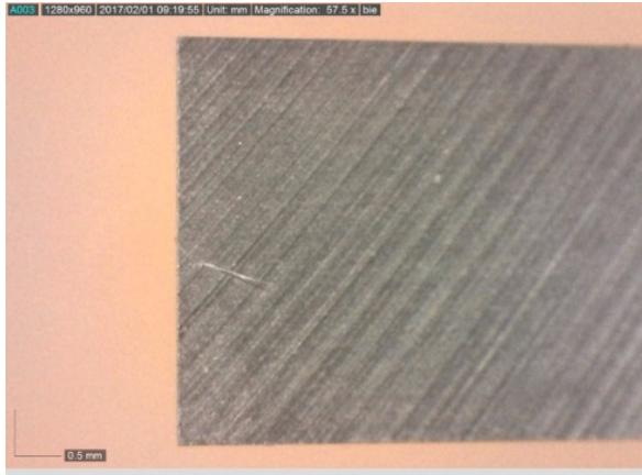
**Figure 5:** Cutting edge (left side) made of hard metal material DH10 without bevel. View towards rake face
