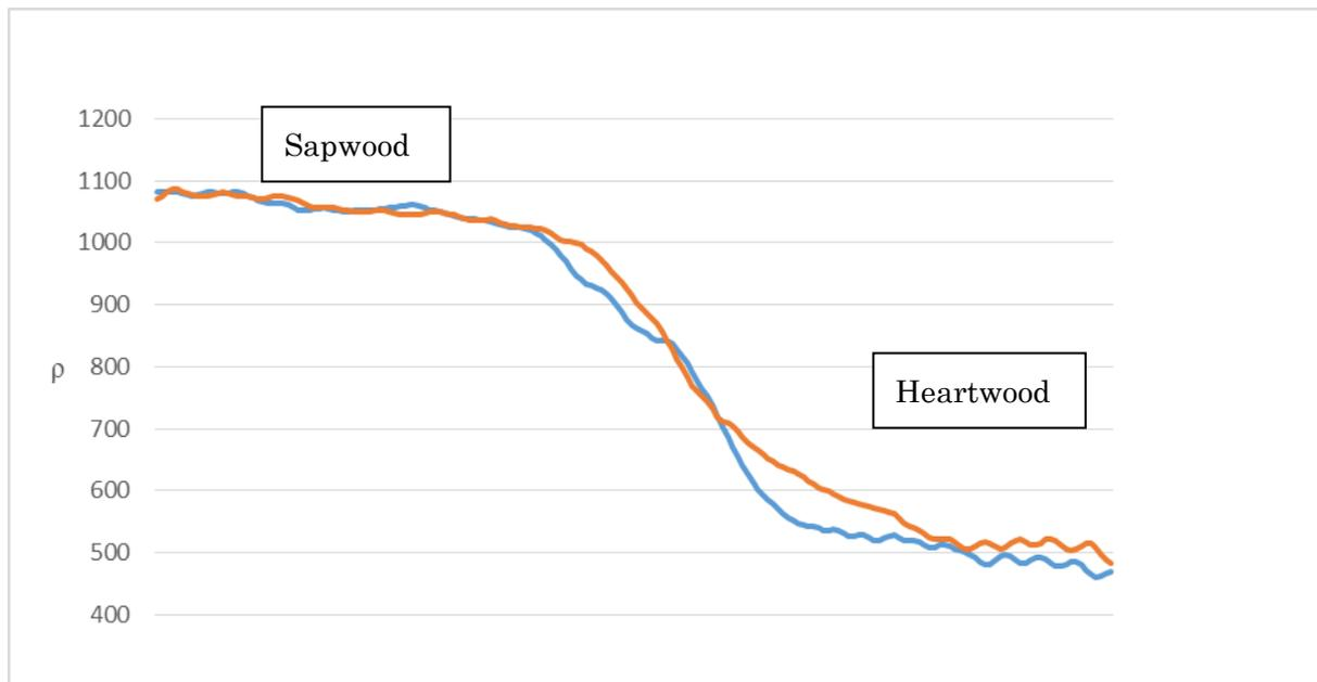
Figure 9: Mean density  $\rho$  (kg/m<sup>3</sup>) in width direction of sample A (blue) and sample B (red).
