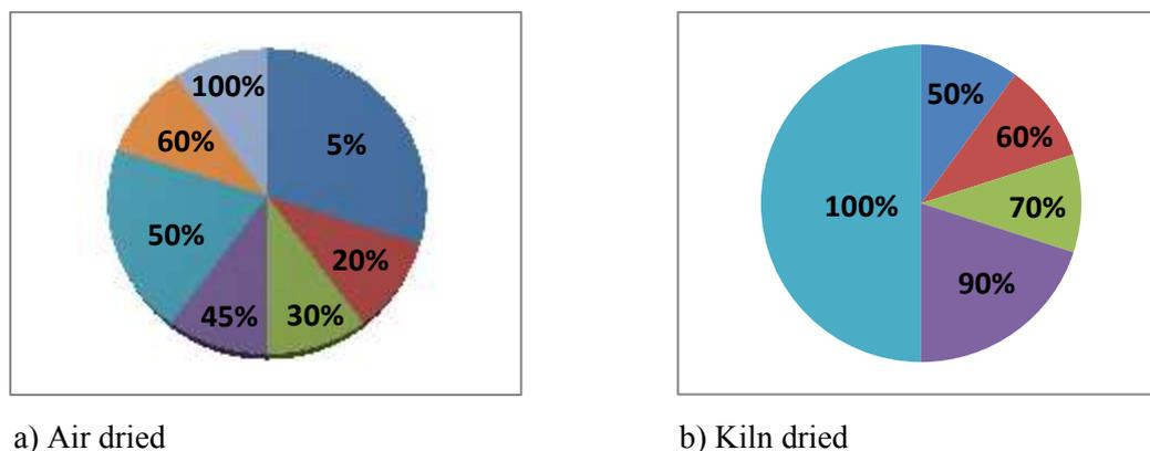
Figure 2: Variability of the area coverage of mould (%) on sapwood of pine boards dried in (a) air or in (b) an industrial kiln
