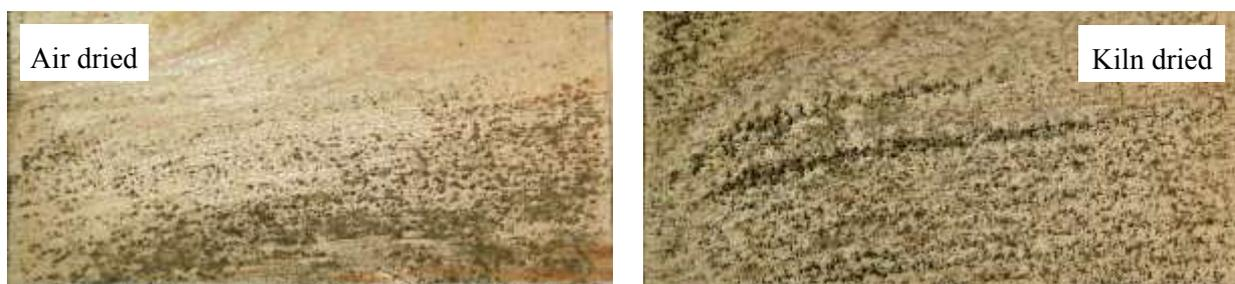
Figure 1: Surface view of air and kiln dried Scots pine sapwood boards after mold test
