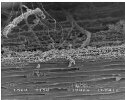
Figure 3: Scanning electron micrograph of mould growth on a kiln-dried wood surface
