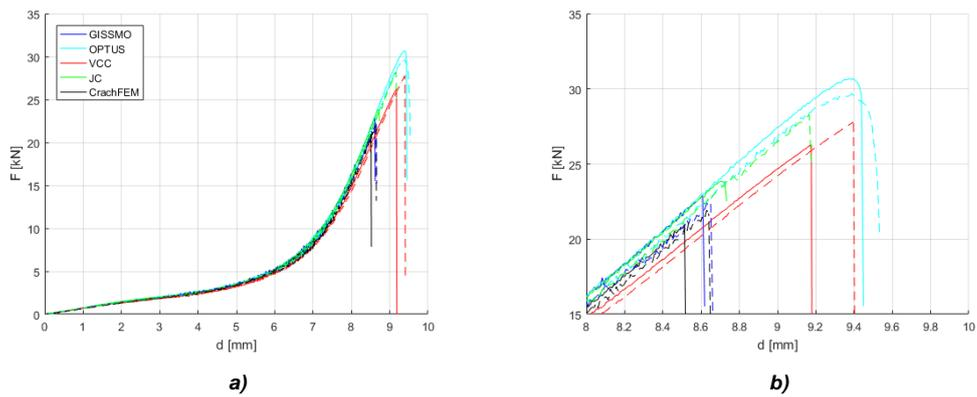
**Figure 5:** Load-displacement response of the virtual test component compared for five models.
