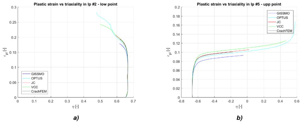
**Figure 3:** Stress triaxiality in the lower and upper point of the element in the critical cross-section.
