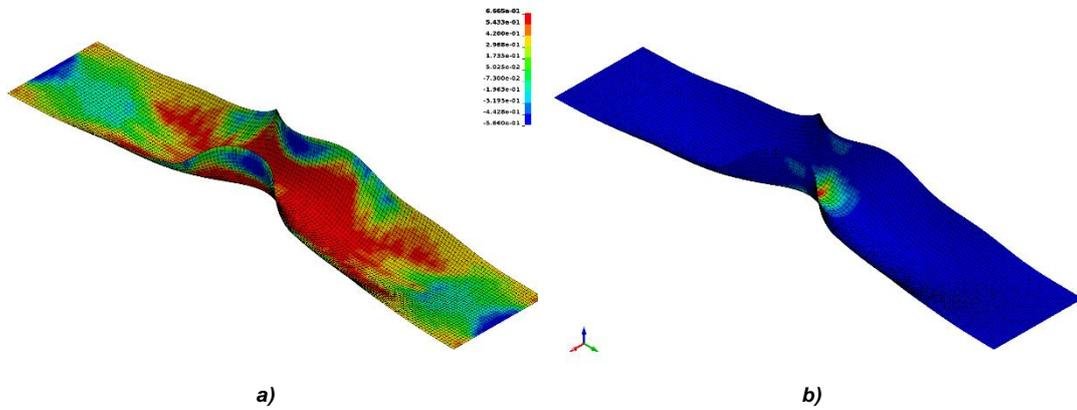
**Figure 4:** Fringe plot of a) stress triaxiality, and b) plastic strain.
