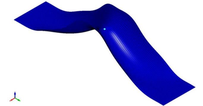
**Figure 2:** Geometry of the virtual test component used for the finite element model. Marked in light blue the element used for data extraction.
