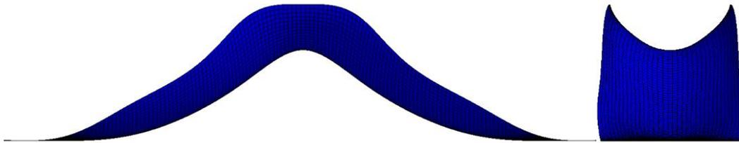
**Figure 1:** Front and side view of the virtual test component. In the view to the left, right end has a boundary condition prohibiting displacement in longitudinal direction of the component, left end with prescribed velocity. Deformation of the component in vertical direction.
