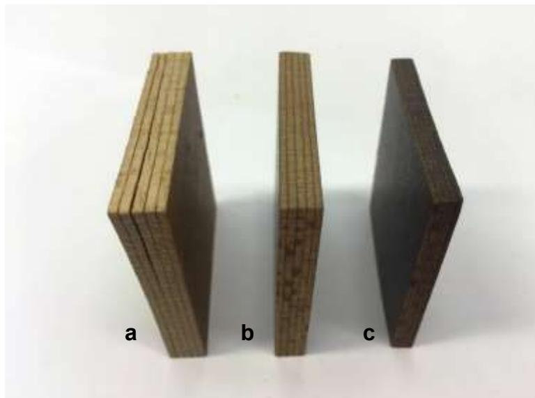
Figure 3: Samples after an adsorption-desorption cycle from 30 to 90% RH. Boards pressed at a) 200°C, 5 MPa, 300 s, b) 225°C, 5 MPa, 300 s, and c) 250°C, 5 MPa, 300 s.
