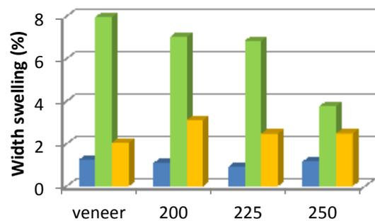
Figure 6: Width swelling of veneers and boards pressed at 200, 225 and 250°C during an adsorption-desorption cycle at 23°C.
