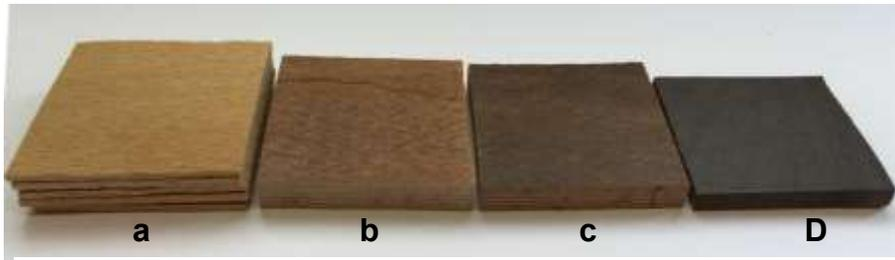
Figure 1: Veneers and boards pressed at different pressing conditions: a) the veneers before pressing, and after pressing at b) 200°C, 5 MPa , 300 s, c) 225°C, 5 MPa , 300 s, and d) 250°C, 5 MPa, 300 s.
