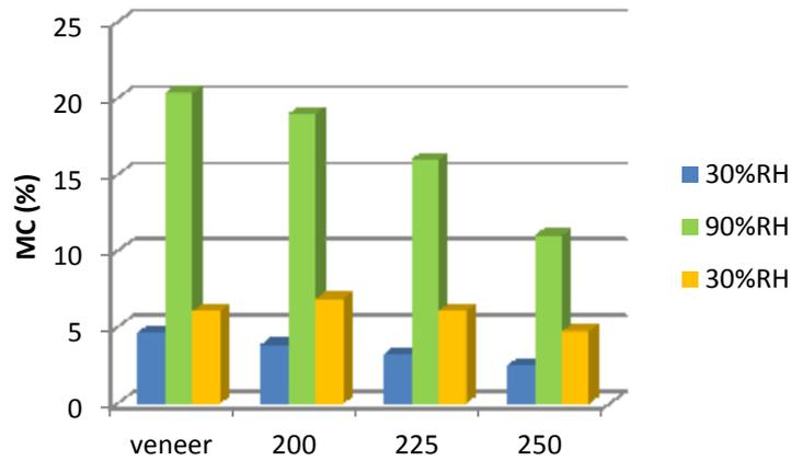
Figure 4: MC of veneers and boards pressed at 200, 225 and 250°C during an adsorption-desorption cycle at 23°C.
