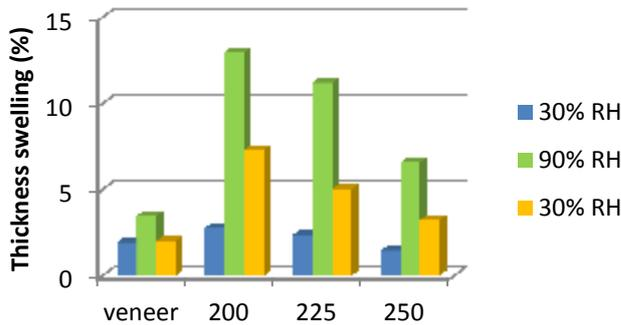
Figure 5: Swelling in thickness of veneers and boards pressed at 200, 225 and 250°C during an adsorption-desorption cycle at 23°C.
