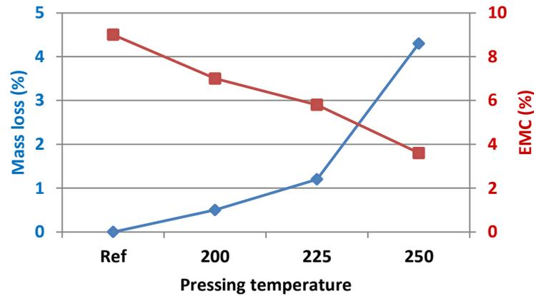
Figure 2: Mass loss and EMC of self-bonded boards.
