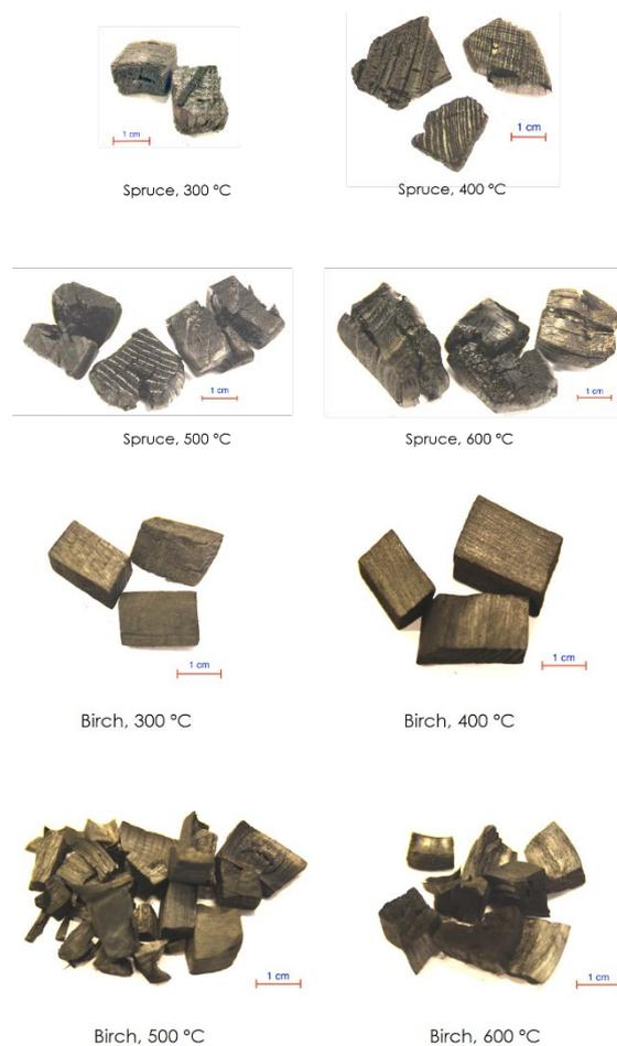
**Figure 4:** Visual appearance of char produced from pyrolysis at different temperature
