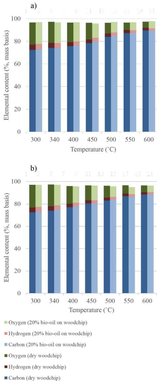
**Figure 5:** Mass content of C, H, and O in biochar samples (a) spruce (b) birch
