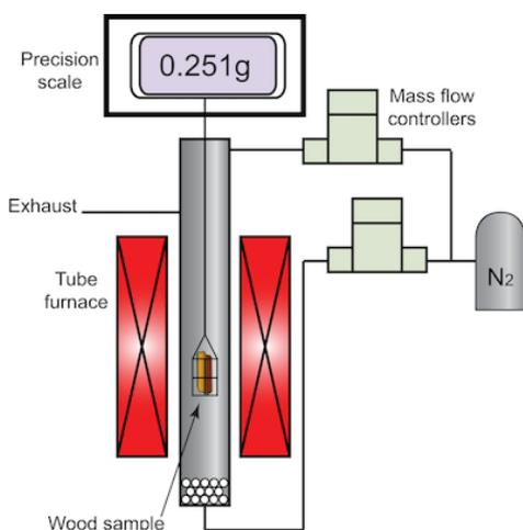
**Figure 1:** Macro-Thermogravimetric experiment
