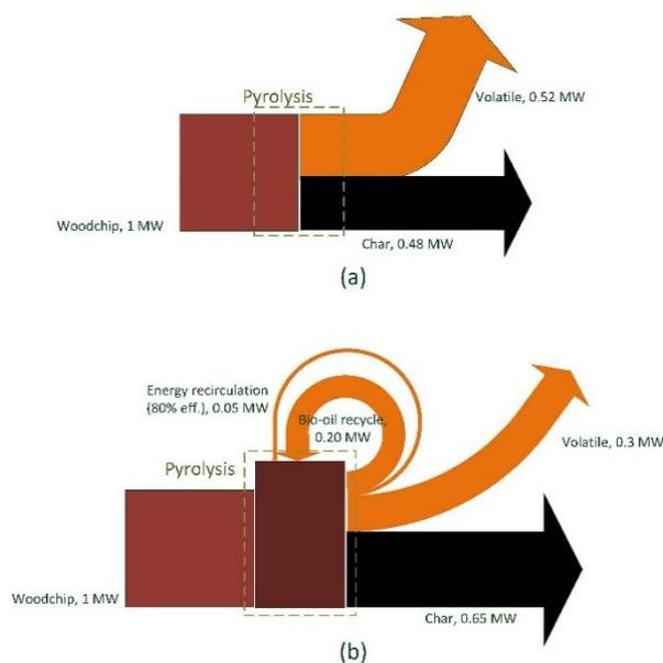
**Figure 8:** Energy balance (a) pyrolysis without bio-oil recycle at 340 °C (b) pyrolysis with 25% (m/m) bio-oil recycle at 340 °C
