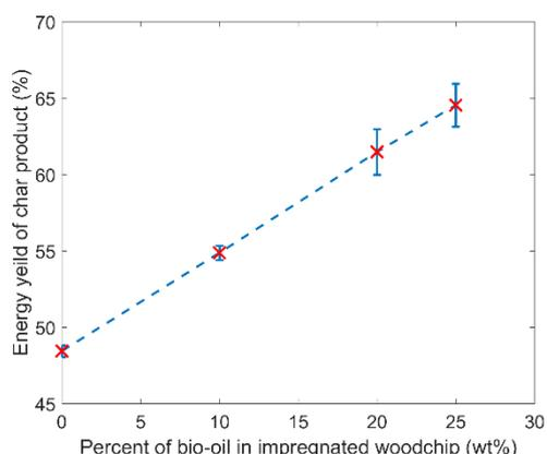
**Figure 7:** Energy yield of char produced at 340 °C with variety of bio-oil ratio
