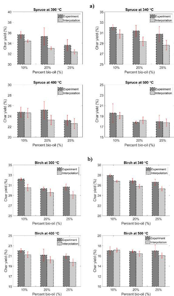
**Figure 3:** Comparison of char yields (mass basis) from isothermal pyrolysis of impregnated woodchip with different bio-oil ratio (a) spruce (b) birch
