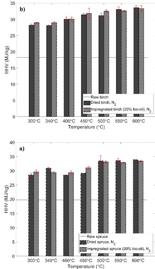
**Figure 6:** HHV results of char from pyrolysis at different temperature (a) spruce (b) birch
