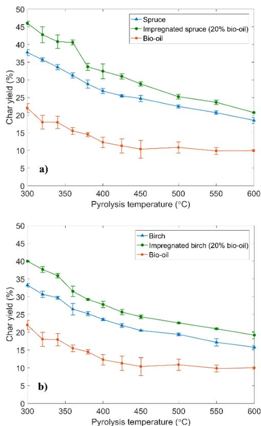
**Figure 2:** Char yield (mass basis) from isothermal pyrolysis at various temperature (a) spruce (b) birch
