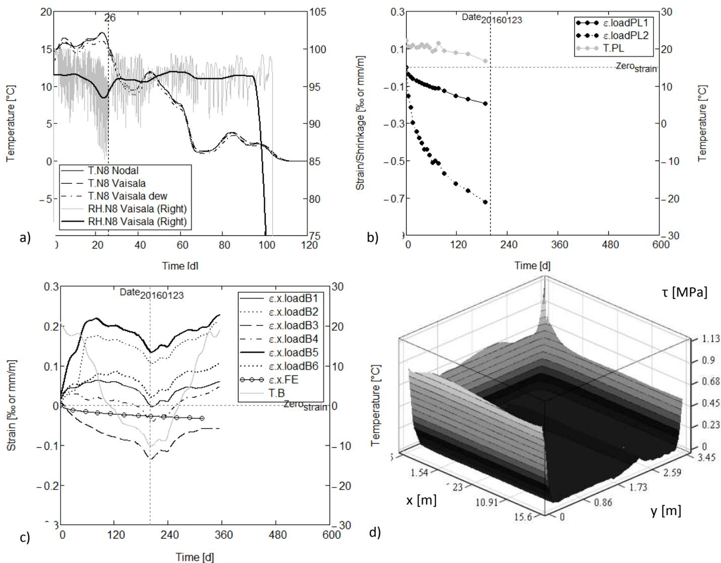
Fig 3.a) Climate data (first 118 d) b) Example of shrinkage - indoor specimens c) example longitudinal overlay strain (first 300 d) d) FEM interface shear stress [MPa,] outer 1/4 part
