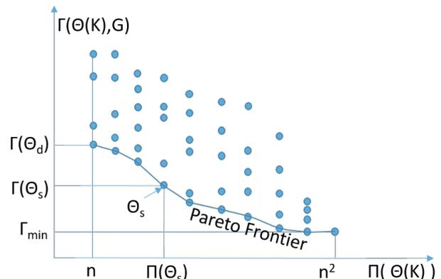
Fig. 5. Illustration of the Control Configuration Selection problem as an optimization scheme.
