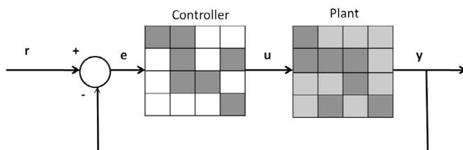
Fig. 4. Sparse control configuration.
