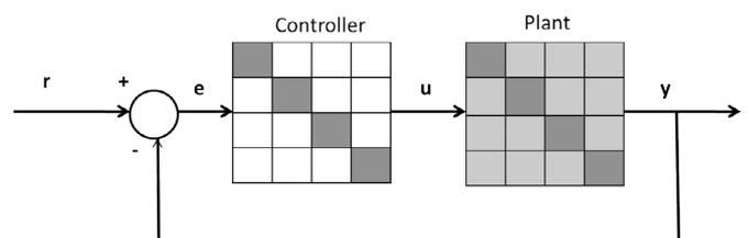
Fig. 2. Fully decentralized control configuration. The shaded elements in the controller matrix represent SISO controllers. The considered input-output channels in the reduced model of the plant are represented in dark gray.
