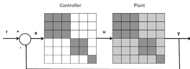
Fig. 3. Block diagonal control structure. In this case, the process is assumed to be composed by three segregated subsystems which are independently controlled by each of the blocks in the controller.
