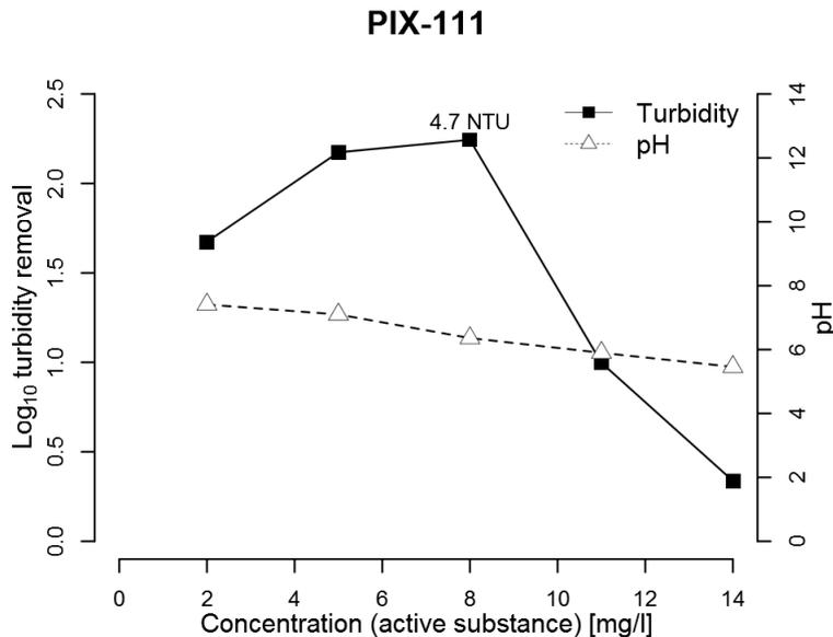
**Fig. 2.** Turbidity log-removal and pH in the snow melt mixture after C/F using PIX-111, an iron chloride coagulant. The residual turbidity for the concentration that yielded the highest turbidity removal is indicated.
