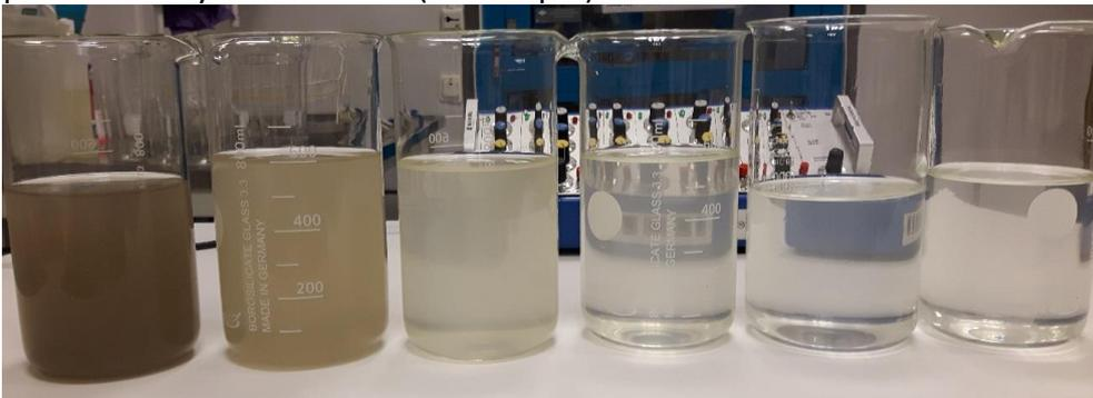
**Fig. 1.** Left-most beaker contains untreated urban snow melt mixture. The following beakers have been treated with an increasing concentration of PAX-215.
