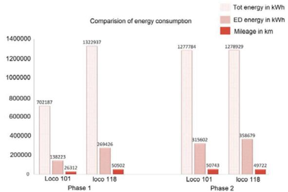
Figure 5. Comparison of energy consumption, regenerative energy and mileage between the re-profiling of locomotives no.101 & 118 during the period of 2014-12-10 to 2015-12-10.
