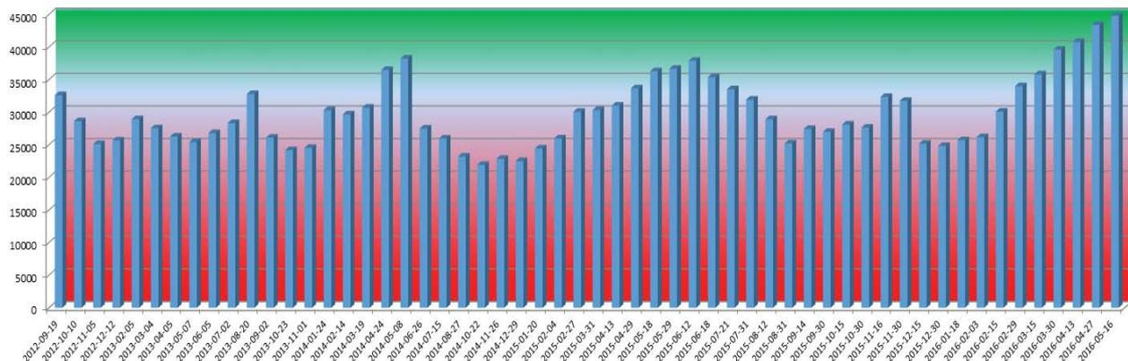
Figure 2. Estimated lifetime locomotive wheels based on turning interval rolling 12 months, September 2012 to May 2016.
