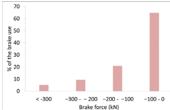
Figure 3. ED-brake force distribution for IORE locomotives.
