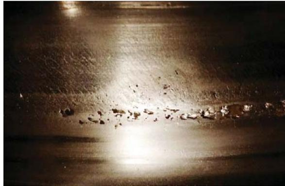
Figure 4. RCF class 3, IORE locomotive no. 101.
