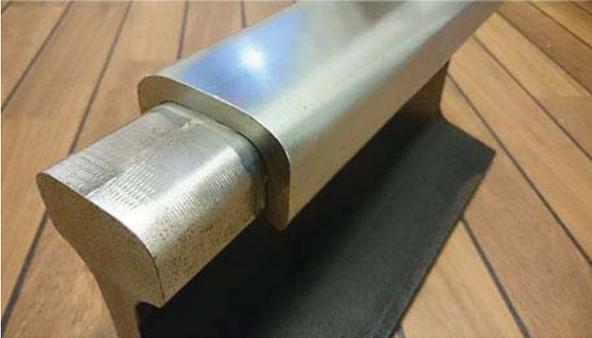
Figure 12. ReRail is a replaceable rail head.
