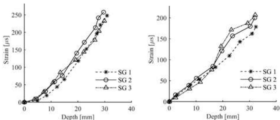
Figure 3. Measured development of strains as function of saw-cut depth for non-destructive determination of the residual prestress force in the south girder, Left: Section A close to midspan 1. Right: Section D at midspan 3. Bagge (2017) [6].
