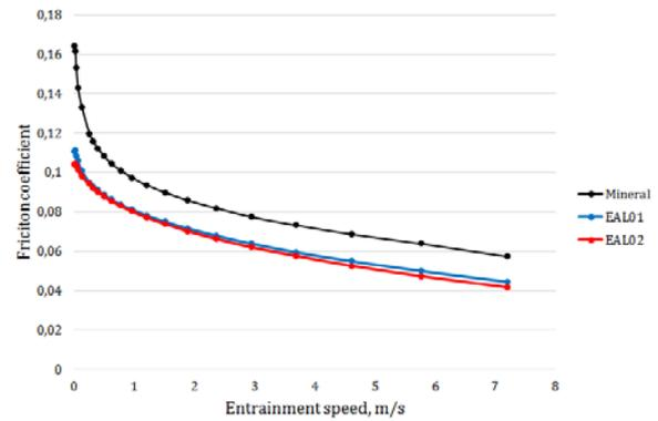
**Fig. 5 Rolling/sliding friction vs entrainment speed**
