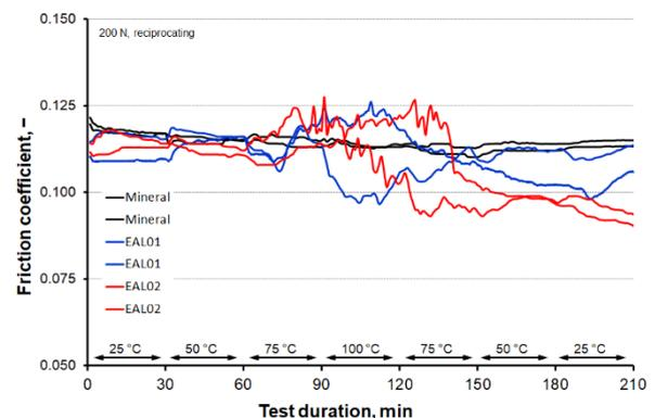
Fig. 3 Friction in temperature-programmed test
