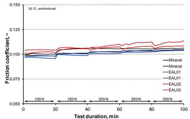
Fig. 1 Friction in unidirectional motion
