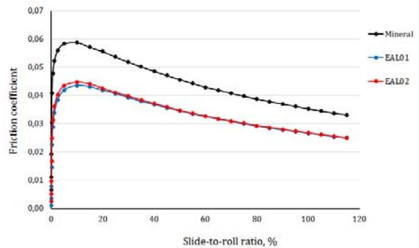
**Fig. 6 Rolling/sliding friction vs slide-to-roll ratio**
