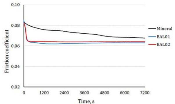
**Fig.7 Friction vs time in rolling/sliding wear test**
