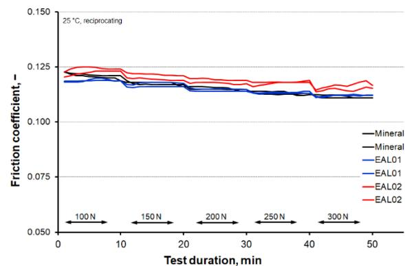
Fig. 2 Friction in reciprocating motion
