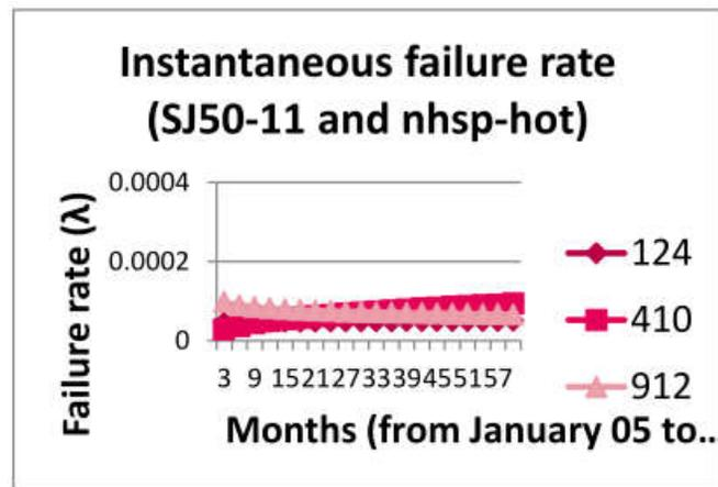
Figure 10: Failure rate of turnout SJ50-11 in different tracks in hot season
