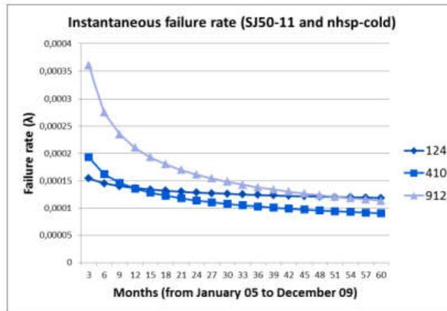
Figure 9: Failure rate of turnout SJ50-11 in different tracks in cold season
