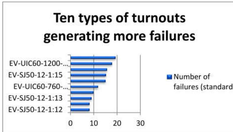
Figure 3: Bar chart of ten types of turnouts generating more failures
