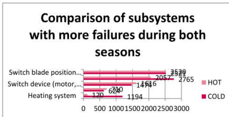
Figure 7: Comparison of subsystems with more failures during both seasons
