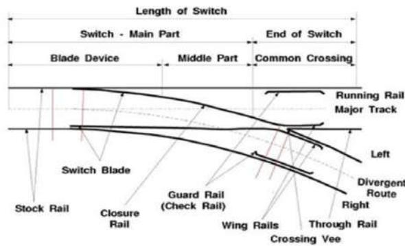
**Figure 1:** Schematic of a switch and crossing
