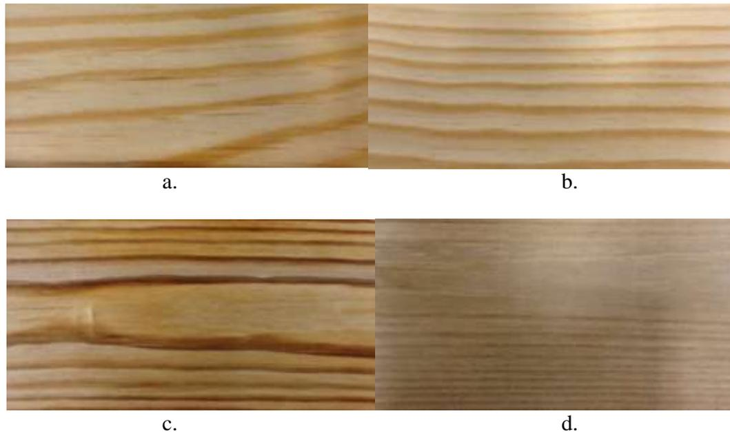
Figure 3: Accelerated weathering of sapwood of pine (PS) and thermally modified timber (TMT) treated with methacrylic resin (MA): a) PS, b) PS+MA, c) TMT, d) TMT+MA.
