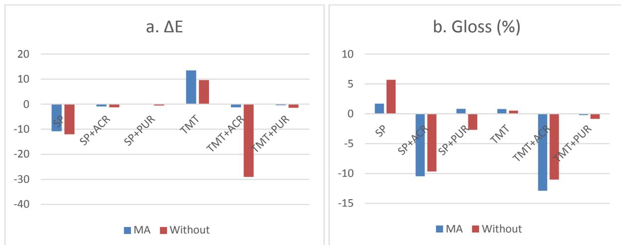
Figure 2: Change in a) colour ( $\Delta E$ ) and b) gloss ( $65^\circ$ ) during accelerated weathering.
