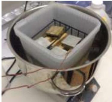
Figure 1: Hot and cold batch of methacrylate and samples of wood.
