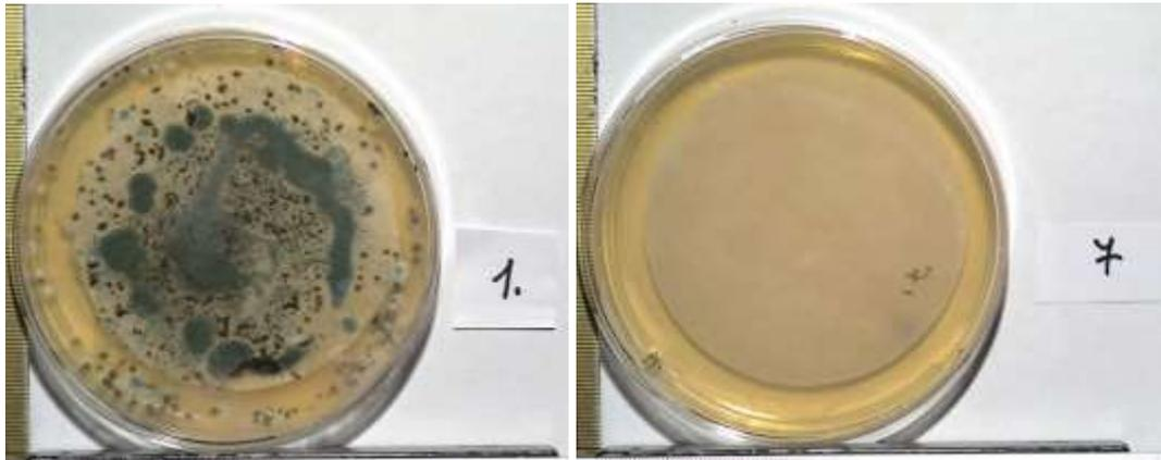
Fig. 4. Filter paper treated without (1) and with methacrylic resin (7) after mould test.
