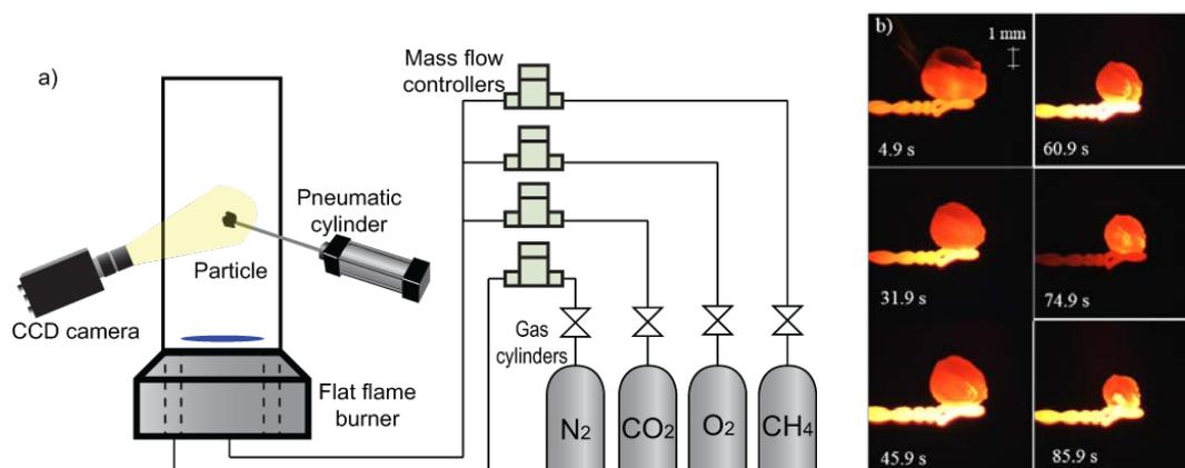
**Figure 1.** Experimental method a) Schematic diagram of the gasification experiment in FFB
