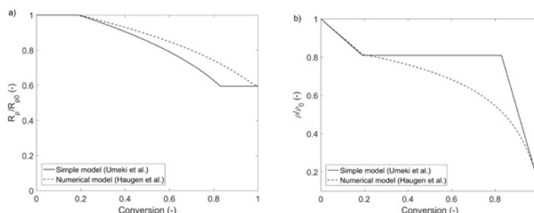
**Figure 2.** Comparison of the models for a) particle radius and b) apparent density. The model was calculated for the initial particle diameter of 30  $\mu\text{m}$  and the reaction temperature of 1300 K.
